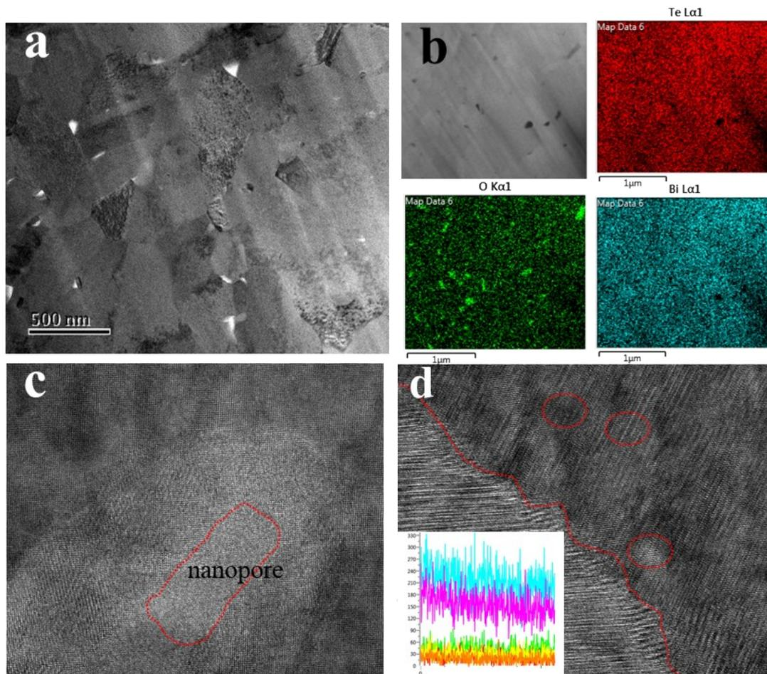
**Fig. S2.** The microstructure of the as-prepared M-BTZ sample. (a) low magnification TEM image. (b) TEM image and corresponding EDS elemental maps. TEM images of (c) the nanopores and (d) sawtooth grain boundaries.
