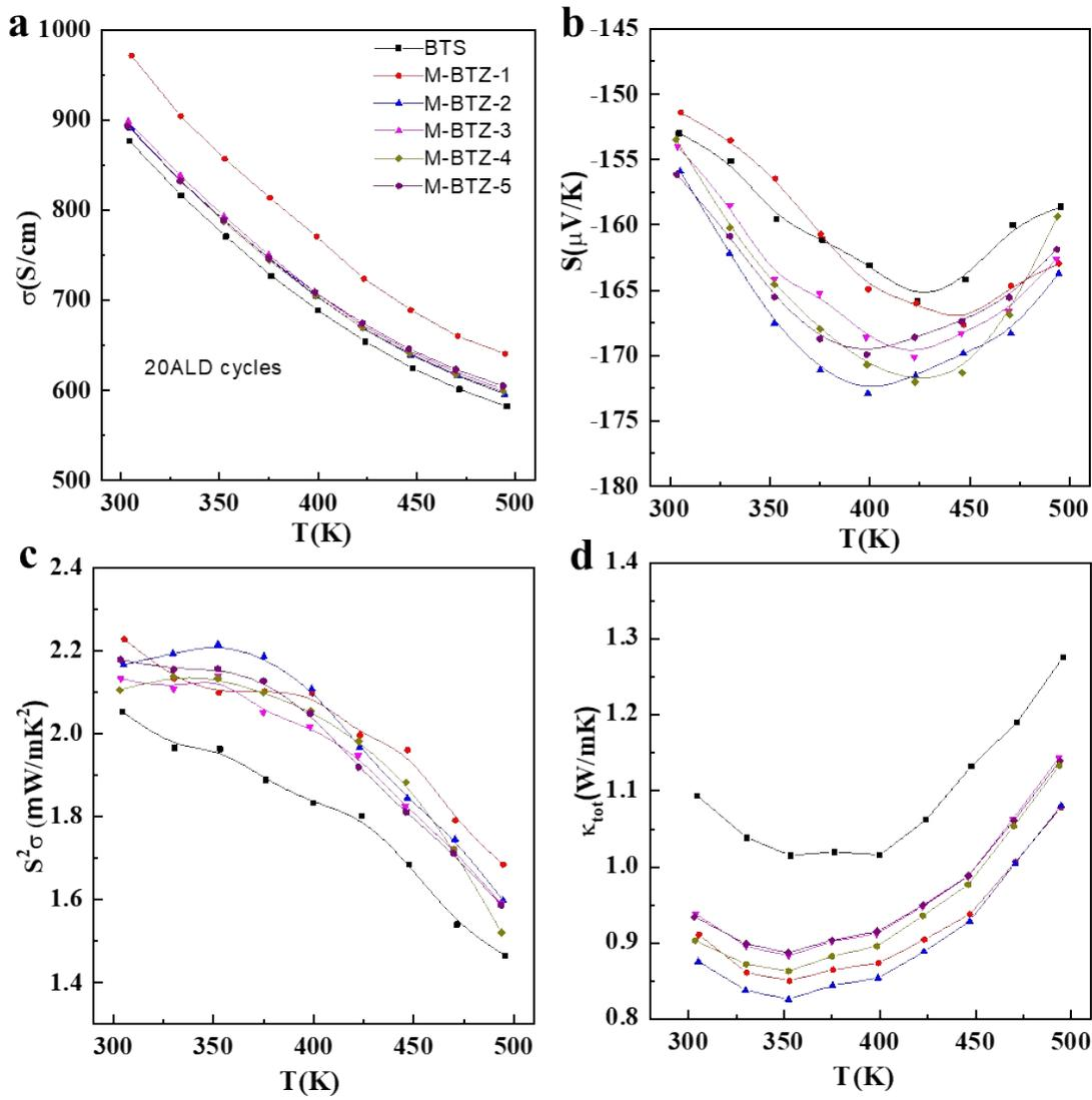
**Fig. S7.** The thermoelectric transport properties of the M-BTZ samples. (a) Electrical conductivity ( $\sigma$ ), (b) Seebeck coefficient (S), (c) power factor ( $S^2\sigma$ ). (d) Total thermal conductivity ( $\kappa_{\text{tot}}$ ).
