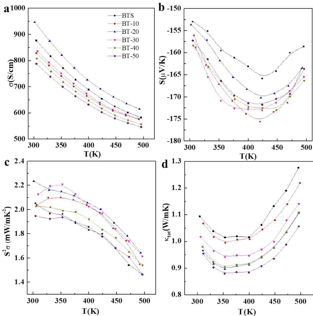
**Fig. S5.** The thermoelectric transport properties of the BT samples with different ALD cycles. (a) Electrical conductivity ( $\sigma$ ), (b) Seebeck coefficient ( $S$ ), (c) power factor ( $S^2\sigma$ ). (d) Total thermal conductivity ( $\kappa_{\text{tot}}$ ).
