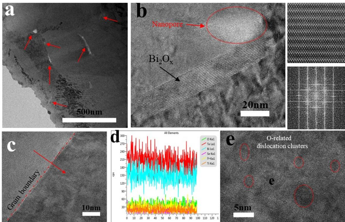
**Fig. S1.** The microstructure of the as-prepared BTZ sample. (a) low magnification TEM image. (b) the widespread nanopores and  $\text{Bi}_2\text{O}_x$  nanoprecipitates at the grain boundaries. (c) the TEM image (c) and corresponding EDS line-scan profiles. (e) the HRTEM image of the O-related dislocation cluster.
