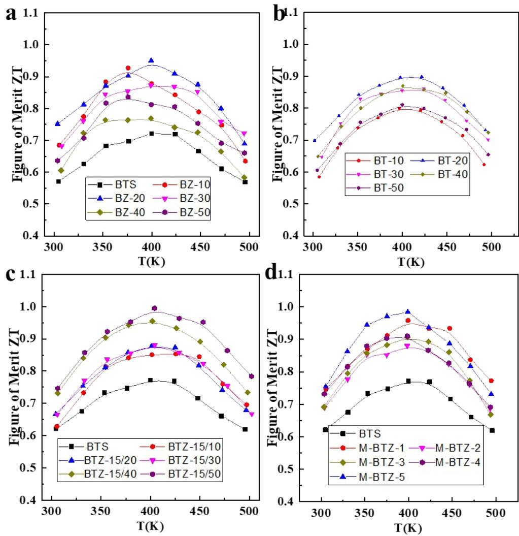
**Fig. S8.** Thermoelectric figure of merit  $ZT$  of the as-prepared sample. (a) BZ samples. (b) BT samples. (c) BTZ samples. (d) M-BTZ samples.
