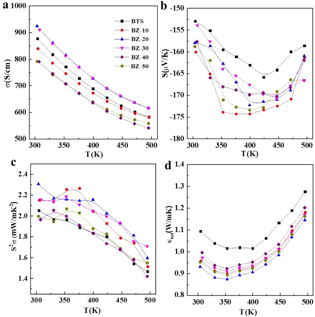
**Fig. S4.** The thermoelectric transport properties of the BZ samples with different ALD cycles. (a) Electrical conductivity ( $\sigma$ ), (b) Seebeck coefficient ( $S$ ), (c) power factor ( $S^2\sigma$ ). (d) Total thermal conductivity ( $\kappa_{\text{tot}}$ ).
