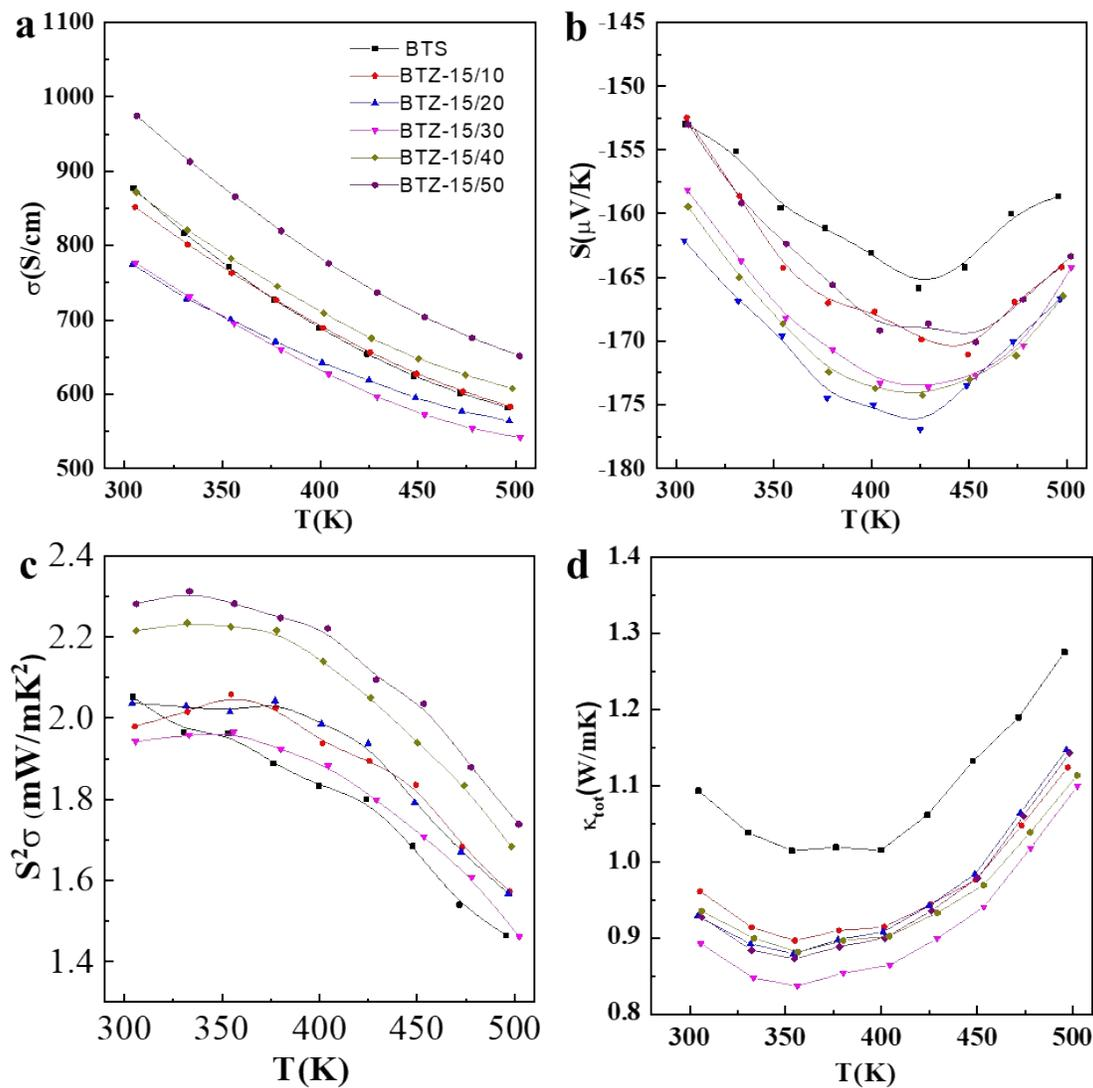
**Fig. S6.** The thermoelectric transport properties of the BTZ samples with different ALD cycles. (a) Electrical conductivity ( $\sigma$ ), (b) Seebeck coefficient (S), (c) power factor ( $S^2\sigma$ ). (d) Total thermal conductivity ( $\kappa_{\text{tot}}$ ).
