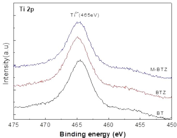
**Fig. S3.** XPS spectra for the as-prepared ALD coated BTS sample. (c) Ti 2p peaks of BT, BTZ and M-BTZ sample.
