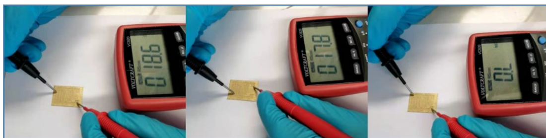
Fig. S17 Resistance testing of the device before active materials painting
