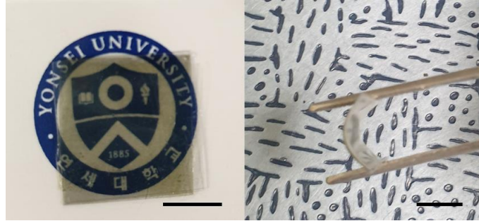
Fig. S3. Photographs of the fabricated MoS 2 -based TENG Scale bar is 5 mm.
