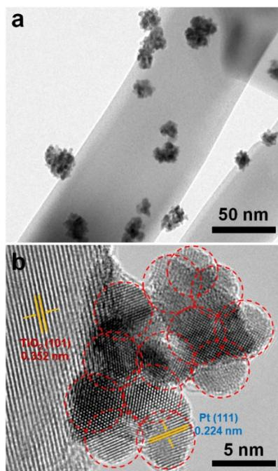
**Figure S1.** TEM (a) and HRTEM (b) images of Pt-NPs/TiO<sub>2</sub>. By using NaBH<sub>4</sub> in aqueous solution to reduce Pt precursor, the obtained reduced Pt tends to aggregate to large nanoparticles. The large particles are composed of primary particles with a diameter of about 3.9 nm.
