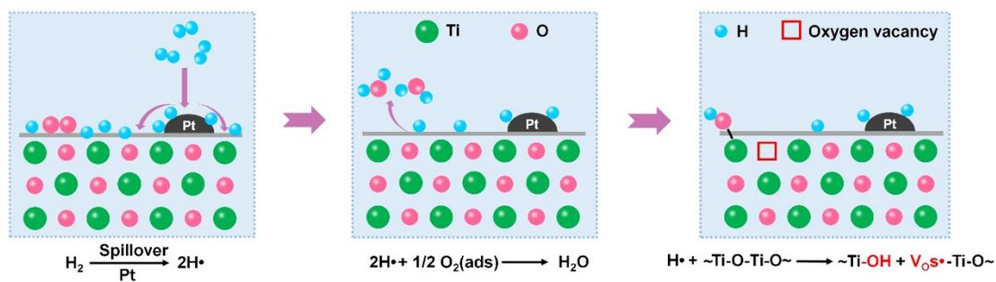
**Figure S5.** Schematic illustration of the formation of Ti-OH and oxygen vacancy with the assistance of hydrogen spillover effect.
