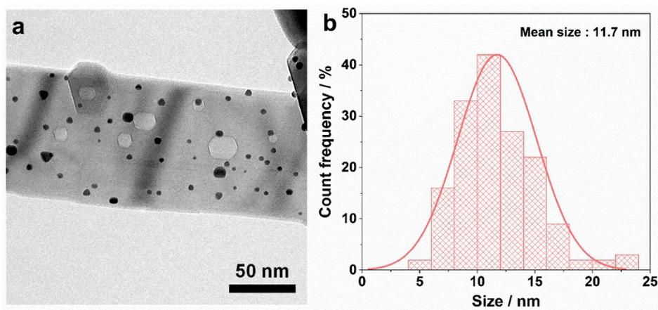
**Figure S7.** (a) TEM image of Pt-NPs/TiO<sub>2</sub> after the treatment in N<sub>2</sub> atmosphere at 700 °C for 5 h. (b) Histograms of Pt particle size distribution of the catalyst in (a).
