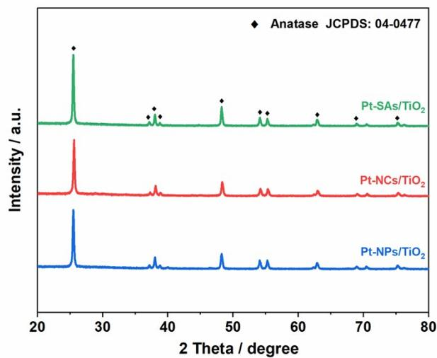
**Figure S4.** XRD patterns of Pt-NPs/TiO<sub>2</sub>, Pt-NCs/TiO<sub>2</sub> and Pt-SAs/TiO<sub>2</sub>. New peaks that can be attributed to the rutile TiO<sub>2</sub> phase can not be found, indicating that no phase transition would occur at the treatment temperature in this experiment.
