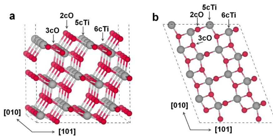
**Figure S8.** (a) Side and (b) top views of anatase TiO<sub>2</sub>(101) surface. The red means O atom and the grey means Ti atom.
