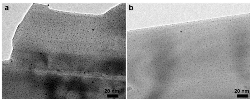
**Figure S3.** TEM images of the catalysts with Pt loading amount of (a) 0.5 wt.% and (b) 0.1 wt.% after treated in 10 vol.% H<sub>2</sub>/Ar atmosphere at 700 °C.
