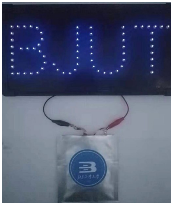
Figure S18. Soft-pack batteries (five batteries in series) for lighting up a set of LED lights.
