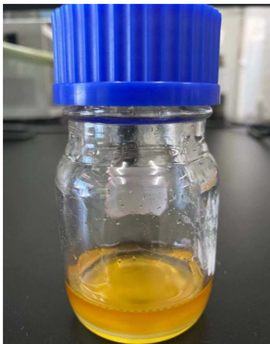
Figure S1. An optical image of the viscous solution containing the N-rich polymer precursor and well-dissolved \text{Zn}(\text{NO}_3)_2 \cdot 6\text{H}_2\text{O} for preparing HPCK.
