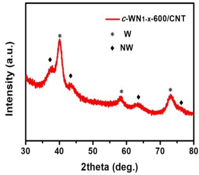
**Fig. S10** XRD patterns of  $c\text{-WN}_{1-x}\text{/CNTs}$  annealed at 600 °C under  $\text{H}_2$  flow.
