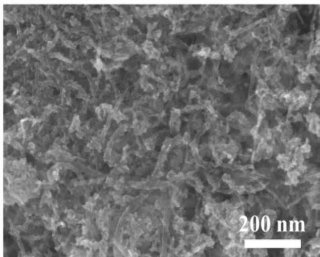
**Fig. S2** SEM image of Co(OH)<sub>2</sub>/c-WN<sub>1-x</sub>/CNTs catalysts.
