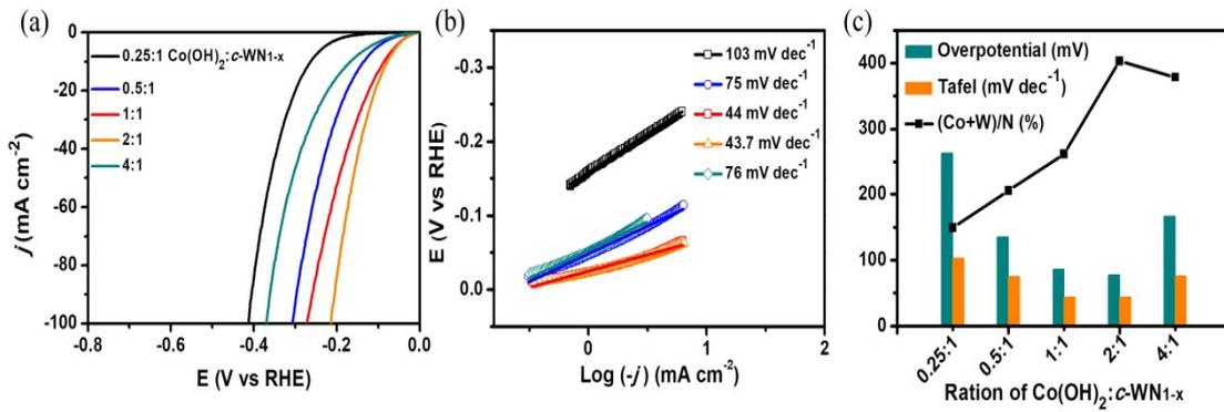
**Fig. S4** (a) Polarization curves; (b) Tafel slope and (c) Histogram of overpotential for achieving current density of  $10 \text{ mA cm}^{-2}$ , Tafel slope and dot plot of surface atomic ratio  $((\text{Co}+\text{W})/\text{N})$  for  $\text{Co}(\text{OH})_2/\text{c-WN}_{1-x}/\text{CNTs}$  catalysts with different mole ratios.
