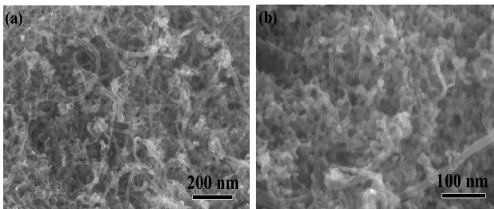
**Fig. S8** SEM images of  $c\text{-WN}_{1-x}/\text{CNTs}$  at different magnifications.
