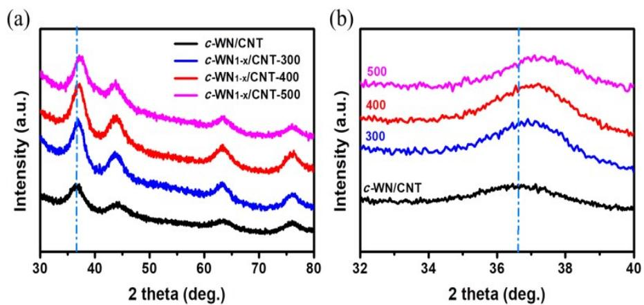
**Fig. S7** XRD patterns of  $c$ -WN/CNTs and  $c$ -WN<sub>1-x</sub>/CNTs annealed at 300, 400 and 500 °C
