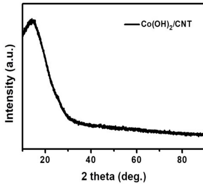
Fig. S1 XRD pattern of Co(OH)<sub>2</sub>/CNTs.
