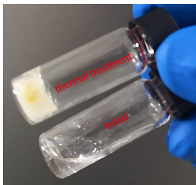
Fig. S1. Photographs of DPPA before and after thermal treatment.
