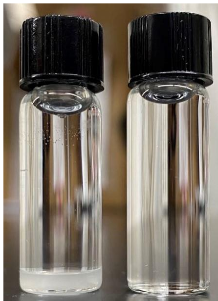
Figure S5. Pictures for the formation of SiW40-P123-10 coacervate and the corresponding supernatant prepared with SiW solution at pH=1.14 (left) and the mixture of 40 wt% SiW (pH=1.75) and 10 wt% P123 aqueous solutions (right).
