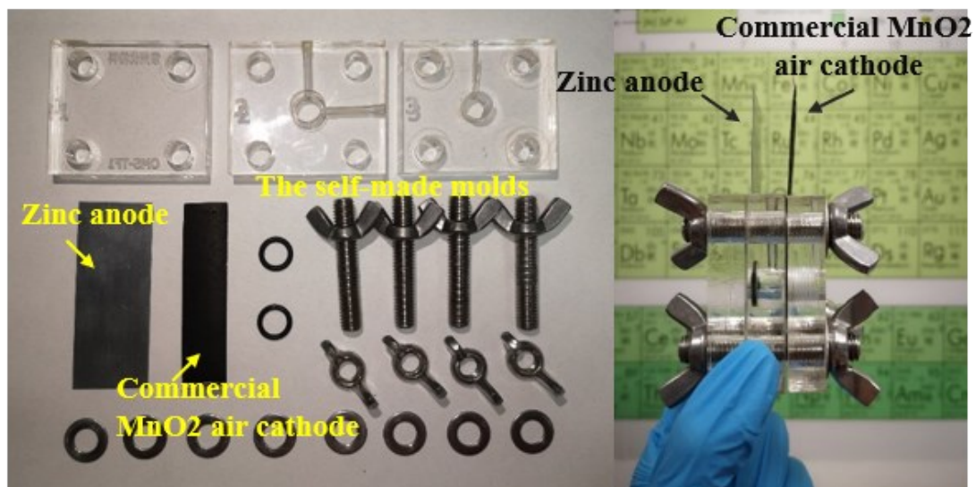
Figure S15. Optical image of the mold for zinc-air battery.
