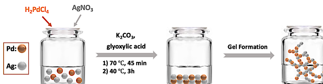
Figure S1. Schematic of the general fabrication process of Pd x Ag y aerogels
