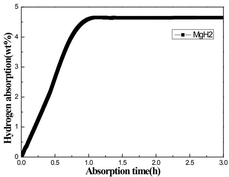
Fig. S10 Absorption property of commercial  $\text{MgH}_2$  at  $250^\circ\text{C}$  under 5MPa of  $\text{H}_2$ .
