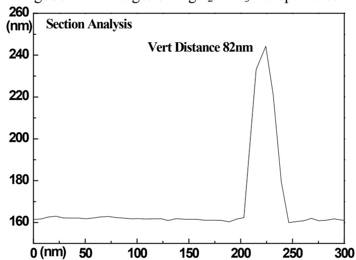
Fig. S9 Section analysis of 95%-2.5 $\text{MgH}_2/\text{AlH}_3@5\%\text{CNTs}$
