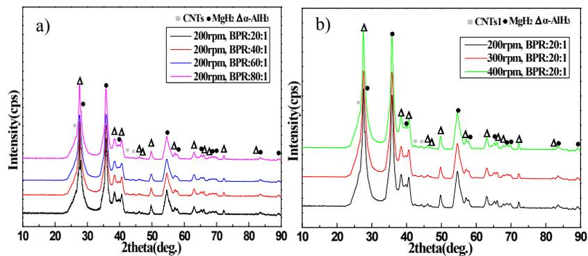
Fig. S5 XRD patterns of as-milled  $MgH_2/AlH_3@CNTs1$  obtained by milling with different ball to powder ratio and rotating speed for 1h
