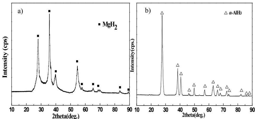
Fig. S1 XRD patterns of as-prepared a)  $\text{MgH}_2$  phase, b)  $\text{AlH}_3$  phase
