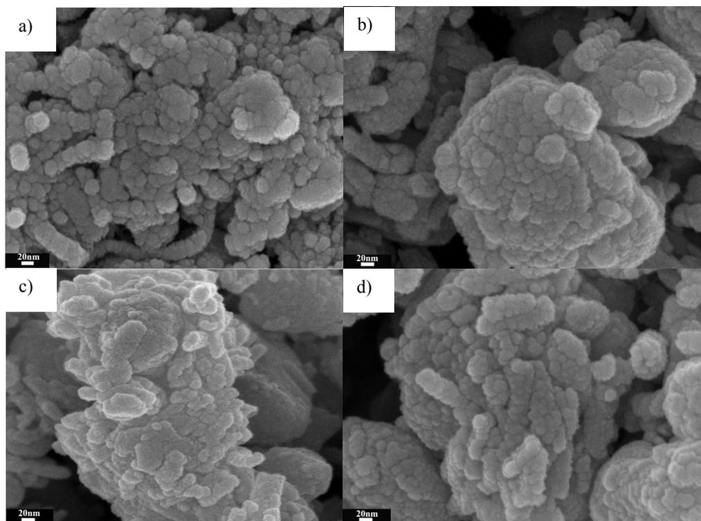
Fig. S6 SEM images of  $\text{MgH}_2/\text{AlH}_3$  wrapped with various CNTs: a)  $\text{MgH}_2/\text{AlH}_3@\text{CNTs}_4$ , b)  $\text{MgH}_2/\text{AlH}_3@\text{CNTs}_1$ , c)  $\text{MgH}_2/\text{AlH}_3@\text{CNTs}_2$ , d)  $\text{MgH}_2/\text{AlH}_3@\text{CNTs}_3$
