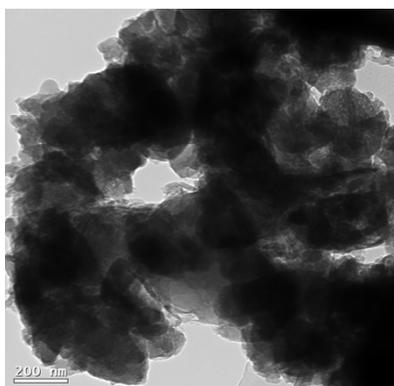
Fig. S8 TEM images of  $\text{MgH}_2/\text{AlH}_3$  nanoparticles
