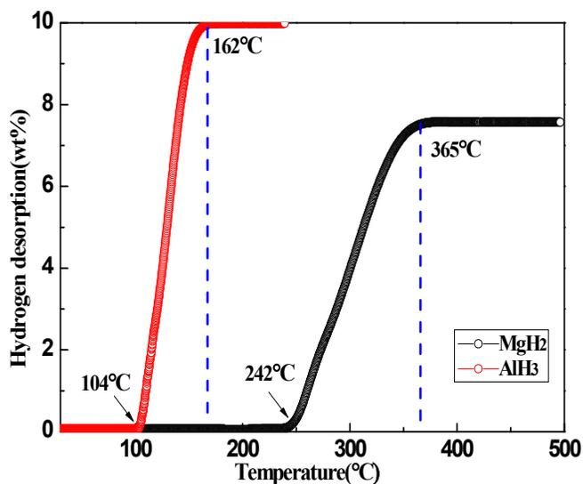
Fig. S2 temperature programmed desorption of a)  $\text{MgH}_2$ , b)  $\text{AlH}_3$ . Samples were heated from room temperature to  $500^{\circ}\text{C}$  with a rate of  $10^{\circ}\text{C}/\text{min}$ .
