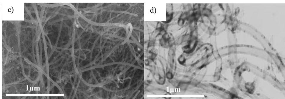
Fig. S3 SEM images of various CNTs: a)CNTs4, b)CNTs1, c)CNTs2, d)CNTs3.
