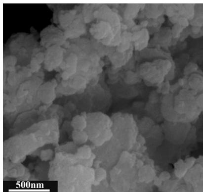
Fig. S7 SEM images of  $\text{MgH}_2/\text{AlH}_3$  nanoparticles
