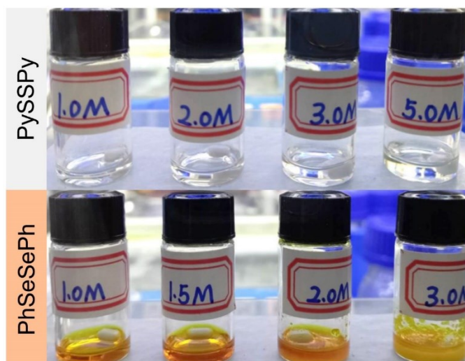
Fig. S2. Solubility test for PySSPy and PhSeSePh. Optical images of PySSPy and PhSeSePh solutions with different concentrations in the supporting electrolyte. For the PySSPy solutions, four bottles were added 44.1, 88.2, 132.2, and 220.3 mg PySSPy, respectively, corresponding concentrations are 1.0 M, 2.0 M, 3.0 M, and 5.0 M, respectively. As for the PhSeSePh solutions, the mass (corresponding concentration) of PhSeSePh in the four bottles are 62.4 (1.0), 93.7 (1.5), 124.8 (2.0), and 187.3 mg (3.0 M), respectively. The volume of electrolyte in every bottle is 0.2 mL. Each sample was stirred for 1 hour before taking pictures.
