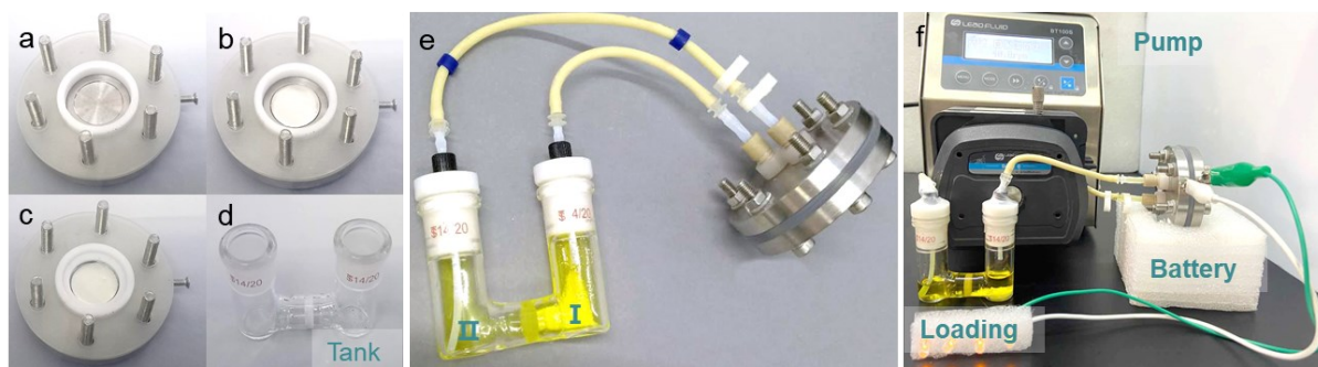
Fig. S3. Photograph of the self-designed flow battery system. a-c, Assembly process of the flow battery and d, A reservoir with two storage tanks which are linked by a diaphragm and e, A flow battery, f, Digital photograph of a complete flow battery system.
