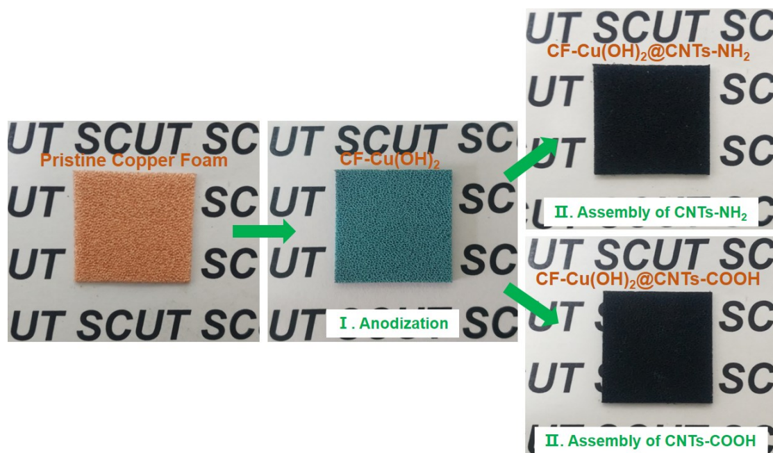
Fig. S2 Digital pictures of the pristine copper foam, CF-Cu(OH) 2 , CF-Cu(OH) 2 @CNTs-NH 2 and CF-Cu(OH) 2 @CNTs-COOH.
