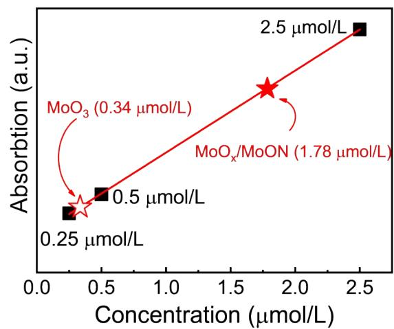
Figure S6 Dye absorption measurements of  $\text{MoO}_x$  nanotubes and  $\text{MoO}_x/\text{MoON}$  nanotubes.
