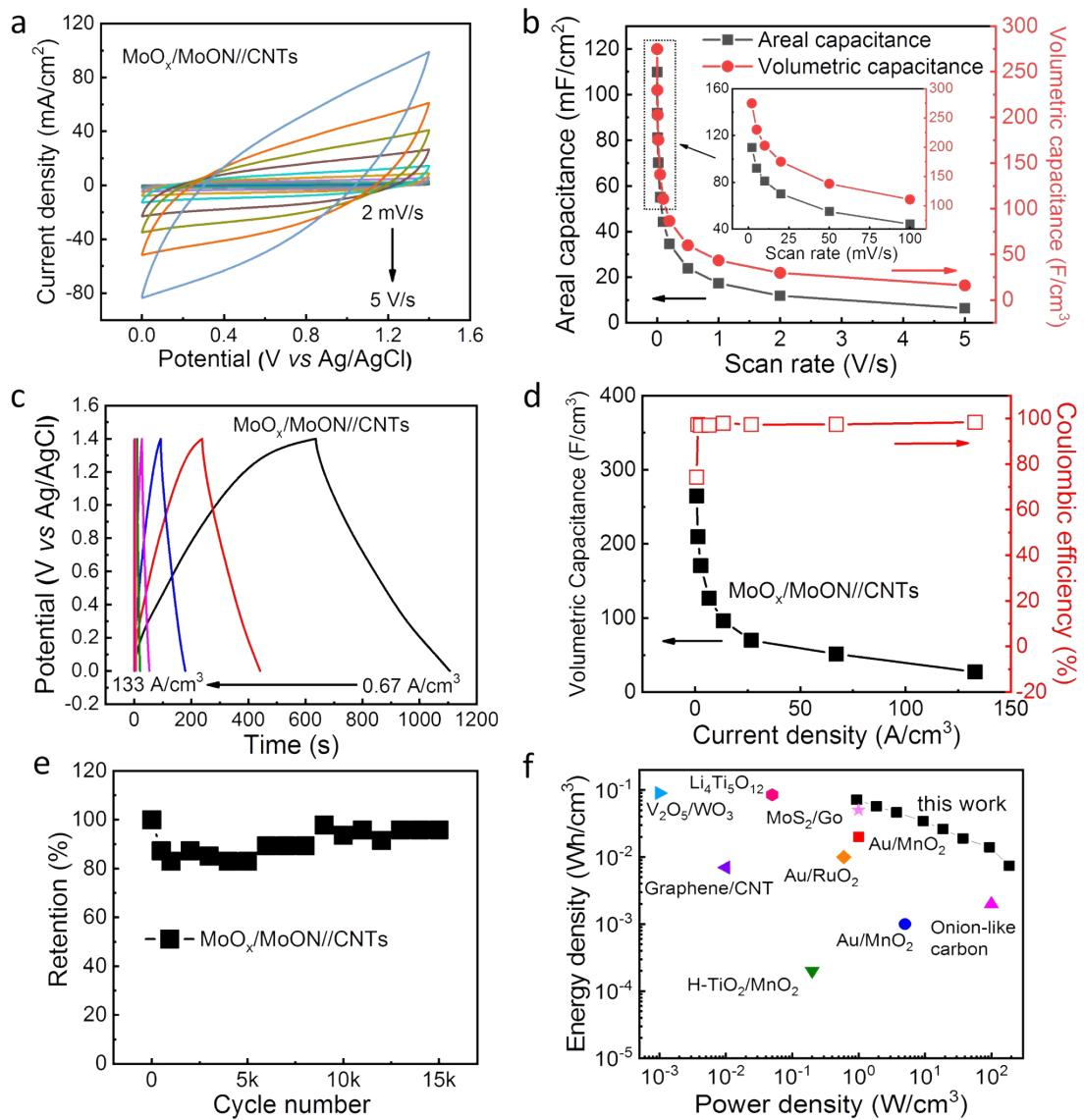
Figure S22 Electrochemical performances of asymmetric supercapacitor (a) CV plots at different scan rates; (b) areal capacitance and volumetric capacitance based on CV plots; (c) GCD plots at different charging rates; (d) volumetric capacitance at different charging rates based on GCD plots; (e) capacitance retention during cycling. (f) volumetric energy density of the ASC<sup>6-8</sup>.
