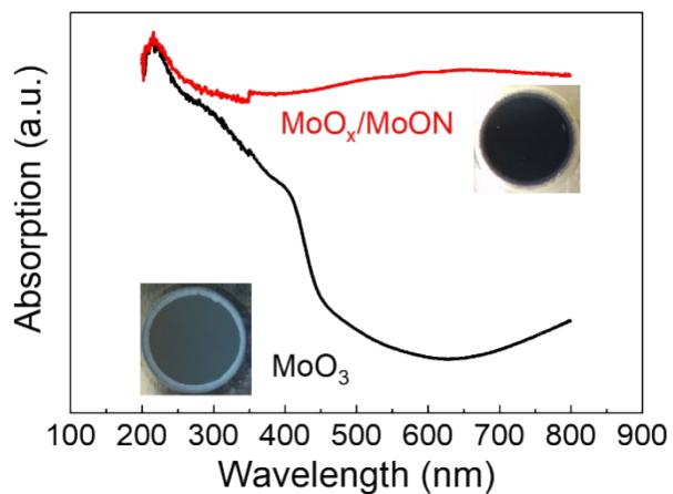
Figure S3 UV-Vis absorption spectra of MoO<sub>3</sub> and MoO<sub>x</sub>/MoON nanotubes (inset: optical photos).
