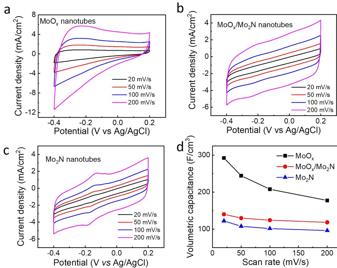
Figure S14 CV plots of (a) MoO<sub>x</sub> nanotubes; (b) MoO<sub>x</sub>/Mo<sub>2</sub>N nanotubes; (c) Mo<sub>2</sub>N nanotubes; (d) relationships between scan rate and capacitance.
