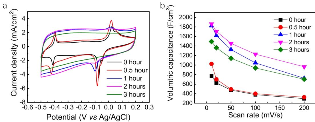
Figure S12 Electrochemical performance of  $\text{MoO}_3$  nanotubes ammonified at 350 °C for different time (a) CV plots and (b) volumetric capacitances.
