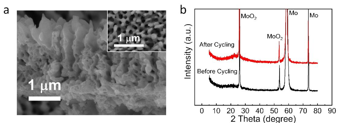
Figure S18 Morphology and crystal phase characterizations of  $\text{MoO}_x/\text{MoON}$  nanotubes after cycling (a) SEM images and (b) XRD patterns.
