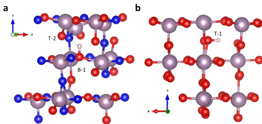
Figure S1 Optimized intercalation configuration for  $\text{H}^+$  into MoON (a) and  $\text{MoO}_x$  (b).
