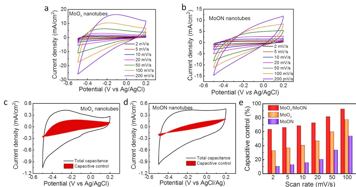
Figure S13 CV plots with different scan rates of  $\text{MoO}_x$  nanotubes (a) and  $\text{MoON}$  nanotubes (b); CV curve recorded with 2 mV/s of  $\text{MoO}_x$  (c) and  $\text{MoON}$  nanotubes (d) (shade curve is capacitive-controlled capacitance); (e) ratios of capacitive-controlled capacitance of  $\text{MoO}_x$  nanotubes and  $\text{MoON}$  nanotubes in total capacitance at different scan rates.
