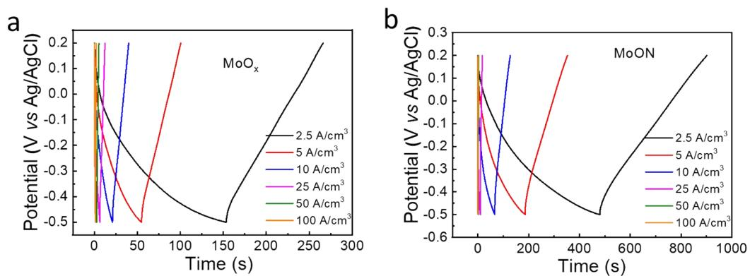
Figure S17 GCD plots of  $\text{MoO}_x$  nanotubes (a) and MoON nanotubes (b).
