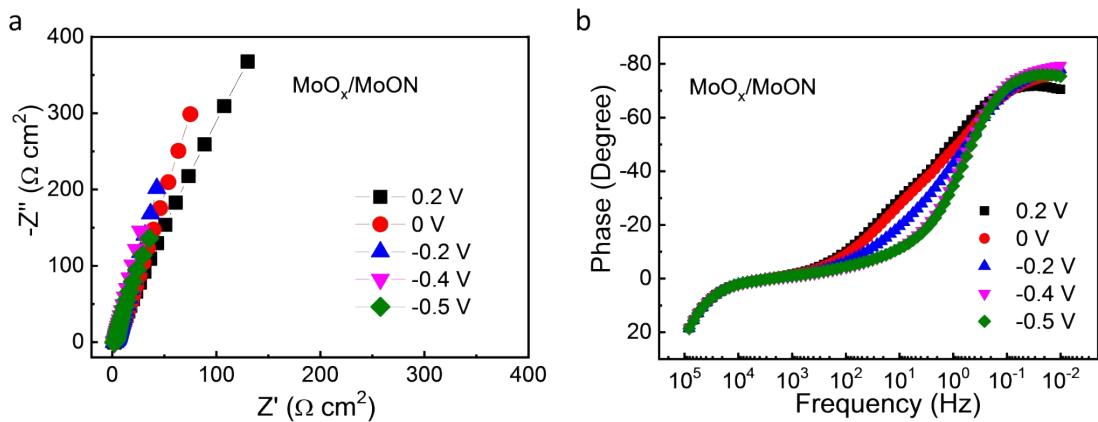
Figure S16 Nyquist plots (a) and corresponding Bode plots (b) of  $\text{MoO}_x/\text{MoON}$  electrode at different potentials.
