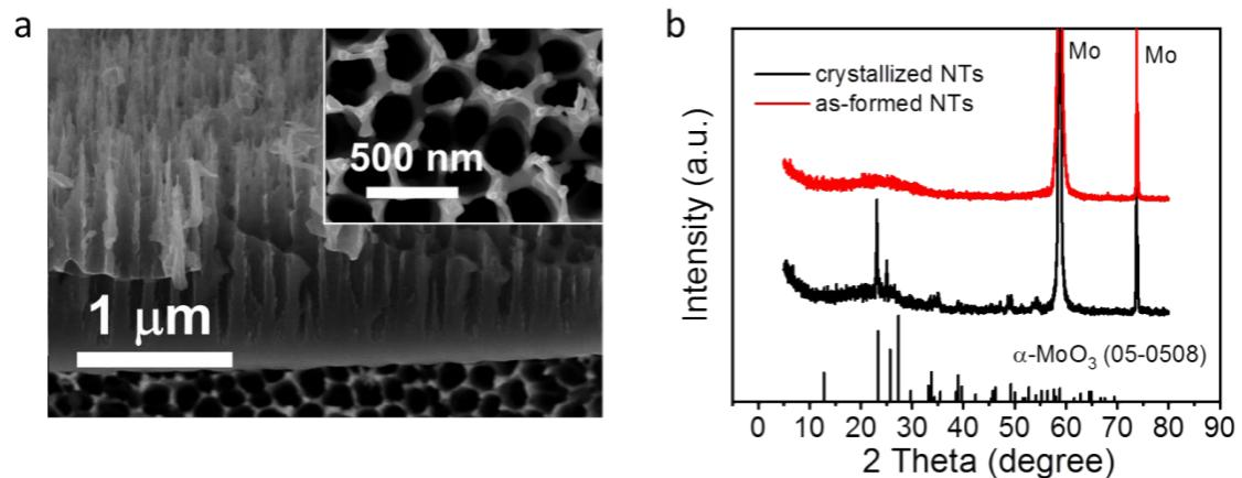
Figure S2 (a) SEM images of as-formed MoO<sub>3</sub> nanotubes; (b) XRD patterns of as-formed and crystallized MoO<sub>3</sub> nanotubes.
