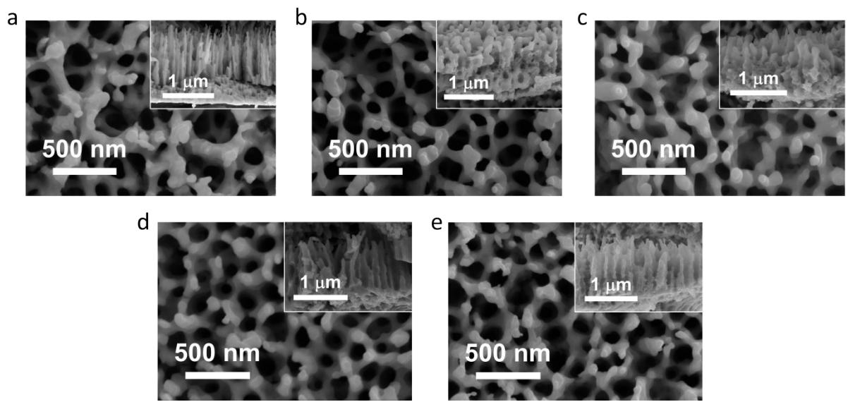
Figure S4 SEM images of  $\text{MoO}_3$  nanotubes with ammonification for 2 h at (a) 300 °C; (b) 400 °C; (c) 450 °C and at 350 °C for 1 h (d) and 3 h (e).
