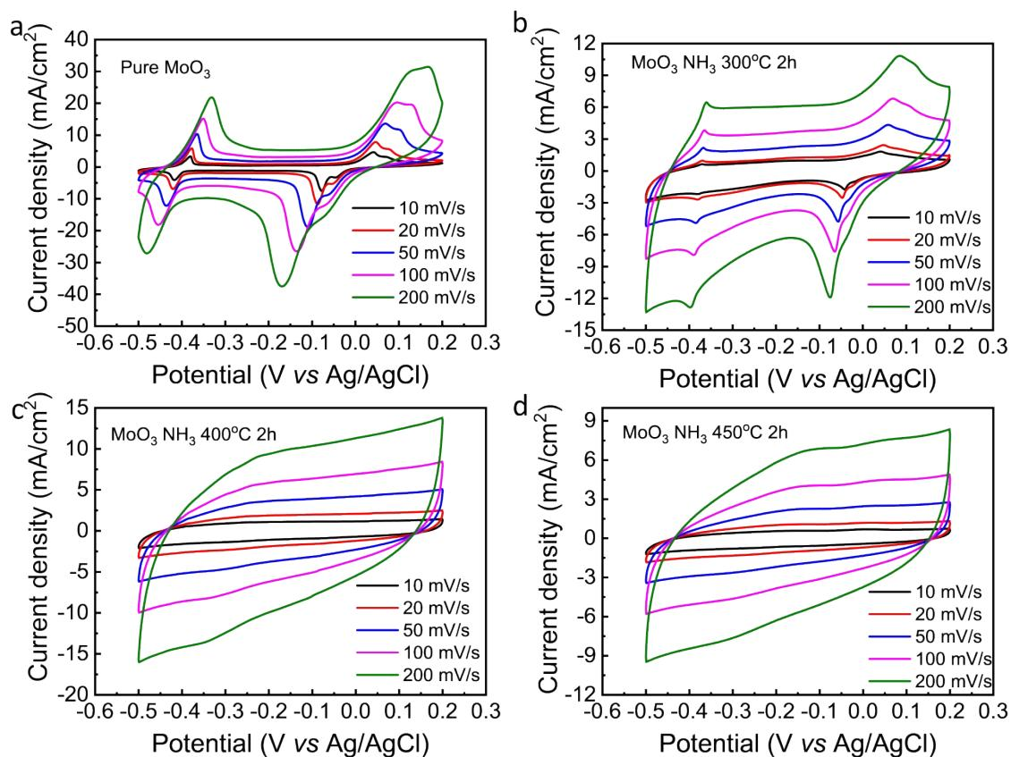
Figure S11 CV plots of  $\text{MoO}_3$  nanotubes ammonified at different temperatures for 2 h (a) crystallized  $\text{MoO}_3$ ; (b) 300 °C; (c) 400 °C; (d) 450 °C.
