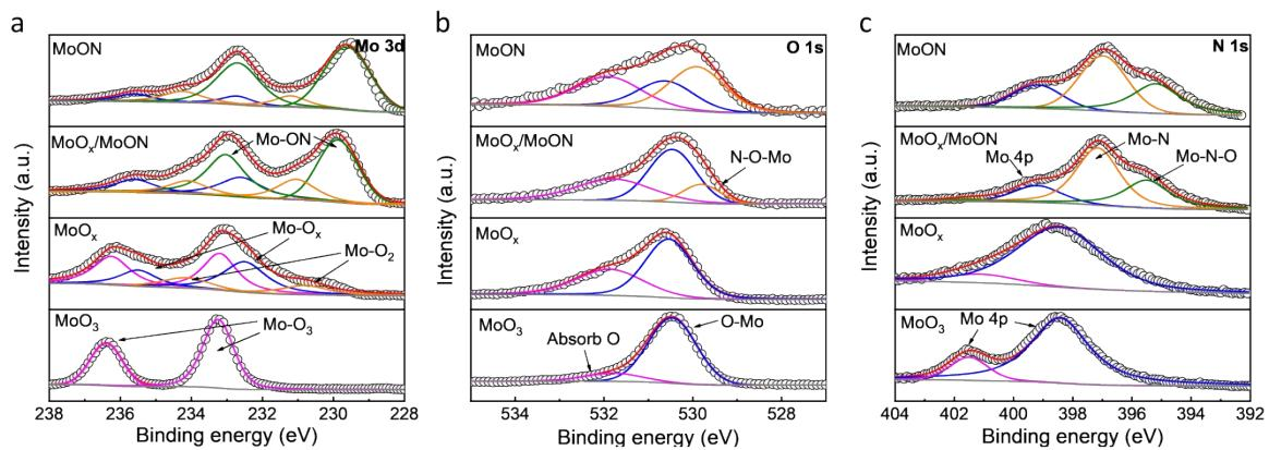
Figure S9 High resolution XPS spectra of  $\text{MoO}_3$ ,  $\text{MoO}_x$ ,  $\text{MoO}_x/\text{MoON}$  and  $\text{MoON}$ : (a) Mo 3d; (b) O 1s, and (c) N 1s.
