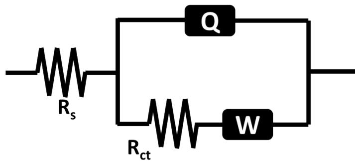
Figure S15 Randles equivalent circuit of EIS results in Fig. 5f.
