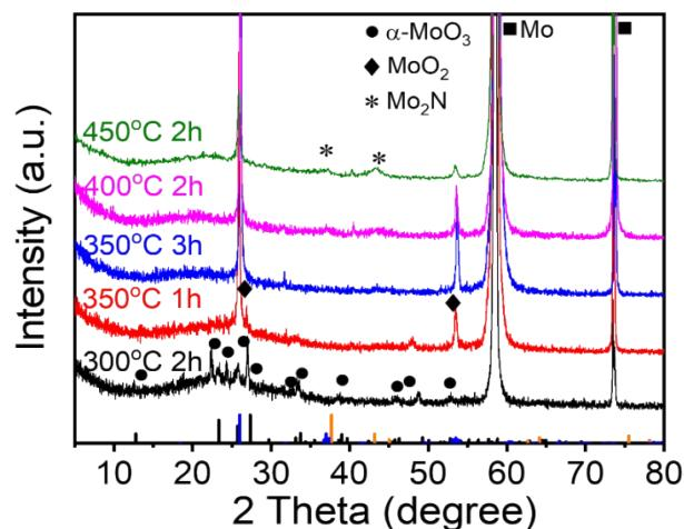
Figure S7 XRD patterns of  $\text{MoO}_3$  nanotubes after ammonification at different temperatures and durations.
