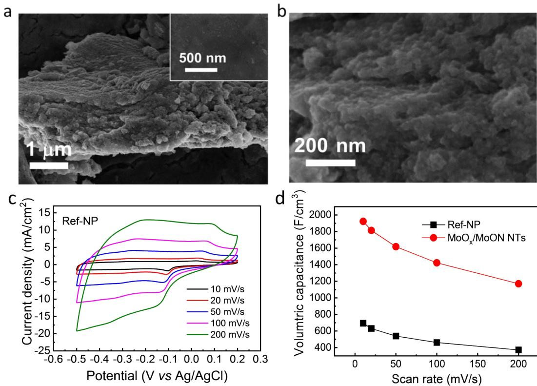
Figure S20 (a,b) SEM images of MoO<sub>x</sub>/MoON nanotubes with 3  $\mu$ m thickness; (c) CV plots of MoO<sub>x</sub>/MoON with 3  $\mu$ m thickness (d) volumetric capacitances of MoO<sub>x</sub>/MoON nanotubes with different thicknesses.
