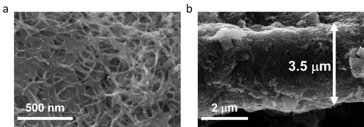
Figure S24 SEM images of CNTs electrode: (a) surface and (b) cross-section.
