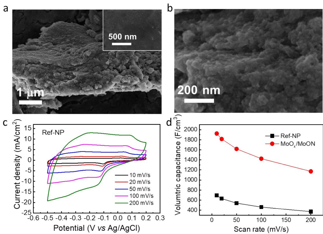
Figure S19 (a,b) SEM images of  $\text{MoO}_x/\text{MoON}$  nanoporous (Ref-NP); (c) CV plots of Ref-NP at different scan rates; (d) volumetric capacitance of  $\text{MoO}_x/\text{MoON}$  nanotubes and Ref-NP.
