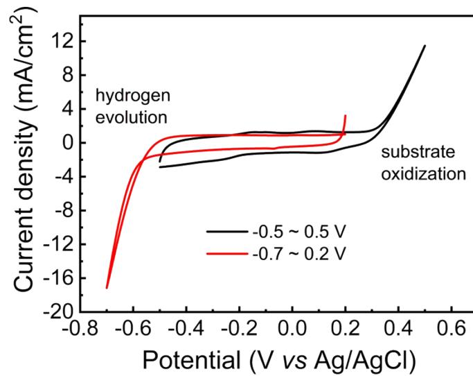
Figure S10 CV curves of  $\text{MoO}_x/\text{MoON}$  nanotubes with different potential ranges.
