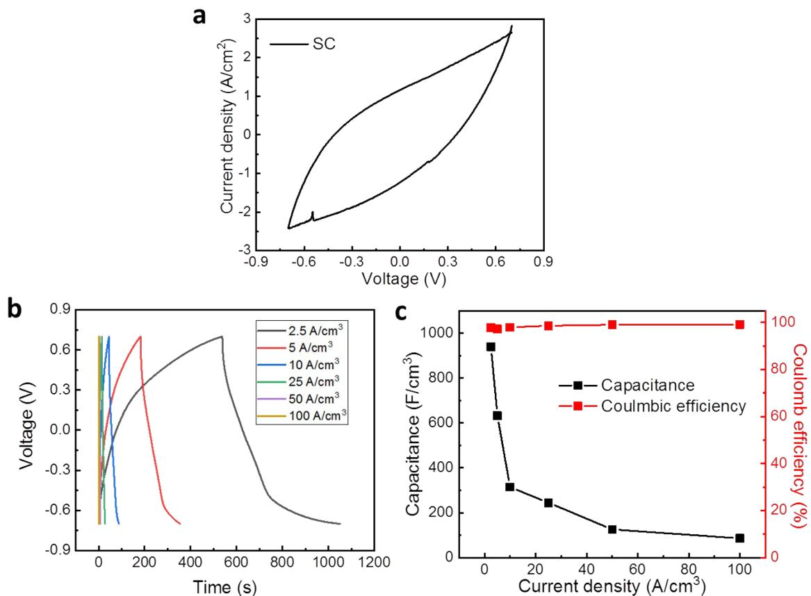
Fig. S23 Performance of SC device (a) the CV plot of SC device at 20 mV/s. (b) GCD plots of SC device at different current densities (c) Capacitance and Coulombic efficiency of SC device.
