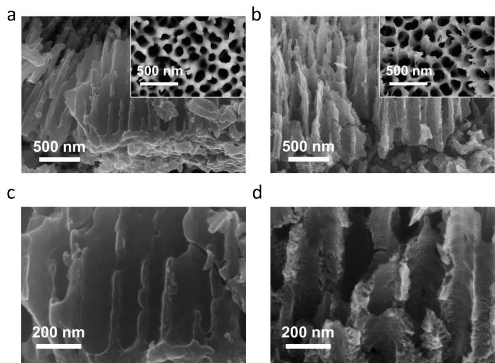
Figure S5 SEM images of (a)  $\text{MoO}_x$  nanotubes; (b)  $\text{MoON}$  nanotubes, and the tube walls of
