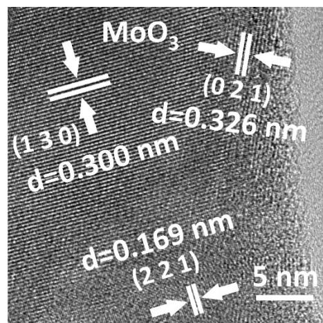
Figure S8 HRTEM image of  $\alpha$ -MoO<sub>3</sub> nanotubes
