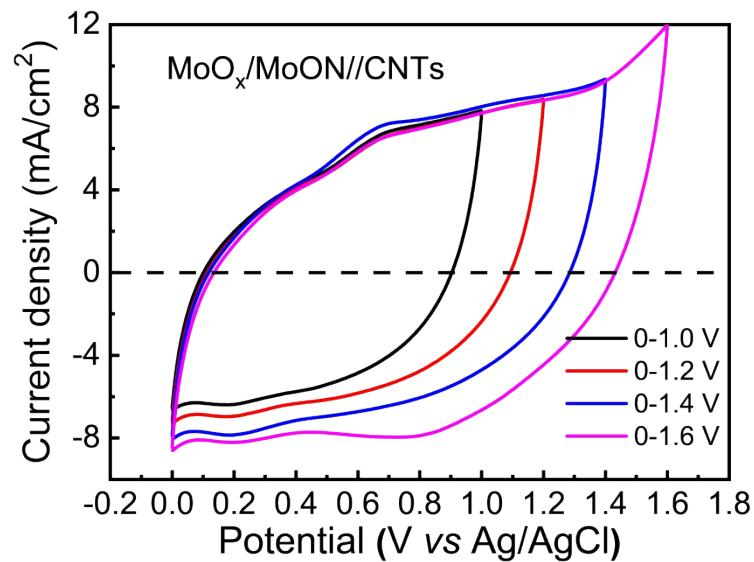
Figure S21 Asymmetric capacitor based MoO<sub>x</sub>/MoON/CNTs in different voltage ranges.
