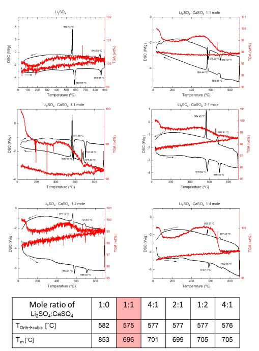
**Figure S1.** Melting temperature of the sensing electrode as a function of its composition determined via DSC/TGA analysis of different mole ratios of  $Li_2SO_4$ :CaSO<sub>4</sub>. The measurement was conducted under synthetic air from room temperature to 900 °C, held for 5 min, and cooled back to room temperature at a ramp rate of 10 °C/min for both the heating and cooling steps. The melting temperatures are also summarized in the table above.
