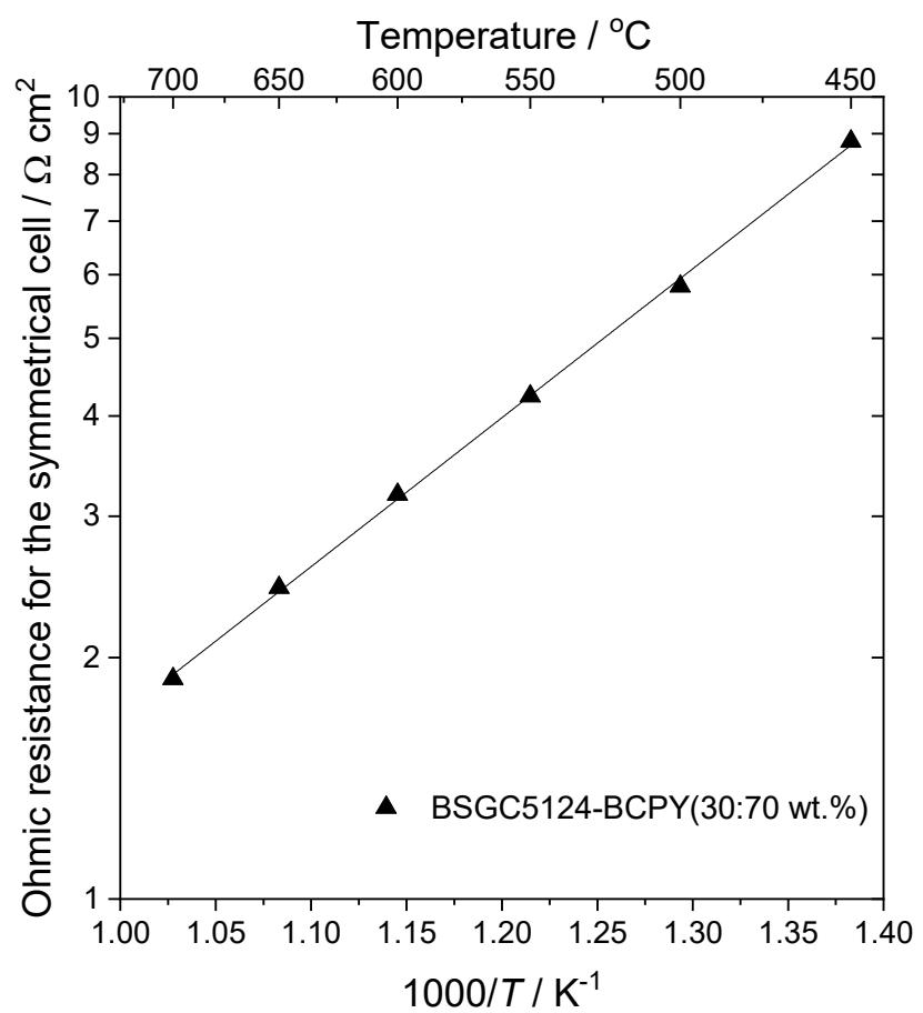
Fig. S5 Temperature dependence of ohmic resistance for the symmetrical cell employing BSGC5124-BCPY (30:70 wt.%) composite electrodes used in Fig. 4. Atmosphere; 3 vol.% humidified synthetic air.
