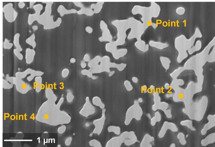
Fig. S6 Cross-sectional SEM image of the BSGC5124–BCPY (30:70 wt.%) composite electrode. The black part corresponds to the pore. Firing temperature of the composite electrode; 1000 °C.
