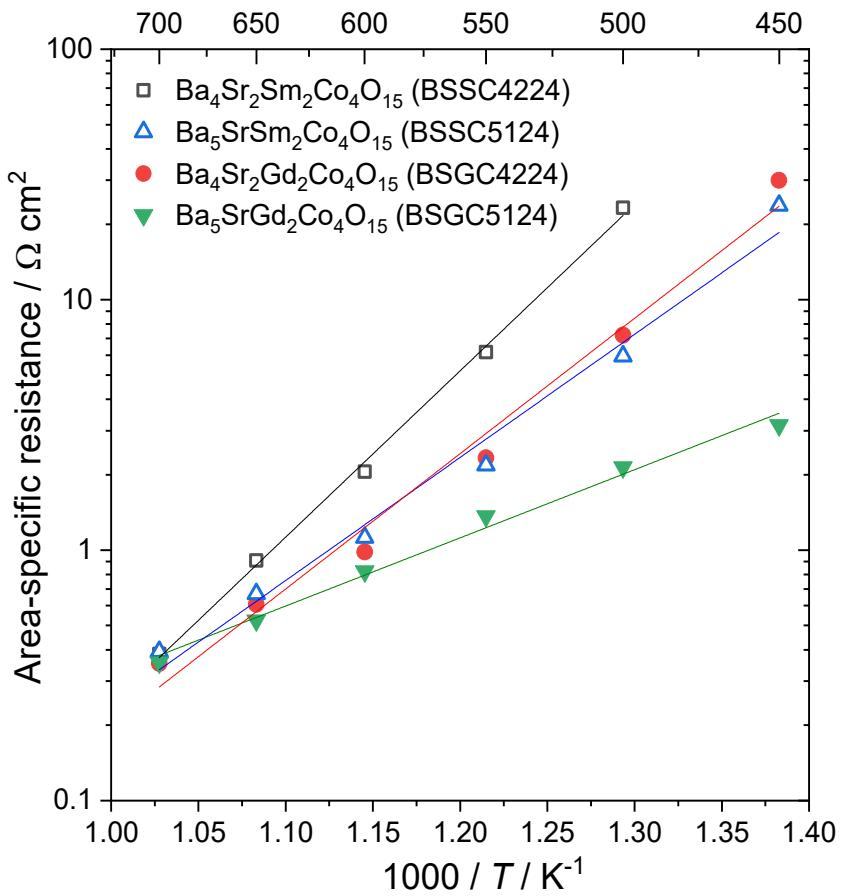
Fig. S3 Temperature dependence of area-specific resistance of  $(\text{Ba}_{6-x}\text{Sr}_x)\text{Gd}_2\text{Co}_4\text{O}_{15}$  and  $(\text{Ba}_{6-x}\text{Sr}_x)\text{Sm}_2\text{Co}_4\text{O}_{15}$  ( $x = 1, 2$ ) electrodes in 3 vol.% humidified synthetic air. All oxides were fired on the BCY disk at 1200 °C.
