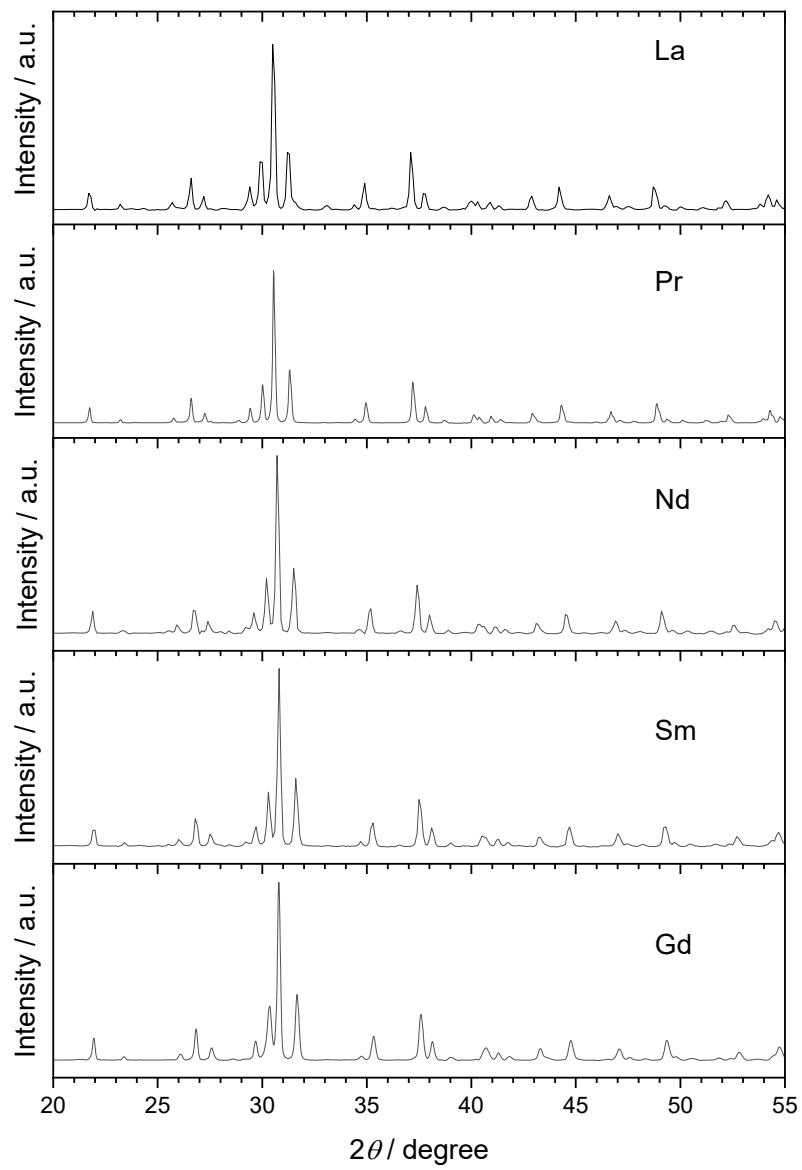
Fig. S2 XRD patterns of  $\text{Ba}_5\text{Sr}RE_2\text{Co}_4\text{O}_{15}$  ( $RE = \text{La}, \text{Pr}, \text{Nd}, \text{Sm}$ , and  $\text{Gd}$ ).
