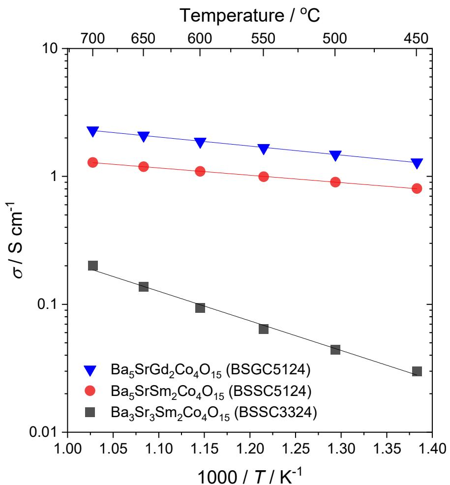
Fig. S4 Temperature dependence of total electrical conductivity of  $(\text{Ba}_{6-x}\text{Sr}_x)\text{Sm}_2\text{Co}_4\text{O}_{15}$  ( $x = 1, 3$ ) and  $\text{Ba}_5\text{SrGd}_2\text{Co}_4\text{O}_{15}$  in 3 vol.% humidified synthetic air. The four-probe dc technique was applied to measure the conductivity with Ag electrodes. All oxides were sintered at 1300 °C for 5 h to prepare dense samples.
