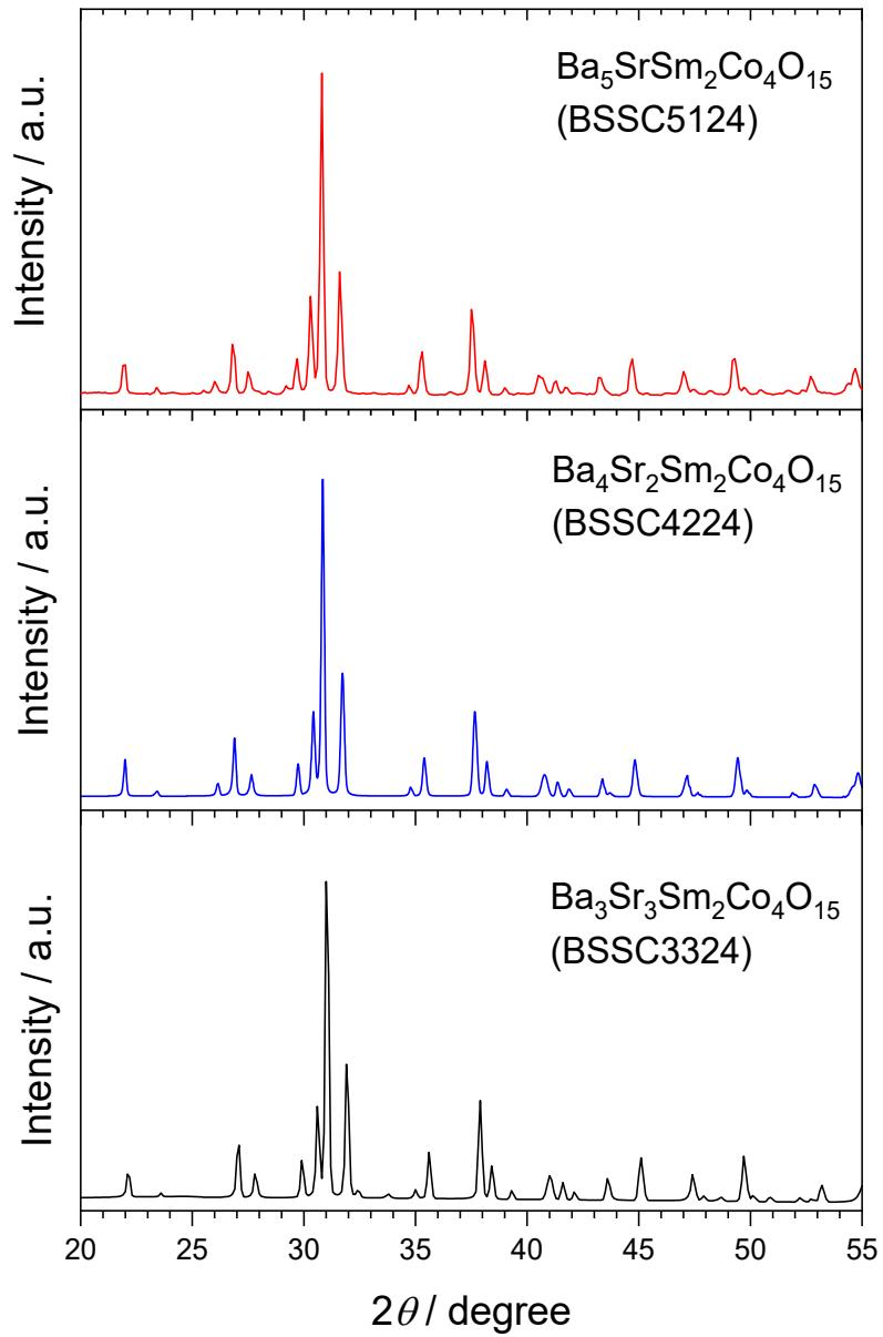
Fig. S1 XRD patterns of  $(\text{Ba}_{6-x}\text{Sr}_x)\text{Sm}_2\text{Co}_4\text{O}_{15}$  ( $x = 1, 2, 3$ ).
