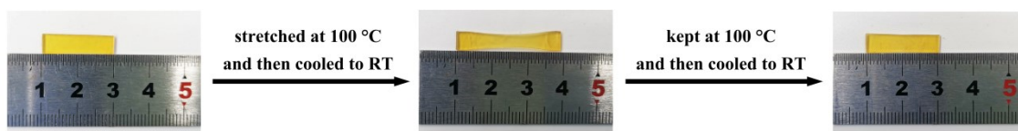
Figure S13. Photograph of temperature-induced shape memory effect cycle of PU film.
