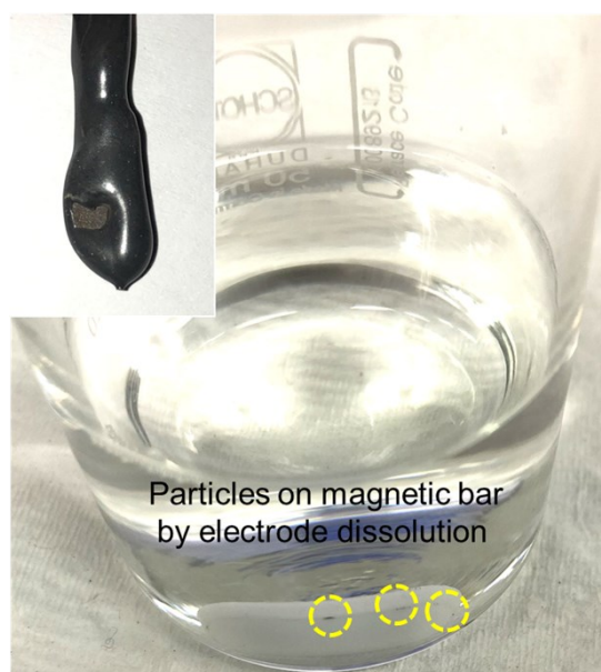
Fig. S11. Dissolution of particles from MMP-1h electrode in 1 M PBS: Particles aggregation on magnetic bar after few hours of HER stability at -50 \text{ mA cm}^{-2} . Inset: electrode image.
