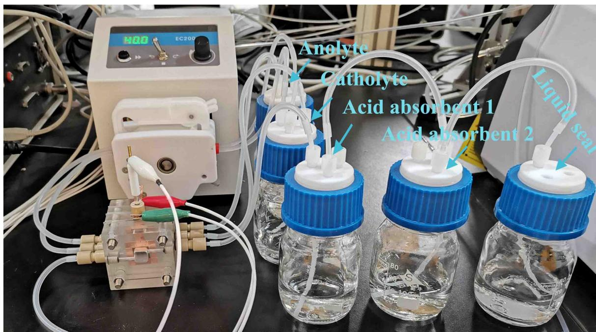
**Supplementary Fig. 28** The electrochemical cell configuration for NRR, which includes a catholyte chamber, anolyte chamber, acid absorbent chamber 1, acid absorbent chamber 2, and liquid seal chamber for the electrolyte and  $\text{NH}_3$  product.
