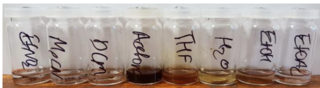
Figure S 13: Picture of a rudimentary solubility test carried out on CABQ in which a micro-spatula full of samples was added to 2 ml of solvent, swirled, and then left to stand. The solvents from left to right are as follows: nitro-ethane, acetonitrile, dichloromethane, acetone, tetrahydrofuran, water, ethanol, ethyl acetate.
