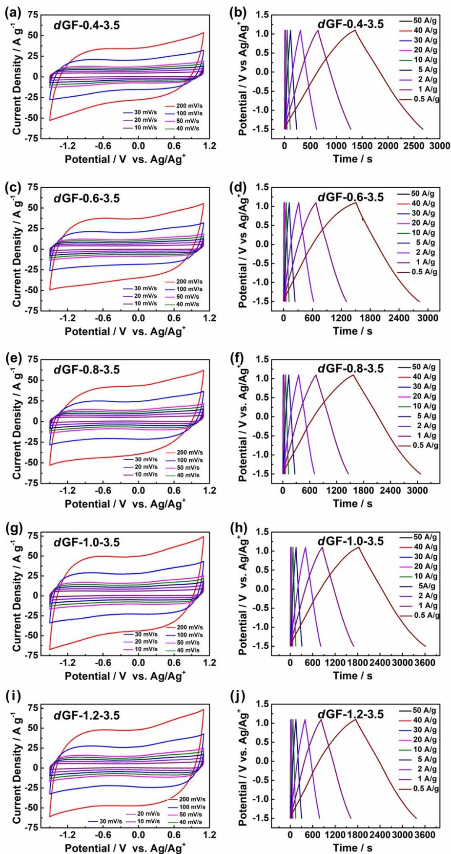
Figure S21. CV curves and GCD curves of *dGFs* with different PSS dosages.
