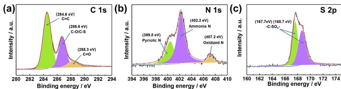
Figure S10. (a) C 1s, (b) N 1s, and (c) S 2p XPS survey of GOF.
