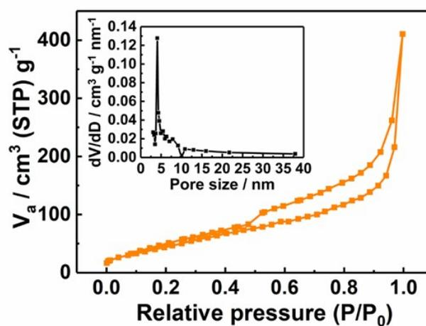
**Figure S16.** The nitrogen adsorption/desorption isotherm and pore distribution for *d*GF-1.0-3.5.
