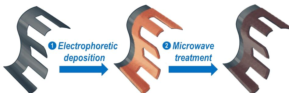
**Figure S24.** The preparation process of the interdigital electrodes.
