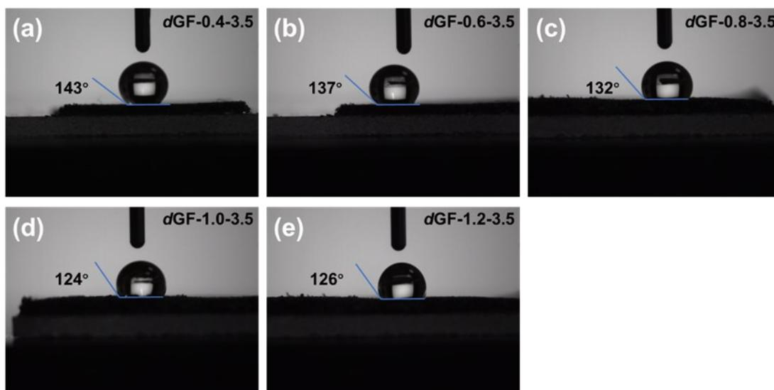
**Figure S20.** The contact angle measuring images of dGF with different PSS dosage.
