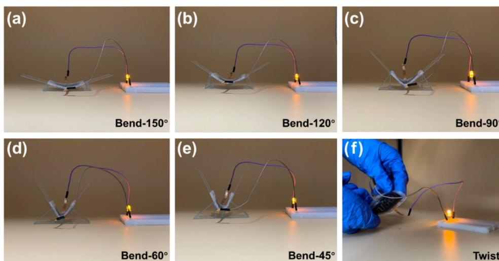
**Figure S26.** Photos of the assembled interdigital supercapacitor lighting up the LED bulb under (a-e) different bending angles and (f) twisting state.
