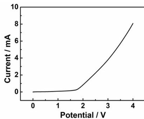
**Figure S3.** LSV curve of the electrolyte for EPD.
