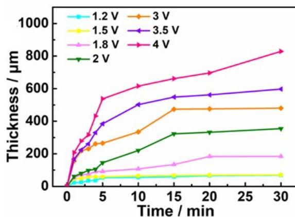
**Figure S13.** The relationship of deposition thickness and time under different EPD voltages.
