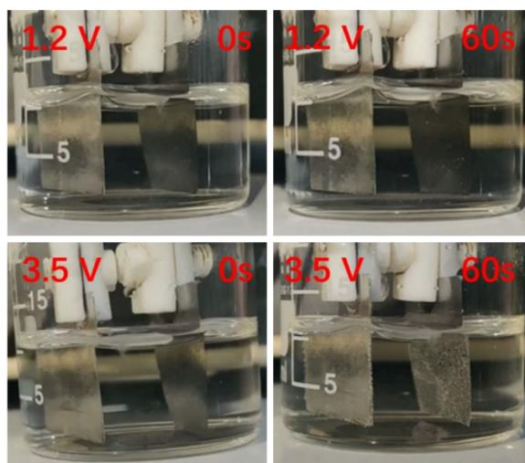
**Figure S4.** Photos of EPD cells in the first 1 min at voltage of 1.2 V and 3.5 V.
