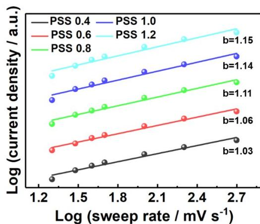
**Figure S23.** The fitting result of CV log (current density) to log (sweep rate) of *dGFs* with different EPD voltages.
