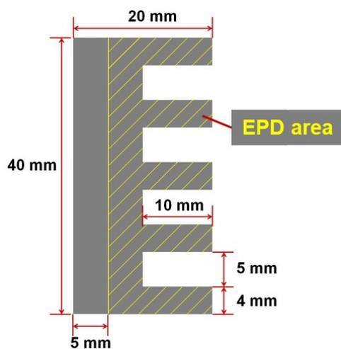
**Figure S28.** The shape of interdigital electrodes.
