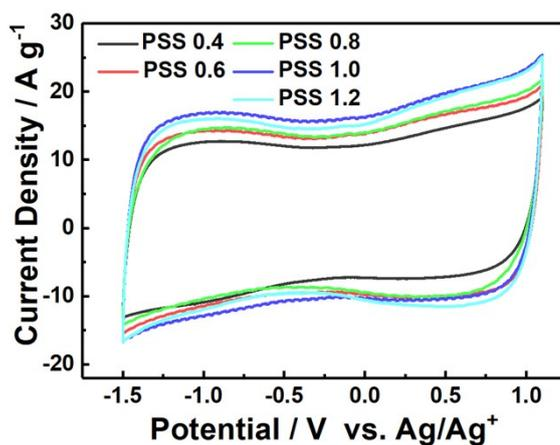
**Figure S22.** The CV curves of *dGFs* with different PSS dosage under  $50 \text{ mV s}^{-1}$ .
