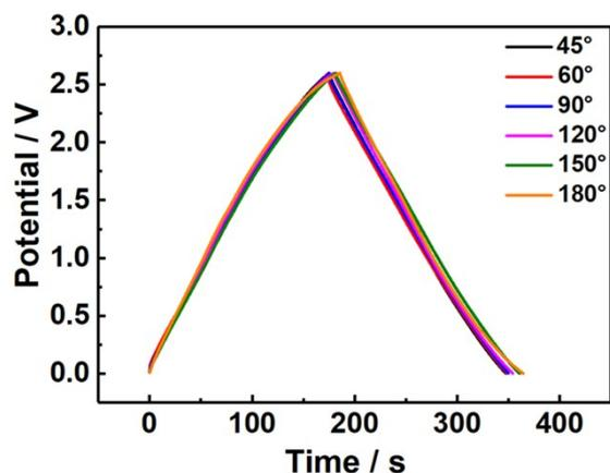
**Figure S25.** GCD curves at  $1 \text{ A g}^{-1}$  of the assembled interdigital supercapacitor under different bending angles.
