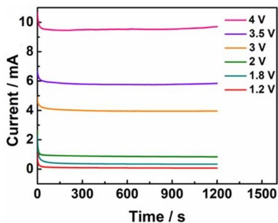
Figure S11. (a) Deposition current-time curves under different EPD voltages.
