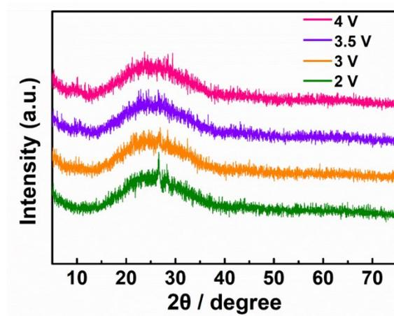
**Figure S15.** XRD patterns of GOF with different EPD voltages.
