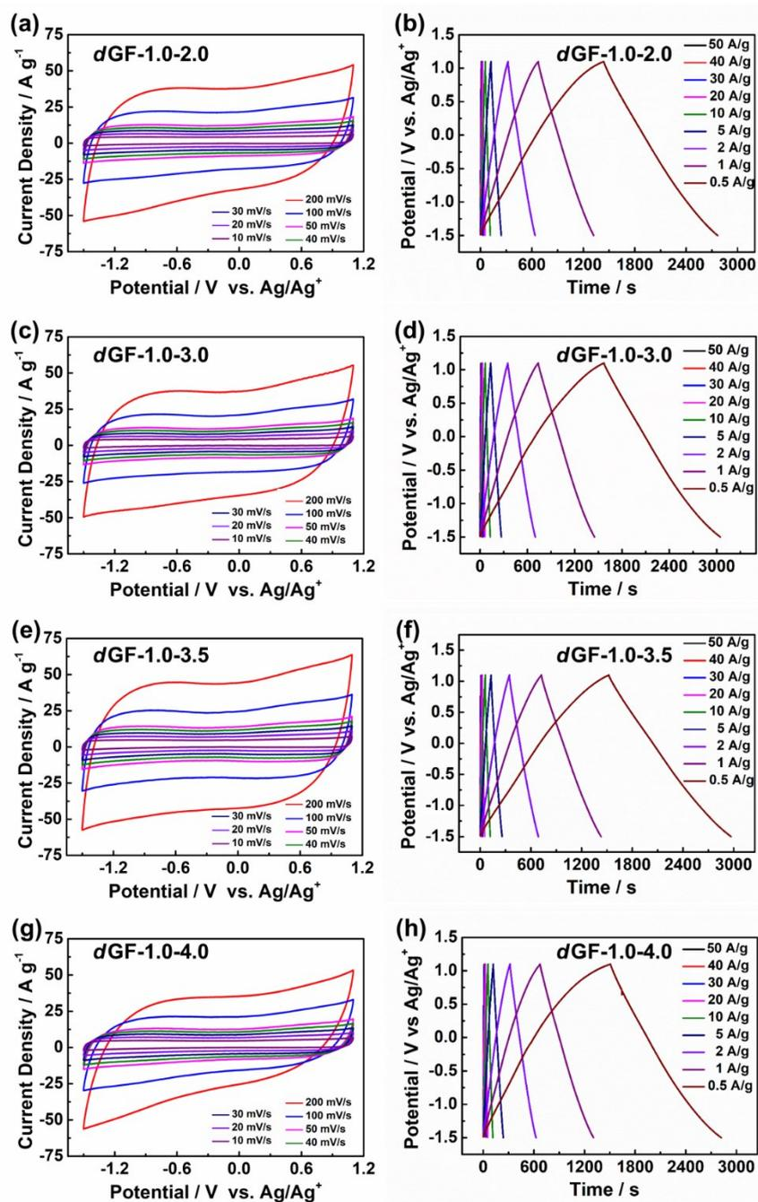
Figure S17. CV curves and GCD curves of *dGFs* with different EPD voltages.
