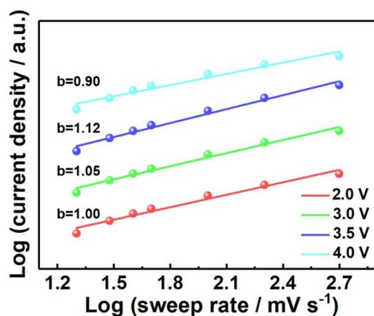
**Figure S19.** The fitting result of CV log (current density) to log (sweep rate) of dGFs with different EPD voltages.
