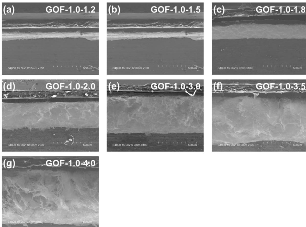
**Figure S12.** (a-g) Cross-sectional FE-SEM images of GOF prepared under different EPD voltages.
