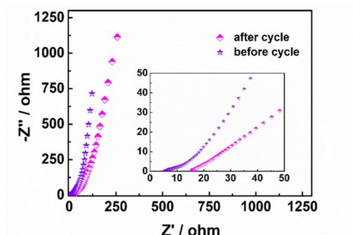
**Figure S27.** EIS of the assembled interdigital supercapacitor before and after 10000 cycles.
