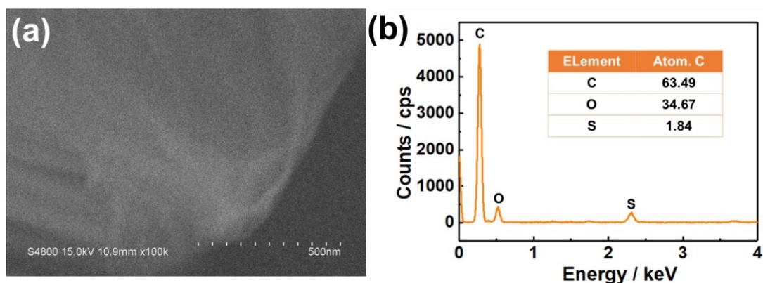
**Figure S1.** (a) High-resolution FE-SEM image and (b) EDS of PSS-GO.
