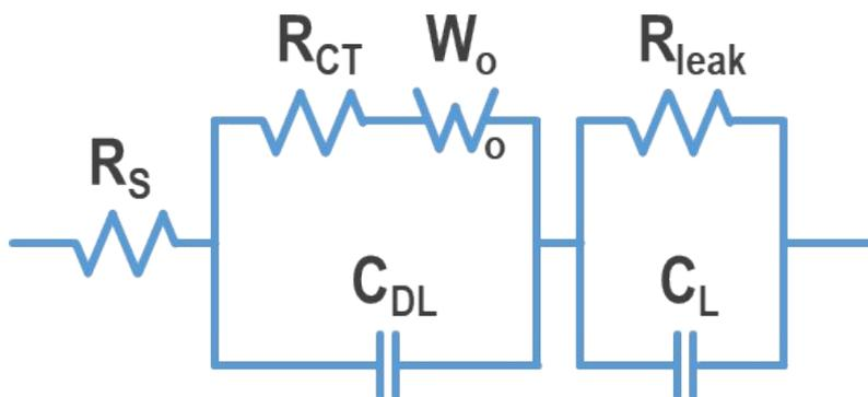
**Figure S18.** Randles equivalent circuit representing the circuit elements in the EIS.
