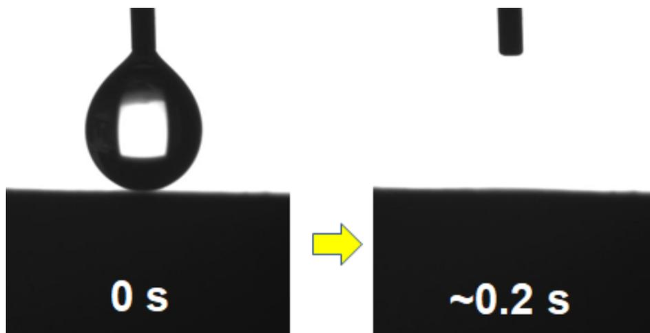
**Figure S4.** Rapid water absorption of V-RGO foam.
