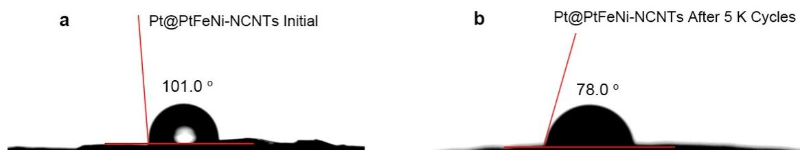
**Figure S21 (a)** The contact angles of the pristine catalyst of Pt@PtFeNi-NCNTs, **(b)** The contact angles of the Pt@PtFeNi-NCNTs catalyst after 5 K cycles.
