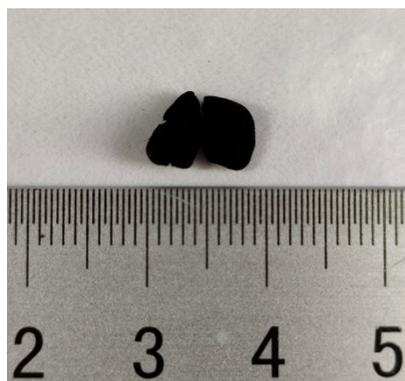
**Figure S1.** Photograph of an Au-Pd-CS-2min aerogel.
