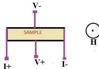
Fig S4: Experimental set-up for measurement of Hall Effect in Sn<sub>0.856</sub>Sb<sub>0.144</sub>O<sub>2</sub>. V stands for voltage, I stands for current and H for magnetic field.
