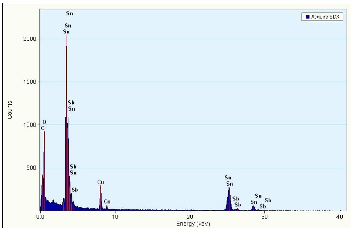
Fig S8: EDX spectrum of  $\text{Sn}_{0.957}\text{Sb}_{0.043}\text{O}_2$  sample. Signals of Cu and C are due to use of copper coated carbon grids during TEM.
