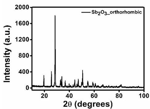
Fig S6: Powder X-ray diffraction pattern of  $\text{Sb}_2\text{O}_3$  (orthorhombic) phase material using  $\text{Cu K}\alpha$  radiation source.
