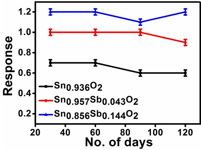
Fig S2: Stability analysis of the antimony doped tin oxide sensors for 120 days. The uncertainty is represented as error bars.
