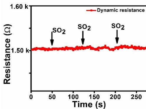
Fig S7: Insensitivity of  $\text{Sb}_2\text{O}_3$  (orthorhombic) sensor to pulses of  $\text{SO}_2$  gas (2 ppm).
