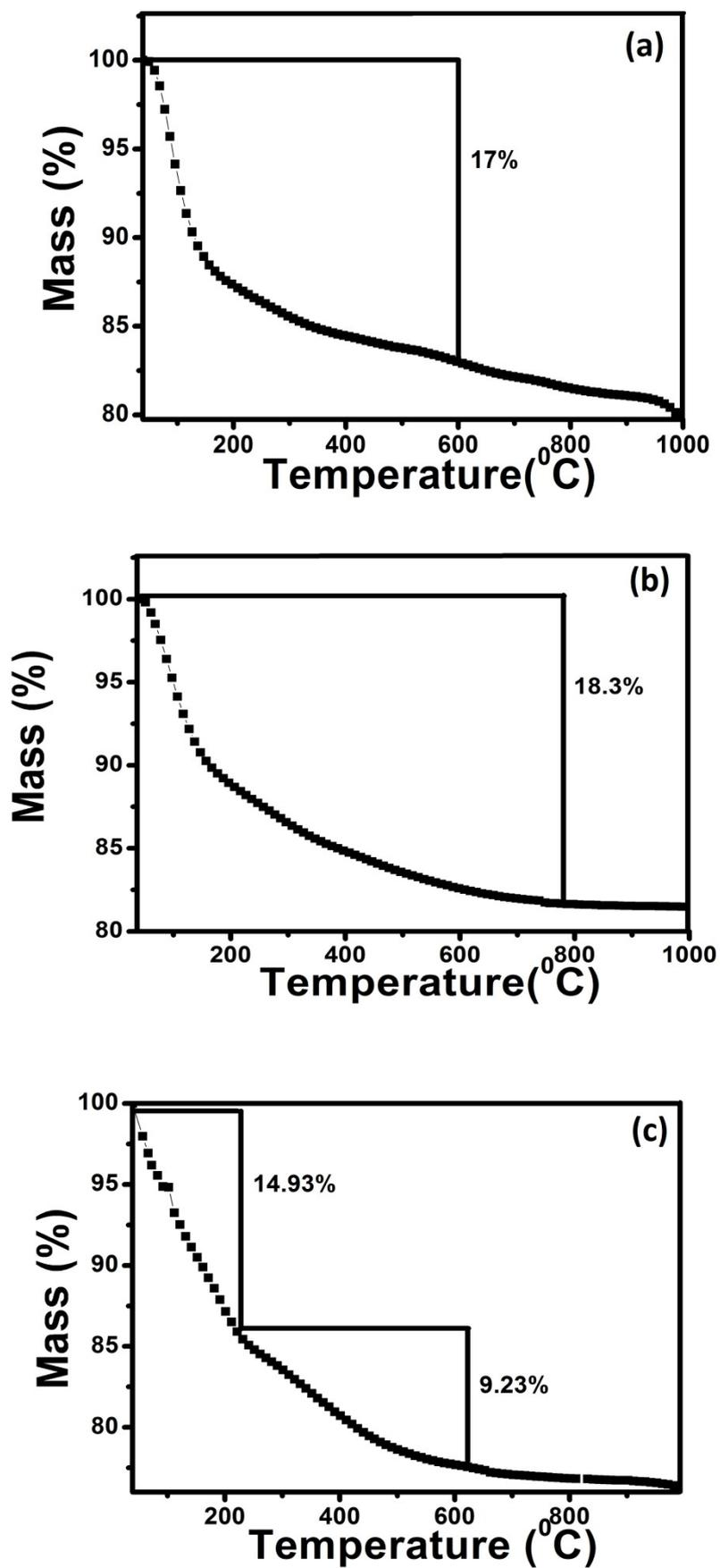
Fig S1: TGA plots of (a)  $\text{Sn}_{0.936}\text{O}_2$  (b)  $\text{Sn}_{0.957}\text{Sb}_{0.043}\text{O}_2$  and (c)  $\text{Sn}_{0.856}\text{Sb}_{0.144}\text{O}_2$  respectively
