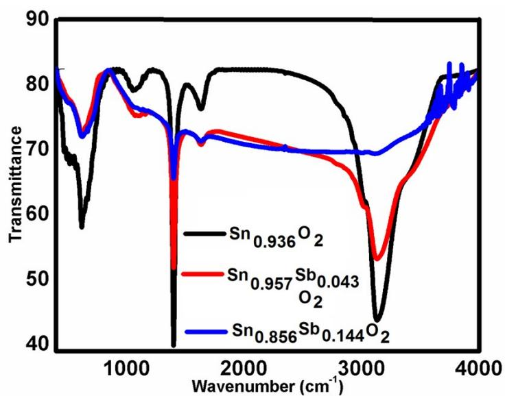
Fig S5: FTIR spectra of (a)  $\text{Sn}_{0.936}\text{O}_2$  (b)  $\text{Sn}_{0.957}\text{Sb}_{0.043}\text{O}_2$  and (c)  $\text{Sn}_{0.856}\text{Sb}_{0.144}\text{O}_2$  respectively.
