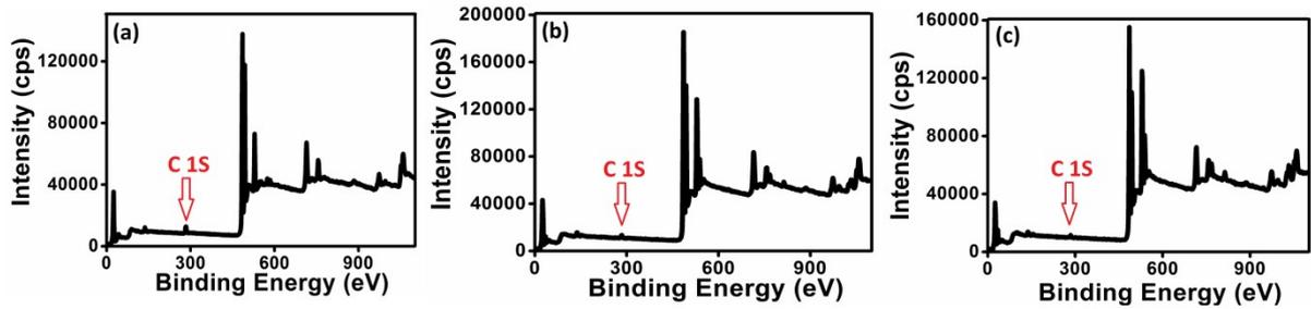
Fig S3: XPS survey scan of (a) Sn<sub>0.936</sub>O<sub>2</sub> (b) Sn<sub>0.957</sub>Sb<sub>0.043</sub>O<sub>2</sub> and (c) Sn<sub>0.856</sub>Sb<sub>0.144</sub>O<sub>2</sub>.
