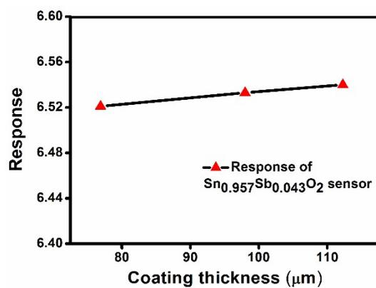
Fig S10: Plot of sensing response to 2 ppm SO<sub>2</sub> at room temperature vs. variation in sensor coating thickness for Sn<sub>0.957</sub>Sb<sub>0.043</sub>O<sub>2</sub> sample. Over a range of 70-120 μm, the response change is negligible.
