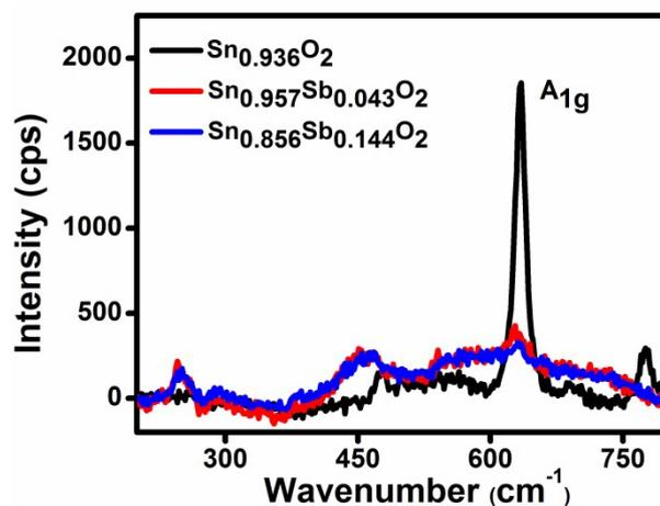
Fig S9: Room temperature Raman spectra of pure and antimony doped tin oxide samples. The shifting of  $A_{1g}$  vibration mode (indicative of tin vibrations) towards lower wave number region in doped samples indicates doping of  $\text{Sn}^{4+}$  by a species of larger ionic radius like  $\text{Sb}^{3+}$  and elongation of Sn-O bond in doped samples.
