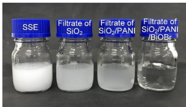
**Fig. S12.** Surfactant-stabilized soybean oil-in-water emulsion (SSE) before and after separation by different membranes.
