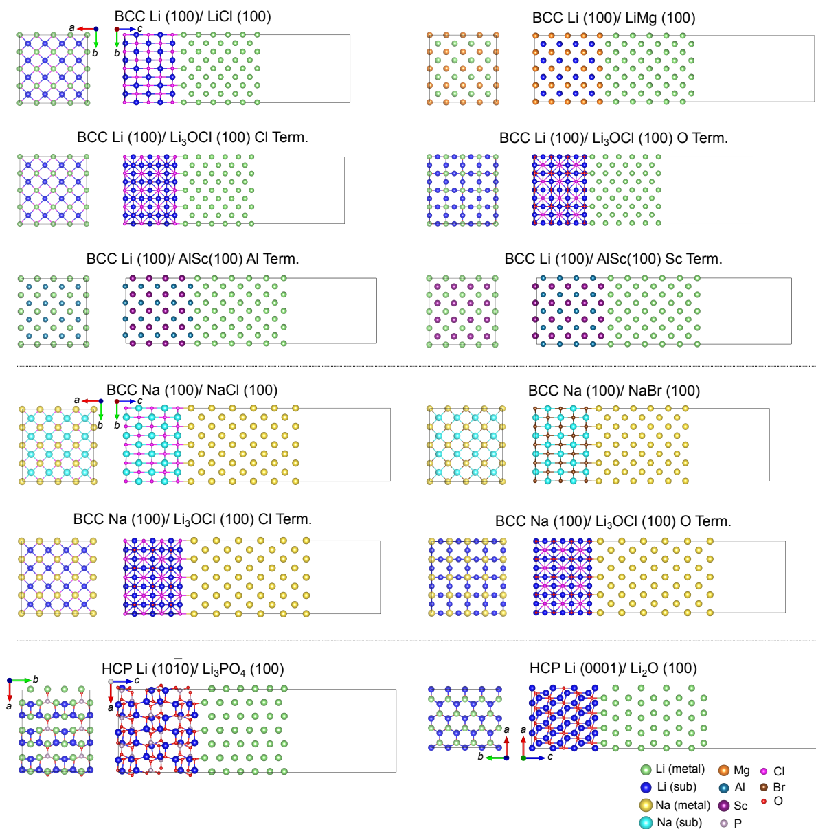
Fig. S2: DFT relaxed alkali metal/solid-state electrolyte interface structures. For all structures, a strain was applied to the body centred cubic (BCC) or hexagonal close packed (HCP) alkali metal (Li or Na) slab to match the lattice parameters of the substrate phase. Different colouring is used for the Li/Na atoms in the alkali metal unit cells and substrate phases to distinguish them.
