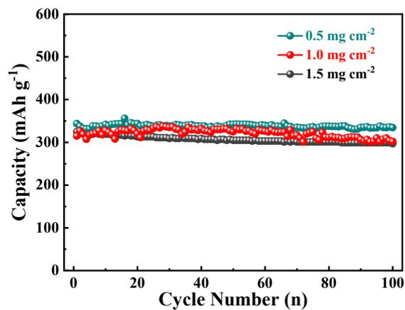
**Fig. S6** Comparative cycling performance of the  $\text{CoSe}_2\text{-CNS}$  electrode at  $10 \text{ A g}^{-1}$  with different mass loadings (the cells were initially activated at  $0.2 \text{ A g}^{-1}$  for 20 cycles).
