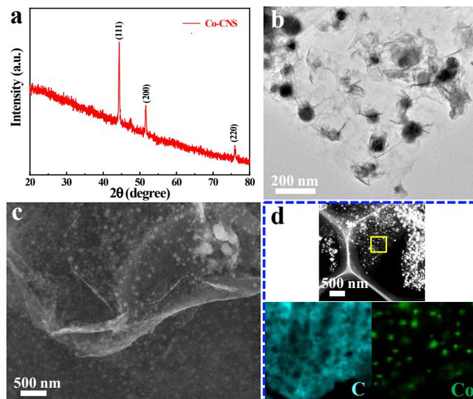
**Fig. S1** The microstructure and morphology of Co-CNS. (a) XRD pattern; (b) TEM image; (c) SEM image, (d) HAADF-STEM image and the EDX mappings.
