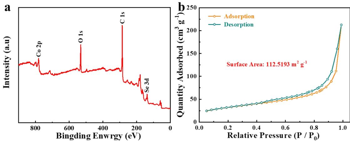
**Fig. S3** (a) The XPS survey spectrum and (b) N<sub>2</sub> adsorption/desorption isotherms of CoSe<sub>2</sub>-CNS.
