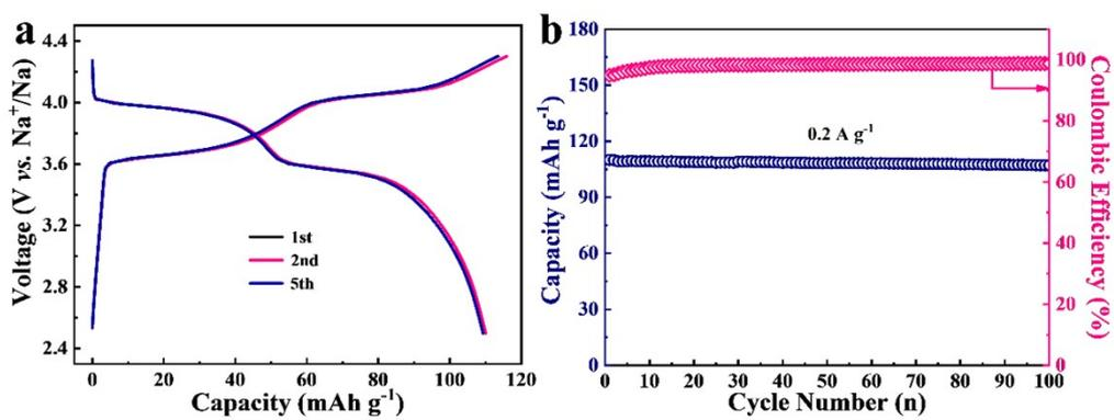
**Fig. S10** The cycle performance at  $0.2\ \text{A g}^{-1}$  of NVPOF cathode.
