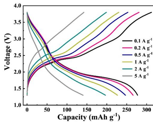
**Fig. S11** The GCD curves of CoSe<sub>2</sub>-CNS/NVPOF full cell at different current densities.
