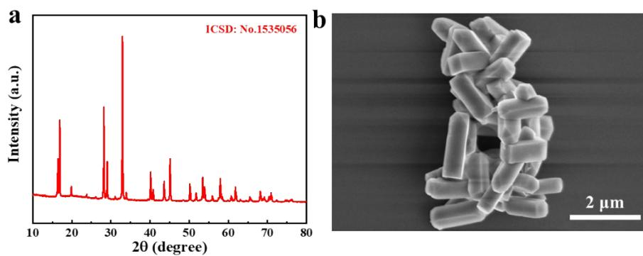
**Fig. S9** (a) XRD and (b) SEM image of the NVPOF.
