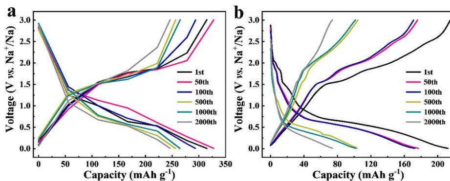
**Fig. S5** The GCD curves at  $10 \text{ A g}^{-1}$  of (a)  $\text{CoSe}_2\text{-CNS}$  and (b) pure  $\text{CoSe}_2$ .
