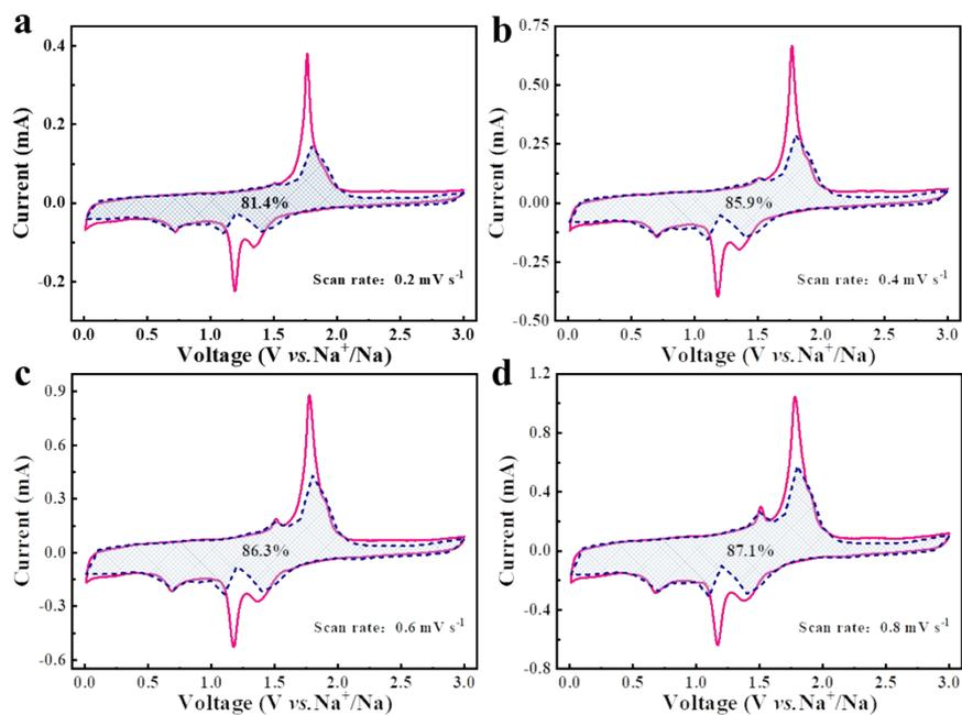
**Fig. S7** Separation of the capacitive (shaded region) and diffusion currents at different scan rates.
