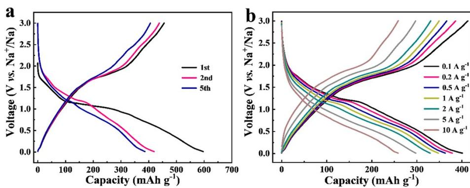
**Fig. S4** (a) The GCD curves at 0.2 A g<sup>-1</sup> and (b) rate capacities at current densities of pure CoSe<sub>2</sub>.
