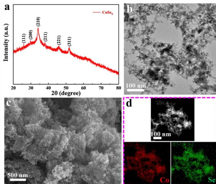
**Fig. S2** The microstructure and morphology of pure  $\text{CoSe}_2$ . (a) XRD pattern; (b) TEM image; (c) SEM image, (d) HAADF-STEM image and the EDX mappings.
