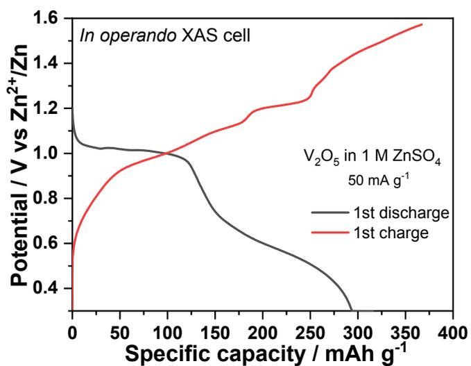
**Figure S5** Discharge-charge profiles of  $V_2O_5$  in 1 M  $ZnSO_4$  electrolyte for *in operando* XAS (50 mA  $g^{-1}$ )
