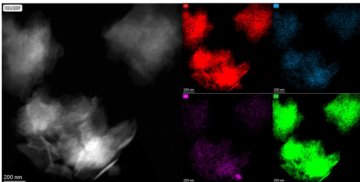
**Figure S6** STEM-HAADF EDX mapping of O (red), S (blue), V (magenta), and Zn (green) for the 1<sup>st</sup> discharged  $V_2O_5$
