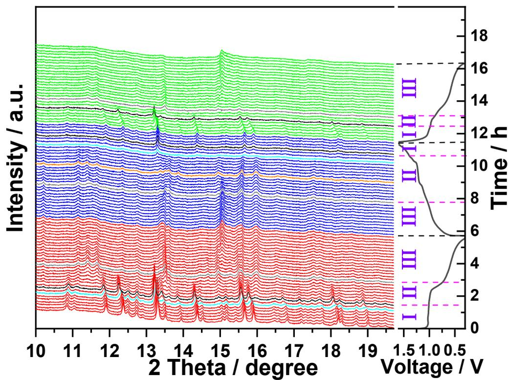
**Figure S3** *In operando* synchrotron diffraction of  $V_2O_5$  during the first one and half cycles and the corresponding voltage profile at a current density of  $50 \text{ mA g}^{-1}$
