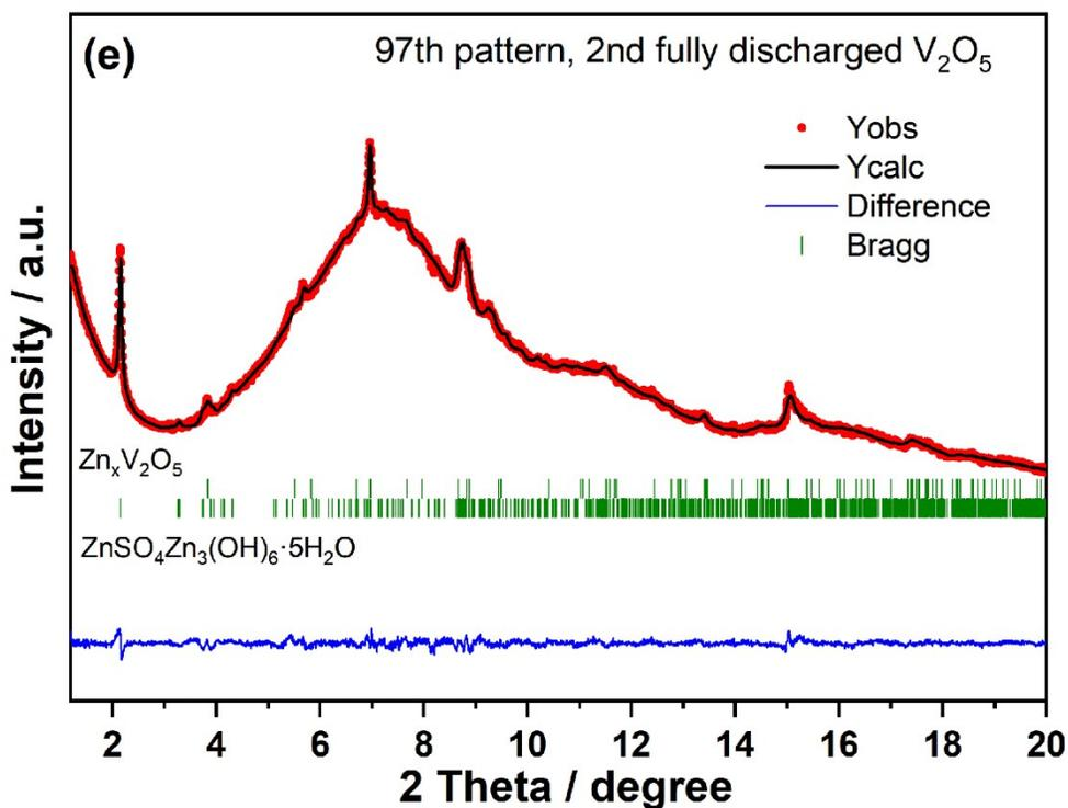
**Figure S2** Rietveld refinement based on the pattern of the pristine  $V_2O_5$  (a), discharged state in the beginning of Region II with the capacity of  $44 \text{ mAh g}^{-1}$  ( $10^{\text{th}}$  pattern, 1.02 V) (b), first fully discharged  $V_2O_5$  electrode at 0.3 V ( $36^{\text{th}}$  pattern) (c), fully charged at 1.6 V ( $69^{\text{th}}$  pattern) (d), and 2<sup>nd</sup> fully discharged  $V_2O_5$  electrode at 0.3 V ( $97^{\text{th}}$  pattern) (e)
