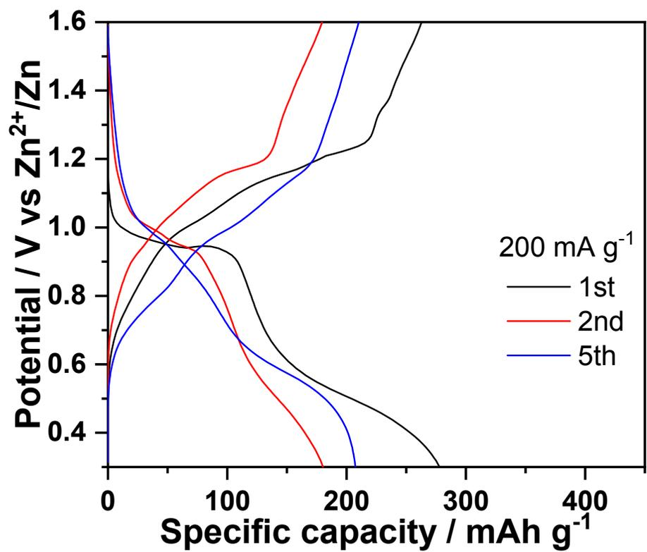
Figure S1 Discharge-charge profiles of  $V_2O_5$  nanowires at  $200 \text{ mA g}^{-1}$  in  $1 \text{ M ZnSO}_4$
