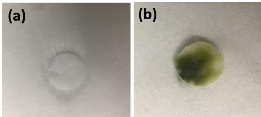
**Figure S4** Images of separator from the 1<sup>st</sup> discharged  $V_2O_5$  at 0.3 V (a) and the 1<sup>st</sup> charged  $V_2O_5$  at 1.6 V (b)
