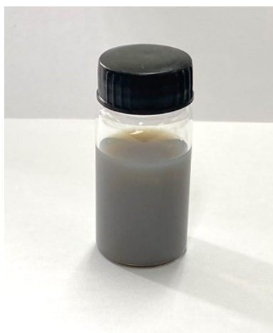
Figure S5. Optical image of the final ND dispersion with the concentration of 2 mg mL -1 .
