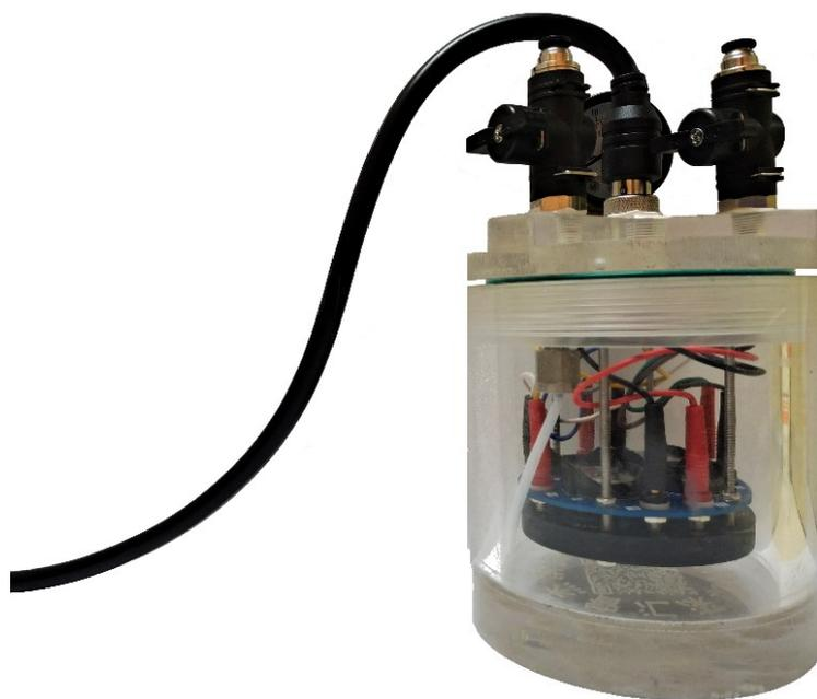
**Fig. S6** The image of the hermetic container for Li-O<sub>2</sub> batteries purchased from NJ Scientific Ltd.
