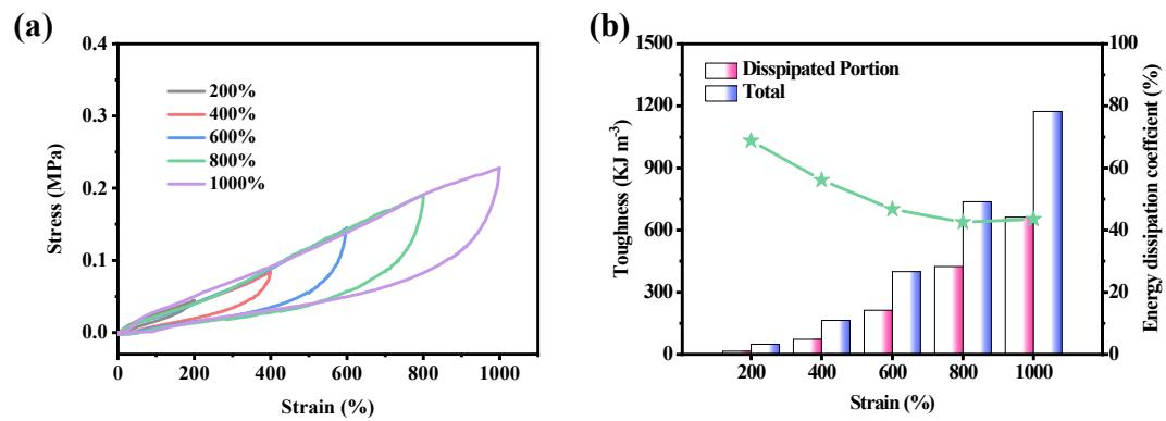
**Figure S6.** Mechanical properties of PPDC hydrogel (a) Loading-unloading curves and (b) corresponding toughness/energy dissipation at different maximum strain.
