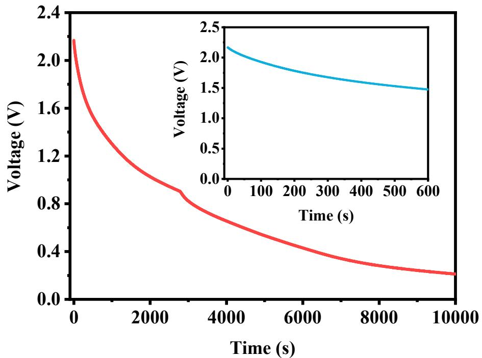
**Figure S16.** The self-discharge profile of the hydrogel supercapacitor.
