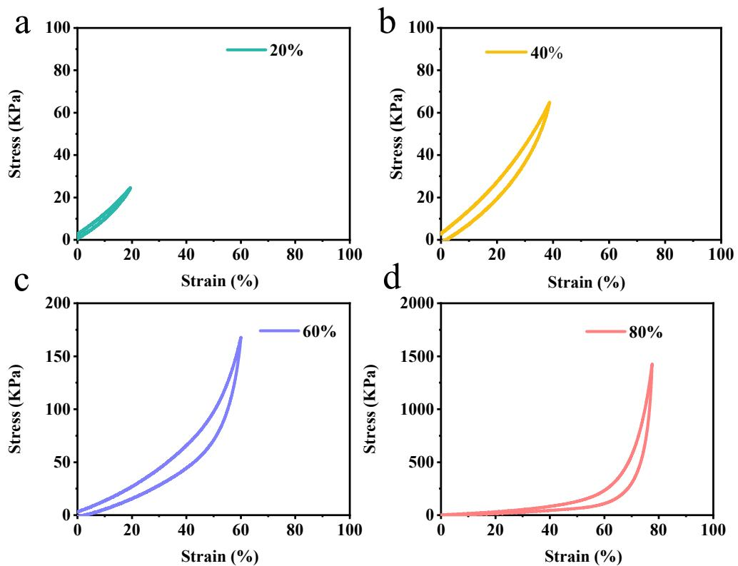
**Figure S3.** Compression-recovery measurements of the PPDC hydrogel at different strain, (a) 20%, (b) 40%, (c) 60% and (d) 80%.
