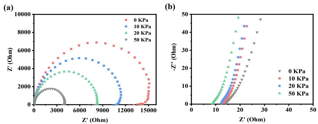
**Figure S15.** Nyquist impedance plots of the supercapacitor at devise compression
