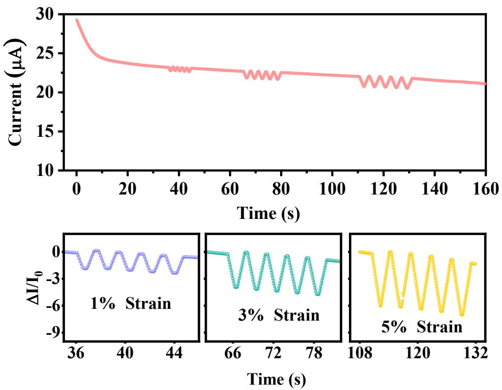
**Figure S20.** Tiny strain response upon loading and unloading strain of 1%, 3% and 5%.
