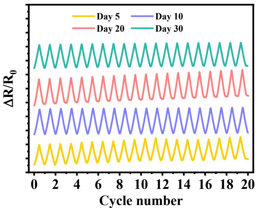
**Figure S19.** Long-term operation at 50% strain of the PPDC hydrogel sensor over 30 day in ambient condition without specific encapsulation
