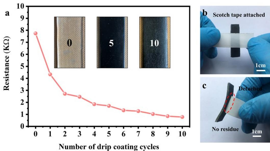
**Figure S11.** (a) The relationship between the surface resistance of supercapacitor and the number of drop coating cycles. (b) and (c) adhesion strength test. scotch tape attached to the surface of supercapacitor and detached respectively.
