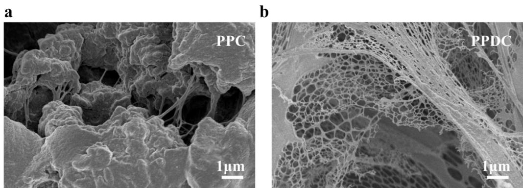
**Figure S5.** SEM images of (a) PPC hydrogel and (b) PPDC hydrogel.
