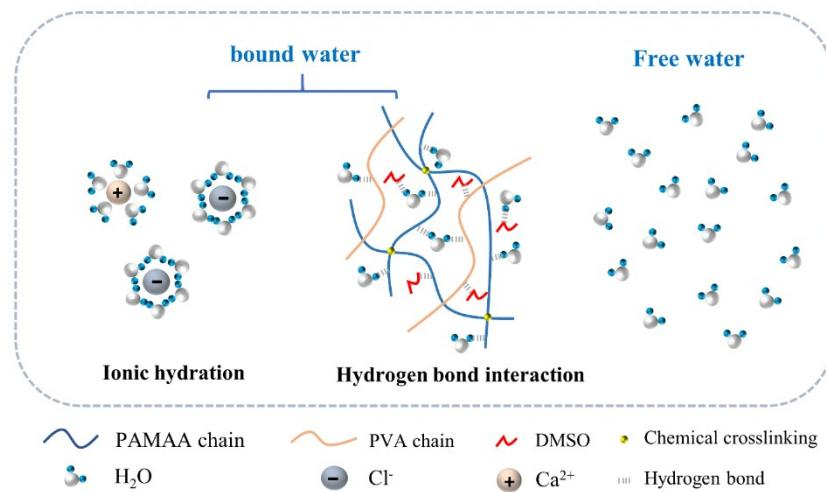
**Figure S10.** Schematic of the hydration of  $\text{CaCl}_2$  in water and the hydrogen bond interaction among the  $\text{H}_2\text{O}$ , DMSO and the PVA/PAMAA chains.
