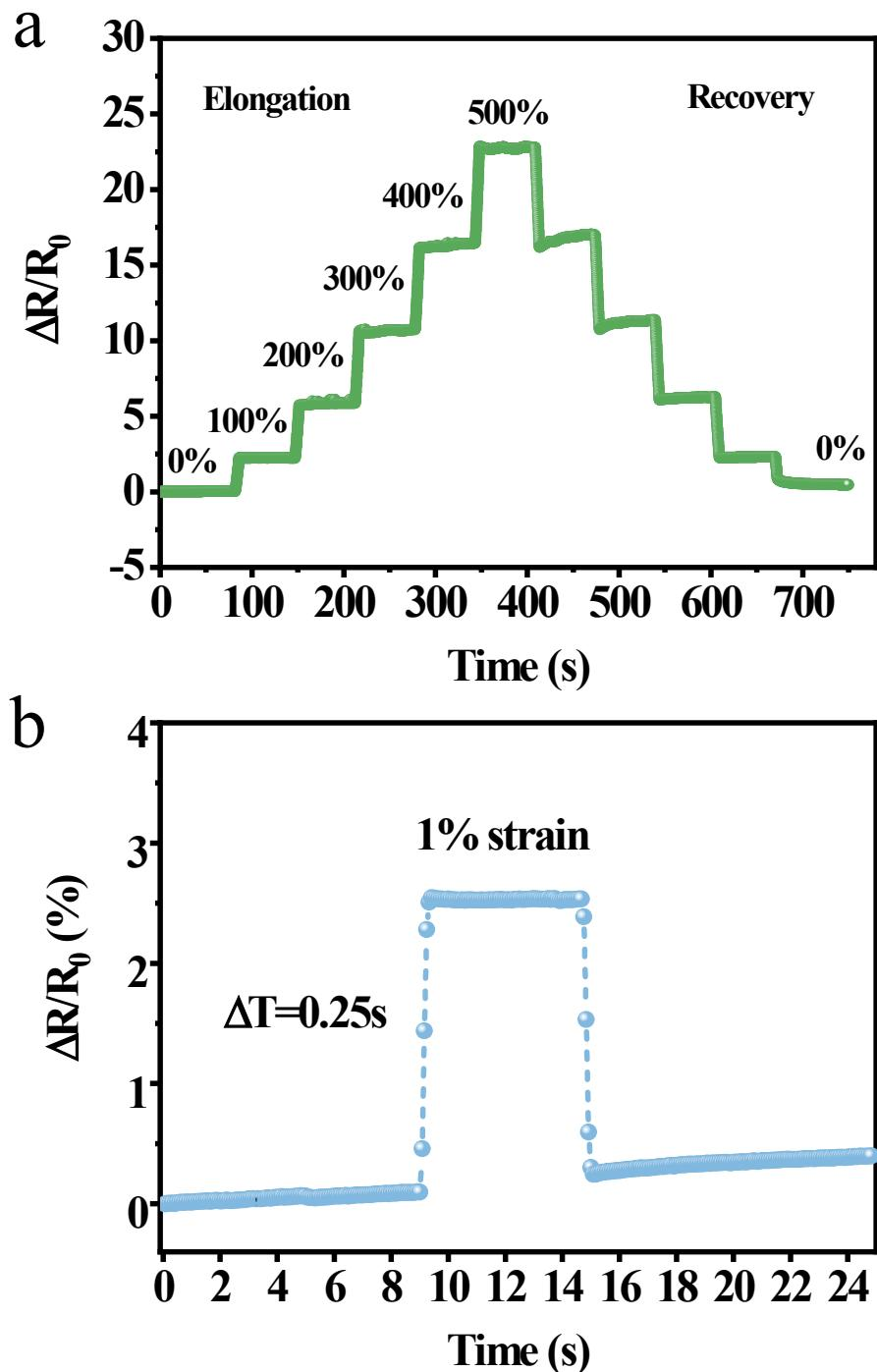
**Figure S18.** (a) Resistance response of the hydrogel strain sensor stretched to 100%, 200%, 300%, 400% and 500%. (b) The resistance response of the hydrogel strain sensor upon loading and unloading a strain of 1%.
