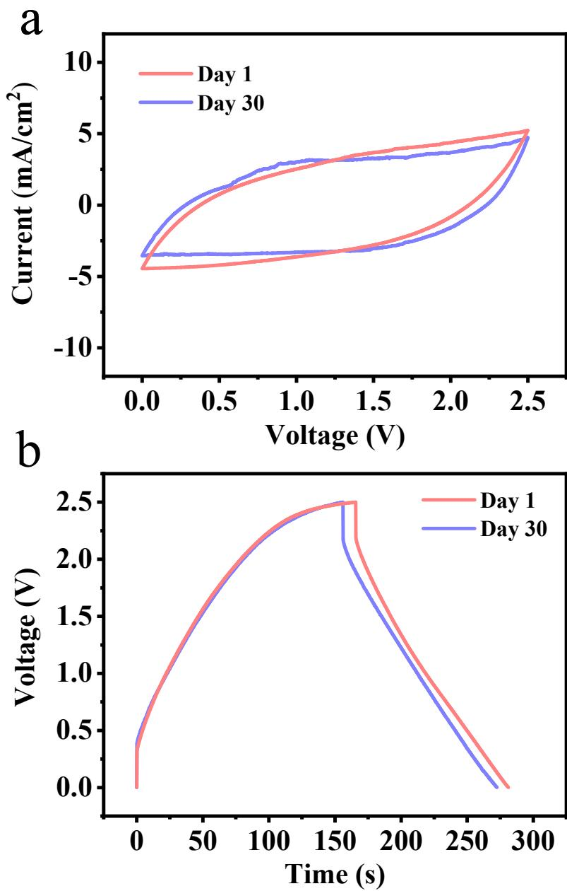
**Figure S13.** (a) The CV curves and (b) The GCD curves of the supercapacitor compared with storage after 1 day and 30 days.
