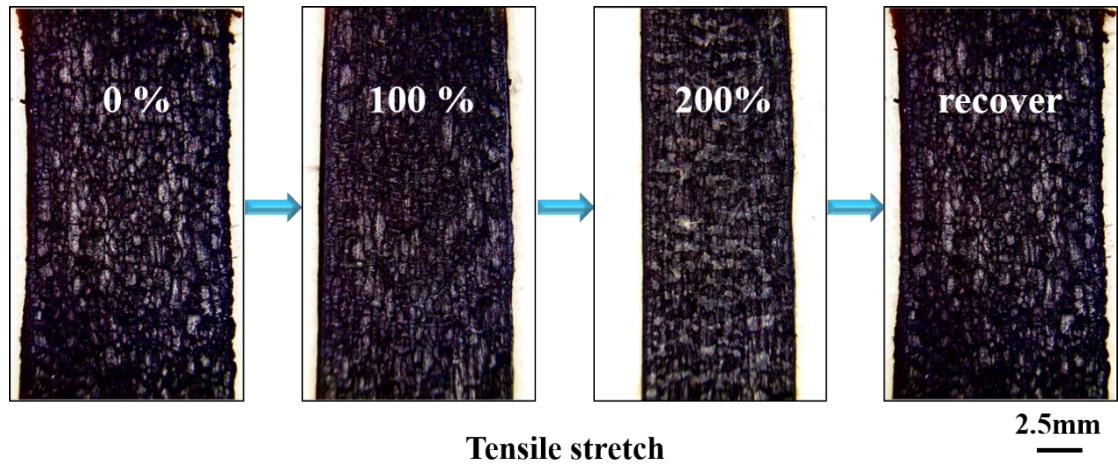
**Figure S14.** Images of a typical supercapacitor when stretched from 0% to 200% strain, and relaxation after unloading.
