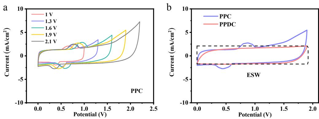
**Figure S12.** (a) CV curves of the PPChydrogel with different work voltage at 50 mV s<sup>-1</sup> (b) The Electrochemical stability windows for (ESW) for PPC and PPDC hydrogels.
