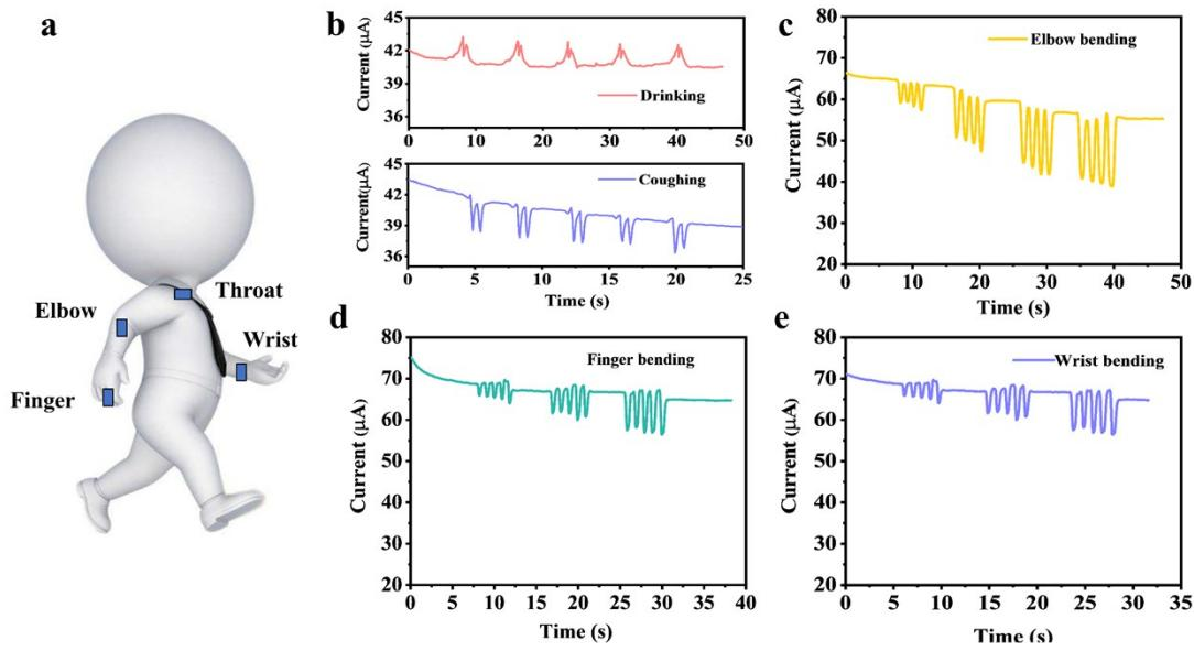
**Figure S21.** Digital images and corresponding time-current response curves of the self-powered integrated sensing systems in human motion detection. (a) Test schematic, (b) drinking and coughing, (c) elbow bending, (d) finger bending, (e) wrist bending.
