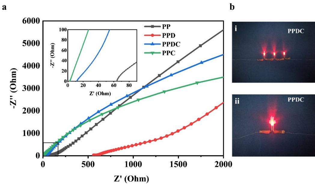
**Figure S17.** (a)Nyquist impedance plots of the PVA/PAMAA based hydrogel (b) the electrical properties illustration of hydrogel.
