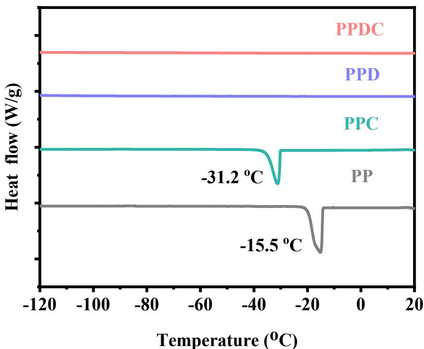
**Figure S9.** The DSC curves of the PP, PPC, PPD and PPDC hydrogel ranging from -120 °C to 20 °C.
