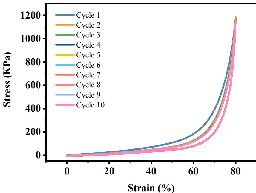
**Figure S4.** Ten successive cyclic loading-unloading curves of the PPDC hydrogel without a resting interval between two consecutive tests.
