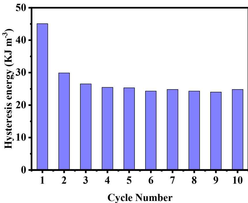
**Figure S7.** The dissipated energies of ten successive loading-unloading cycles at tensile strain of 300%.
