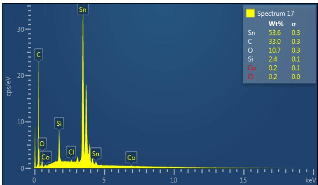
**Figure S21.** EDS analysis of SWCNHs-2 onto FTO.
