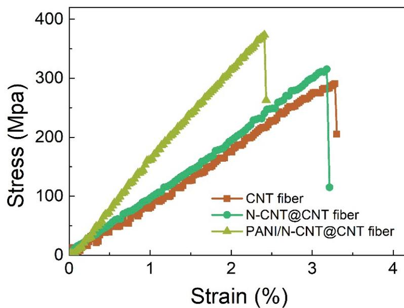
**Figure S5.** Typical tensile stress-strain curves for CNT fiber, N-CNT@CNT fiber and PANI/N-CNT@CNT fiber, respectively.
