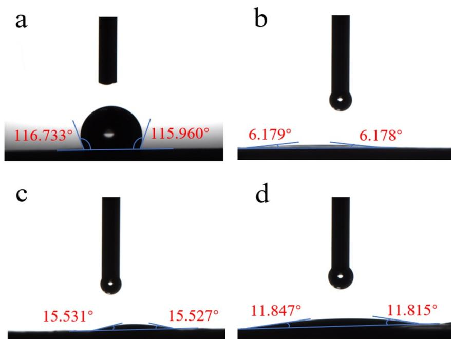
**Figure S3.** Static water contact angles on sheet electrodes with the same material structure of corresponding fiber electrodes. (a) CNT, (b) N-CNT@CNT, (c) PANI@CNT and (d) PANI/N-CNT@CNT.
