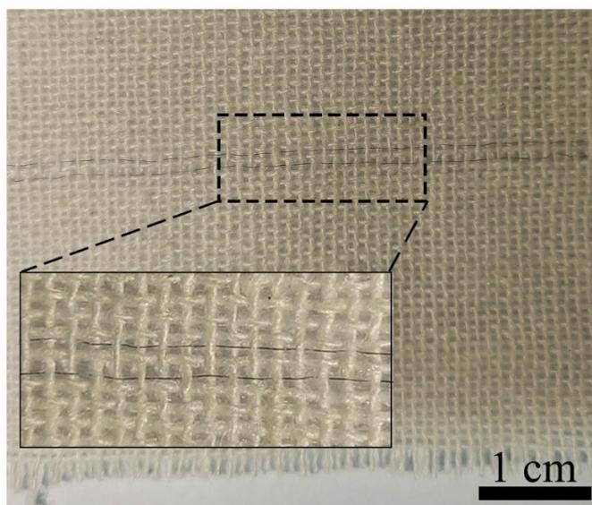
**Figure S13.** The picture of the hierarchical core-sheath fiber based supercapacitors woven into a textile.
