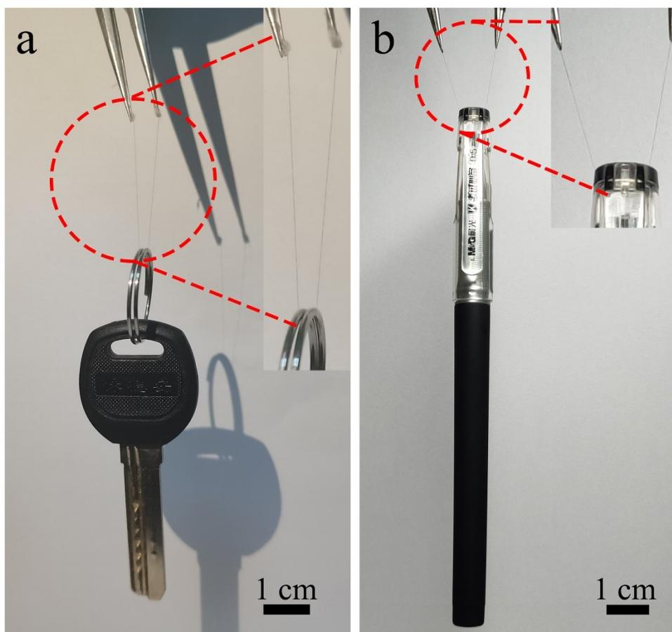
**Figure S4.** Optical images of N-CNT@CNT fiber lifting weights of a (a) key and (b) pen.
