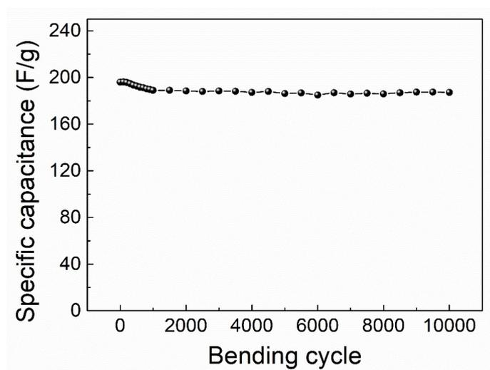
**Figure S15.** FSC capacitance values after different bending cycles of 0°-to-180°-to-0°.
