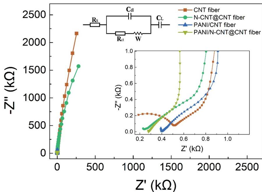
**Figure S9.** Nyquist plots of fiber electrodes with different structures. The insets are the Nyquist plots in the high-frequency region and the Equivalent circuit to fit the EIS data.<sup>60, S4</sup> The equivalent values of  $R_s$  and  $R_{ct}$  were summarized in Table S2.  $R_s$ ,  $R_{ct}$ ,  $W$ ,  $C_{dl}$  and  $C_L$  stand for the series resistance, charge transfer resistance, Warburg element, double-layer capacitance and pseudocapitance, respectively.
