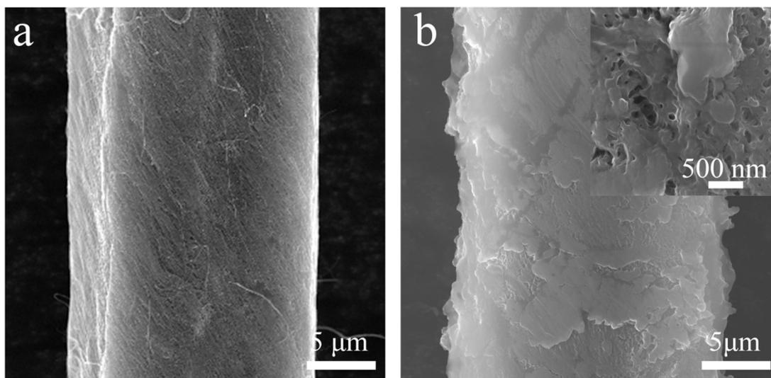
**Figure S8.** SEM images of (a) CNT fiber and (b) PANI@CNT fiber with 70% PANI, the inset in b is the magnified SEM image.
