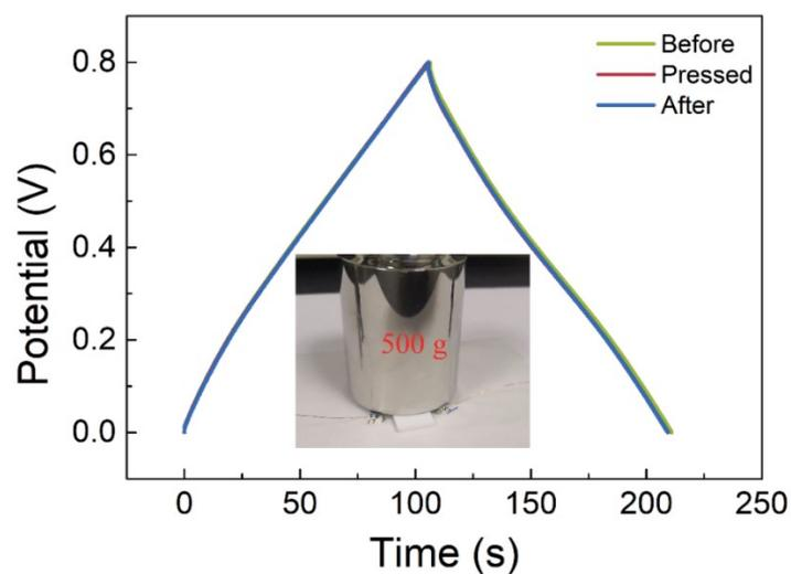
**Figure S16.** GCD profiles of the FCS before, during and after pressing process, and the inset is the
