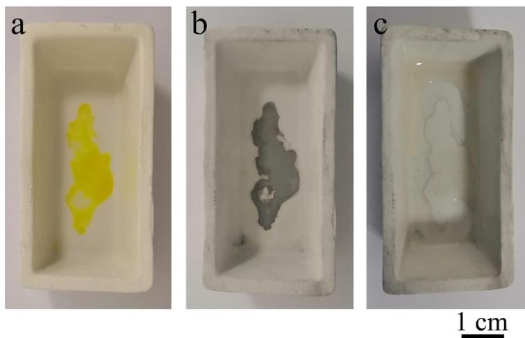
**Figure S1.** Ferric chloride (a) catalyst precursor solution, (b) reduced into iron during CVD process and (c) then dissolved in acid solution.
