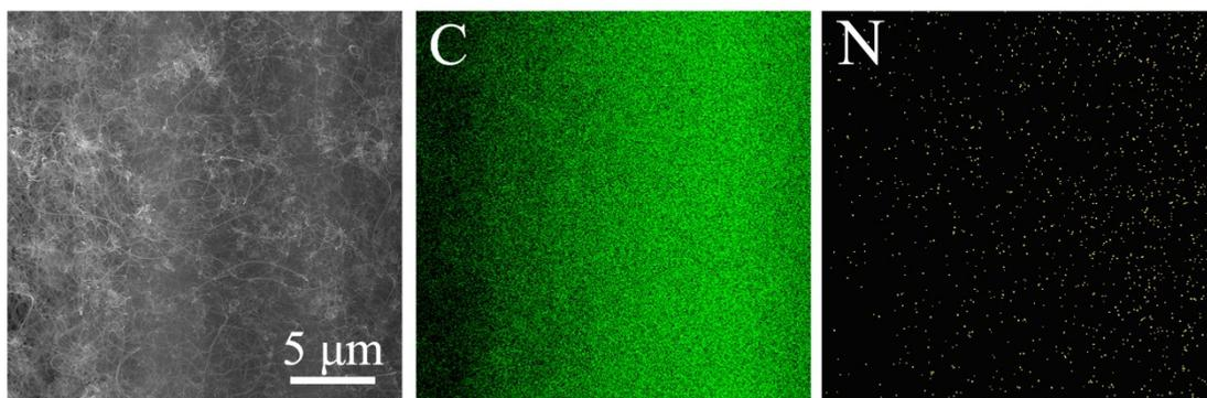
**Figure S2.** EDS mapping of N-CNT@CNT fiber composites.
