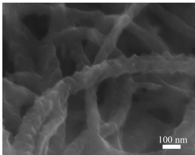
**Figure S6.** Magnified SEM image of PANI/N-CNT in PANI/N-CNT@CNT fiber.
