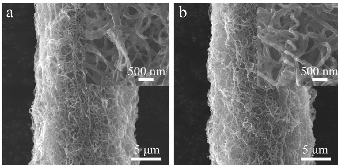
**Figure S12.** SEM images of PANI/N-CNT@CNT fiber electrode (a) before and (b) after 1000 cycles of GCD processes under  $10 \text{ A g}^{-1}$ , the insets are the corresponding SEM image under higher magnification.
