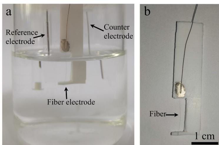
**Figure S7.** The optical photos of (a) fiber electrode in three-electrode system, (b) fiber electrode fixed on a plastic holder.
