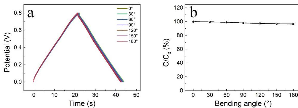
**Figure S11.** Electrochemical characterization of PANI/N-CNT@CNT fiber electrode under different bending angles. (a) GCD profiles of fiber electrode bending at different angles. (b) Capacitance retention of fiber electrode under different bending angles.
