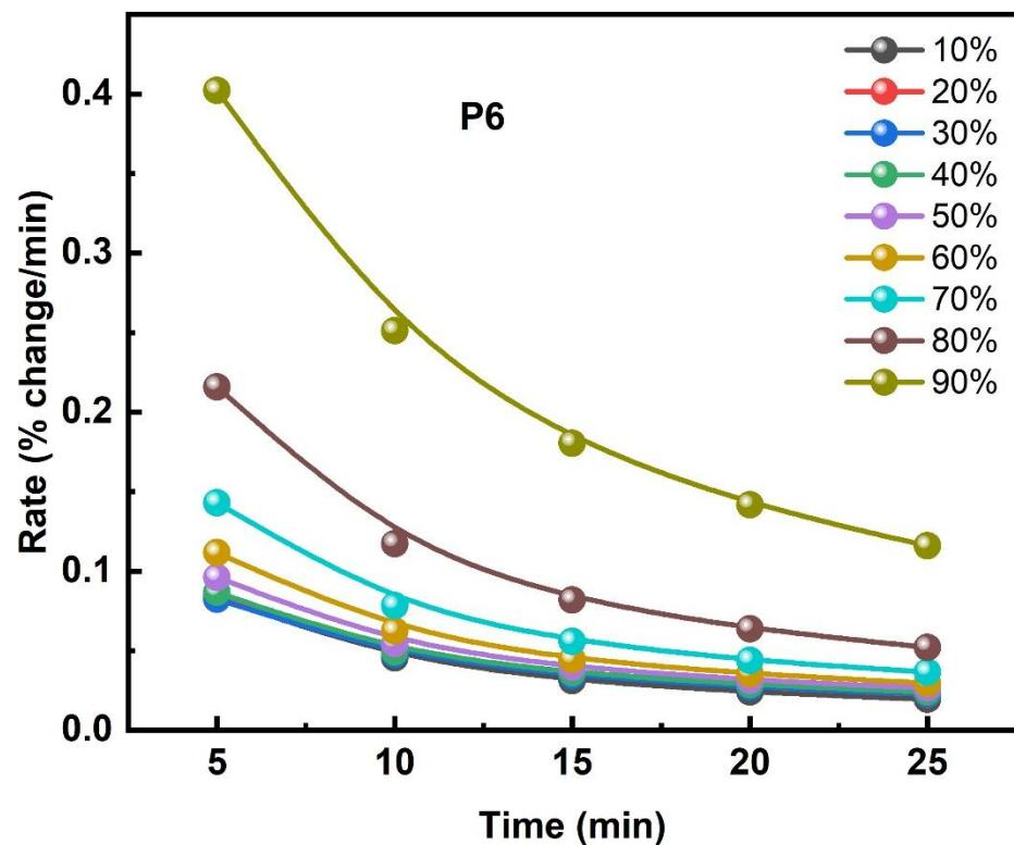
**Figure S10.** Water uptake rate of P6 at different relative humidity ranges from 10 to 90%.
