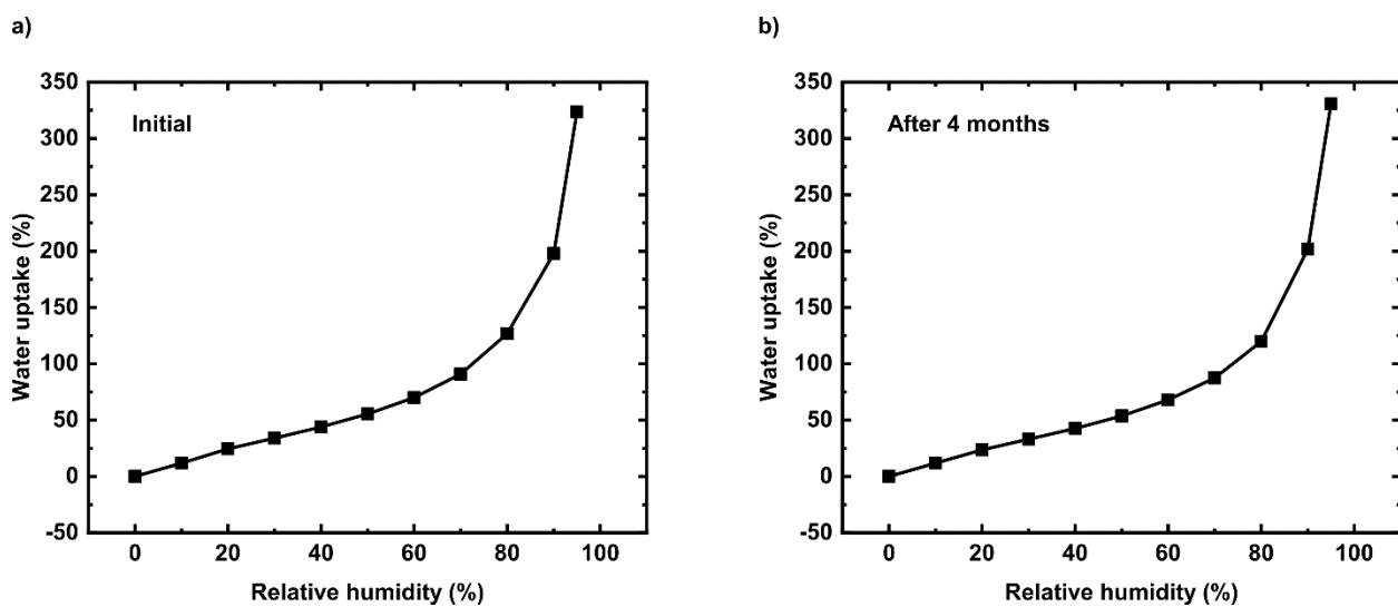
**Figure S13.** The water uptake versus relative humidity of P4 tested (a) initially, and (b) after 4 months. The polymer was stored under wet conditions during the 4 months.
