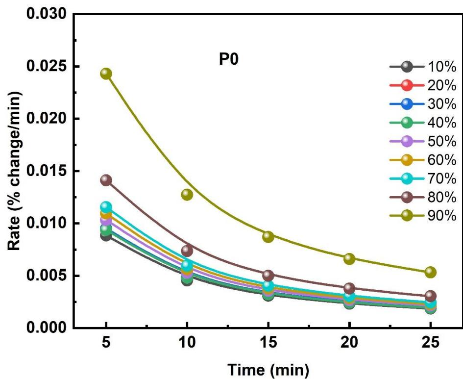
**Figure S4.** Water uptake rate of P0 at different relative humidity ranges from 10 to 90%.
