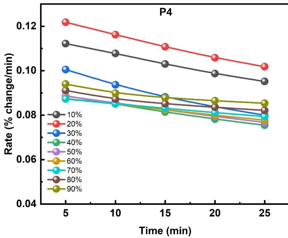
**Figure S8.** Water uptake rate of P4 at different relative humidity ranges from 10 to 90%.
