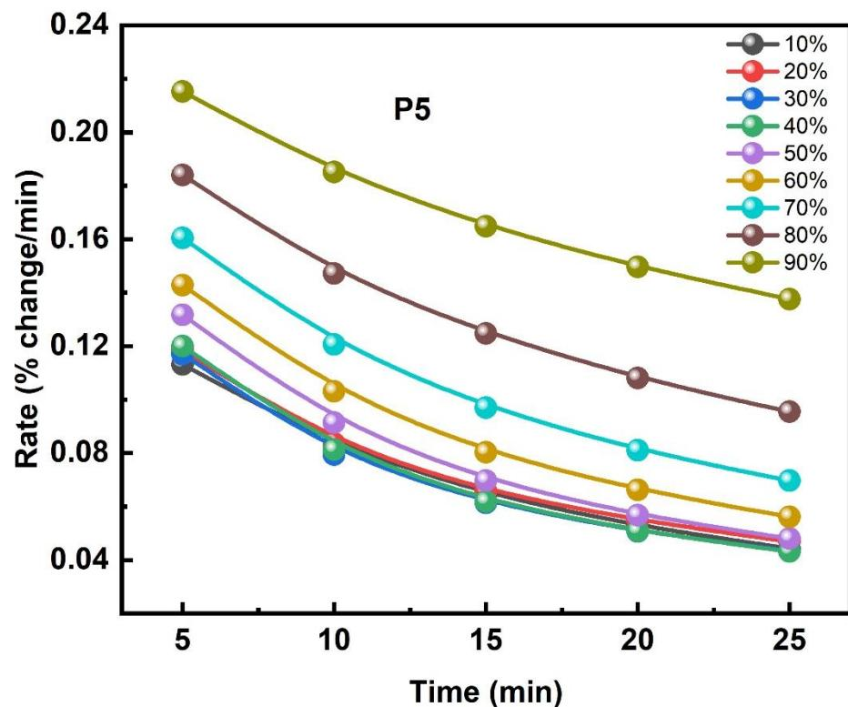
**Figure S9.** Water uptake rate of P5 at different relative humidity ranges from 10 to 90%.
