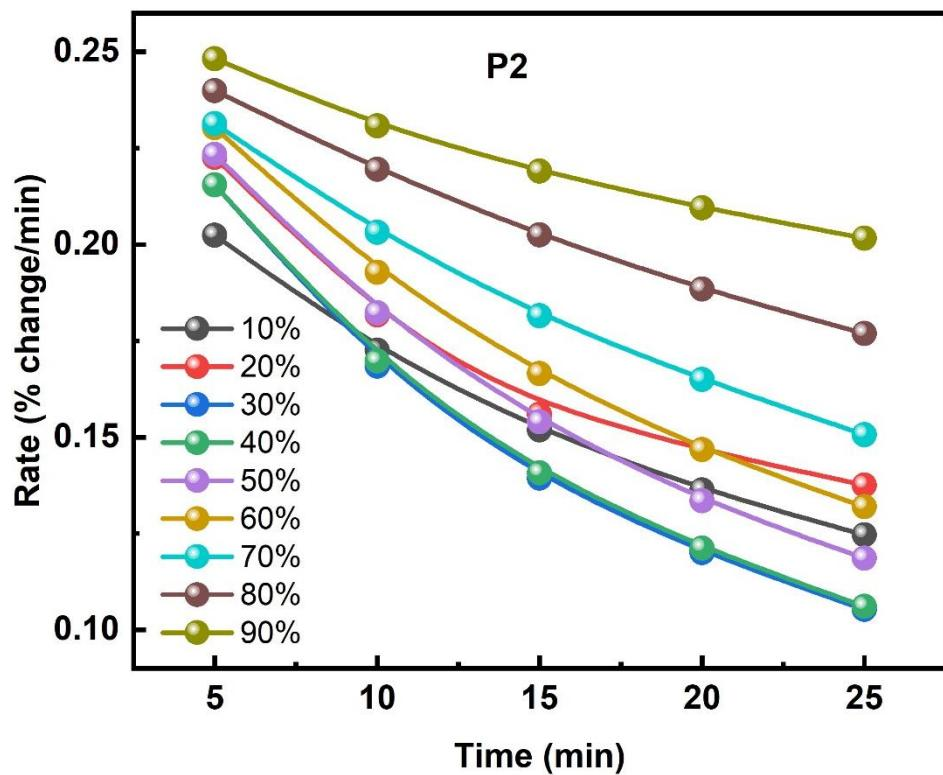
**Figure S6.** Water uptake rate of P2 at different relative humidity ranges from 10 to 90%.
