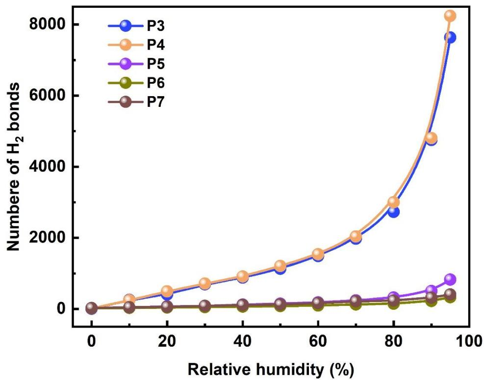
**Figure S3.** Hydrogen bond interactions of the SPEEK polymers as a function of RH.
