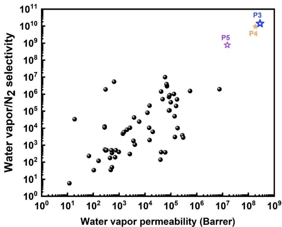
**Figure S12.** Performance of the theoretical membranes and comparison with the state-of-the art membranes for water vapor permeability and selectivity.
