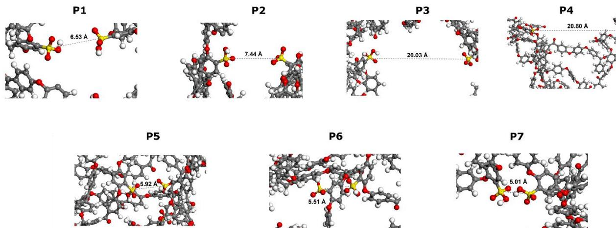
**Fig. S2.** Calculated S-S distances between SO<sub>3</sub>H groups in the SPEEK polymer matrix.
