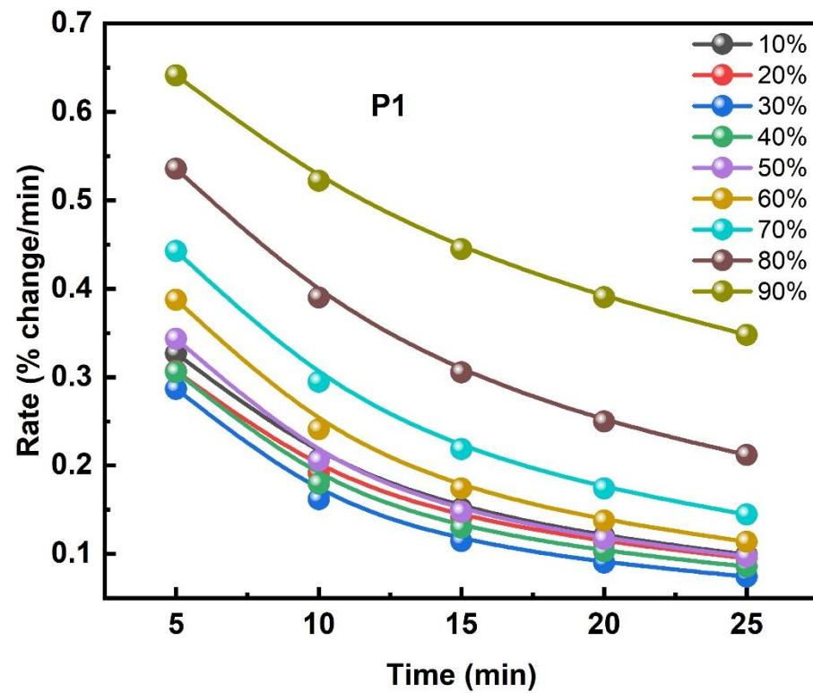
**Figure S5.** Water uptake rate of P1 at different relative humidity ranges from 10 to 90%.
