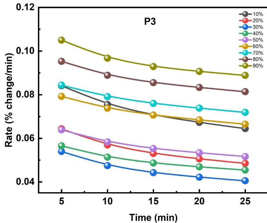
**Figure S7.** Water uptake rate of P3 at different relative humidity ranges from 10 to 90%.
