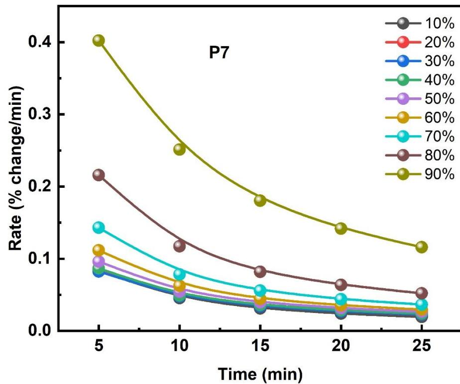
**Figure S11.** Water uptake rate of P7 at different relative humidity ranges from 10 to 90%.
