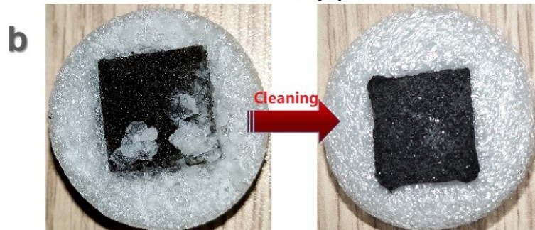
Figure S15. (a) The rate of evaporation before and after the evaporator is washed. (b) surface solid accumulation after the seawater evaporation and the evaporator after the salt removal by hand washing.
