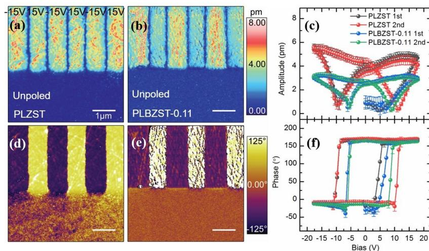
Figure S1. The PFM amplitude and phase of unpoled PLZST and PLBZST-0.11 ceramics.
