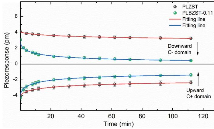
Figure S2. The relaxation process of the piezoresponse of PLZST and PLBZST-0.11 samples.
