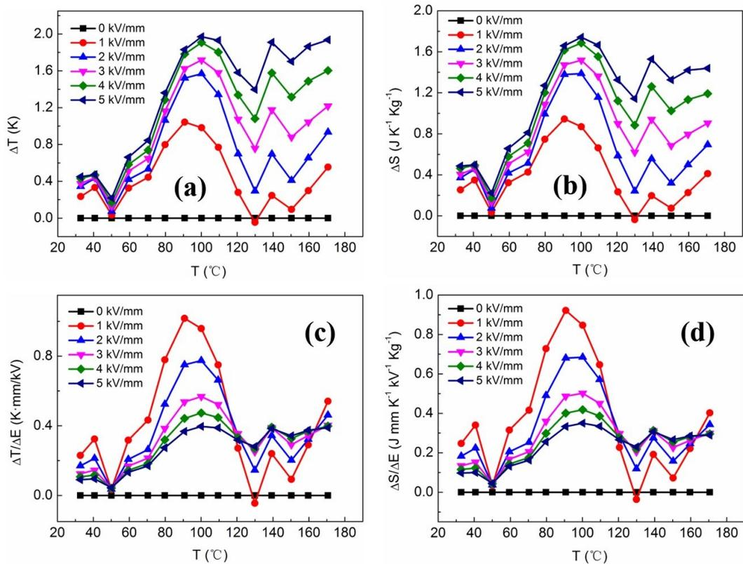
Figure S6. Temperature dependent evolution of (a)  $\Delta T$  and (b)  $\Delta S$  of PLZST ceramics under different electric fields. The temperature dependent electrocaloric strength (c)  $\Delta T/\Delta E$  and (d)  $\Delta S/\Delta E$  of PLZST ceramics under various electric fields.
