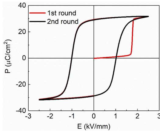
Figure S3. The P-E loops of PLZST ferroelectric ceramics at room temperature.
