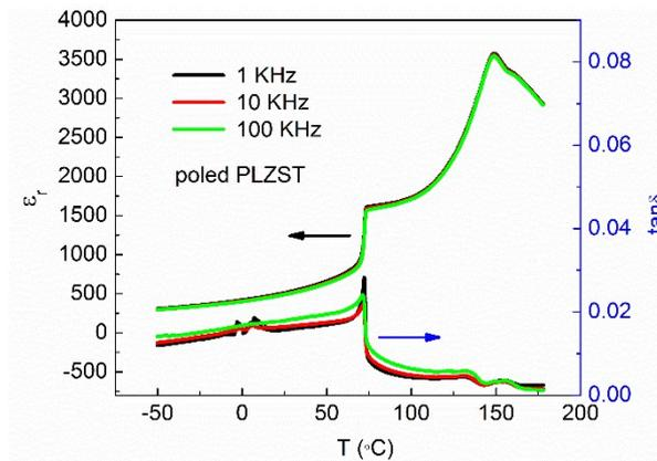
Figure S4. The temperature dependent dielectric constant and dielectric loss of poled PLZST ceramics.
