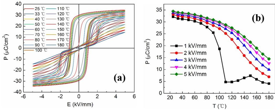
Figure S5. The temperature dependent P-E loops and polarization evolution of PLZST ferroelectric ceramics under different electric fields.
