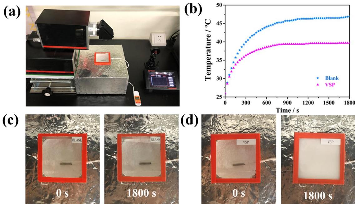
**Supplementary Fig. 6** (a) Photo of the solar simulator equipment. VSP and Blank were installed on the testing box, respectively. (b) The measured temperatures change curve with the irradiation time. (c-d) Optical photos for Blank and VSP at 20 °C and 60 °C, respectively.
