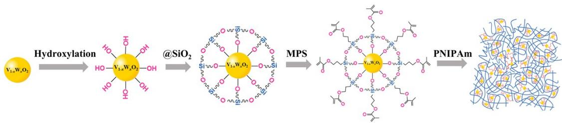
**Supplementary Fig. 1** Schematic illustration of the fabrication procedure of organic-inorganic nanocomposites.
