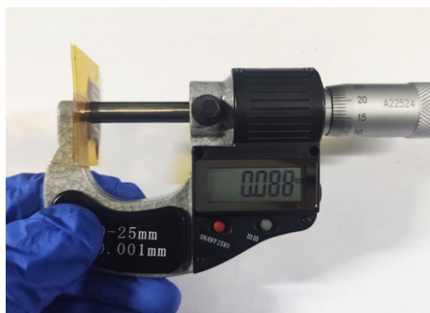
Fig. S24 The thickness of the as-prepared flexible \text{Na}_{0.55}\text{Mn}_2\text{O}_4/\text{VN}/\text{rGO} planar ASCs based on the current collector, active material, gel electrolyte, and Kapton tape was measured by vernier caliper.
