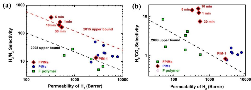
**Fig. S11.** Performance plot of (a)  $\text{H}_2/\text{N}_2$  and (b)  $\text{H}_2/\text{CO}_2$  for FPIMs (red), PIMs (blue) and fluorinated polymers (F polymers, green). The 2008 upper bounds for  $\text{H}_2/\text{N}_2$  and  $\text{H}_2/\text{CO}_2$  were from reference 4; the 2015  $\text{H}_2/\text{N}_2$  upper bound was from reference 5.
