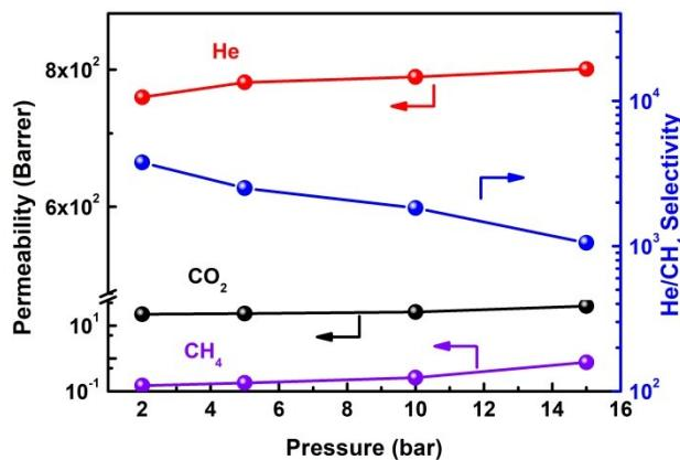
**Fig. S12.** Pressure dependent pure-gas permeability of the He, CH<sub>4</sub> and CO<sub>2</sub>, and the ideal He/CH<sub>4</sub> selectivity under different upstream pressures.
