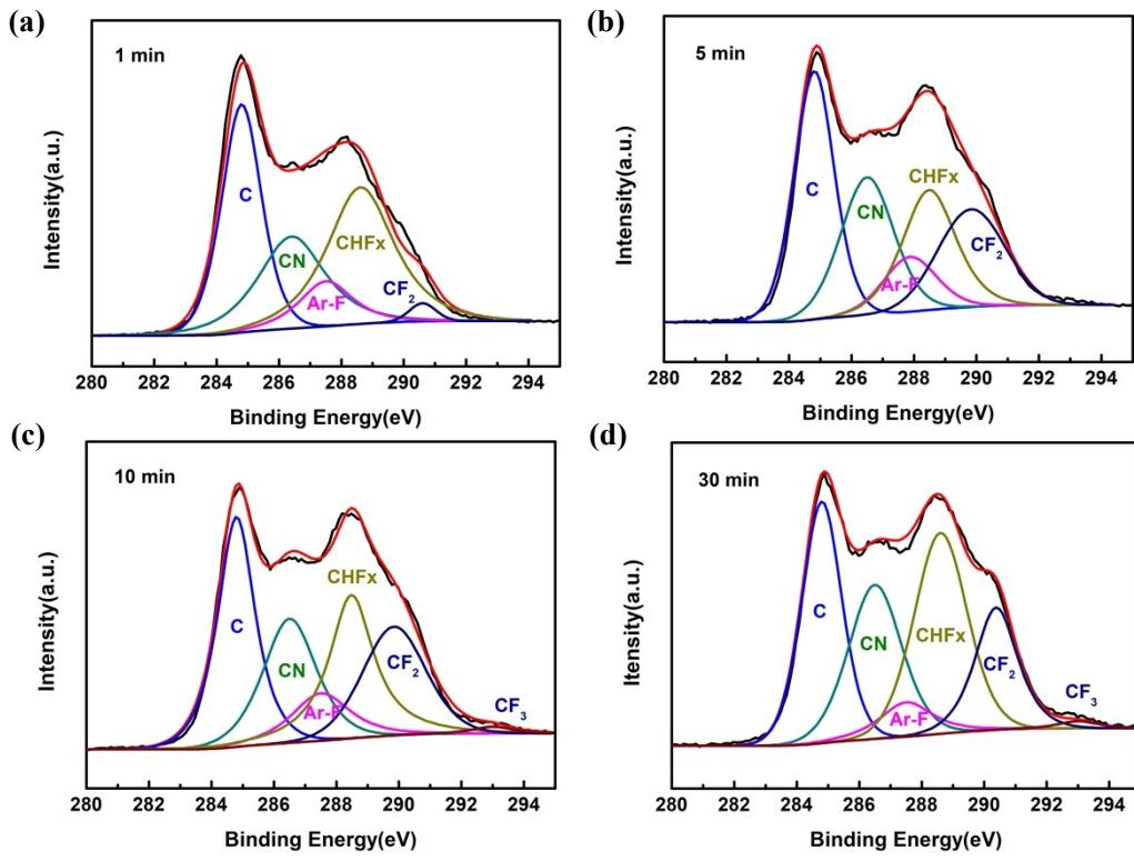
**Fig. S8.** XPS spectra of the C<sub>1s</sub> for PIM-1 membrane at different fluorination times: (a) 1 min, (b) 5 min, (c) 10 min, (d) 30 min. The signals of 284.8 (C), 286.4 (CN), 287.5 (Ar-F), 288.6 (CHFx), 290.6 (CF<sub>2</sub>), and 293 (CF<sub>3</sub>) eV were deconvoluted.
