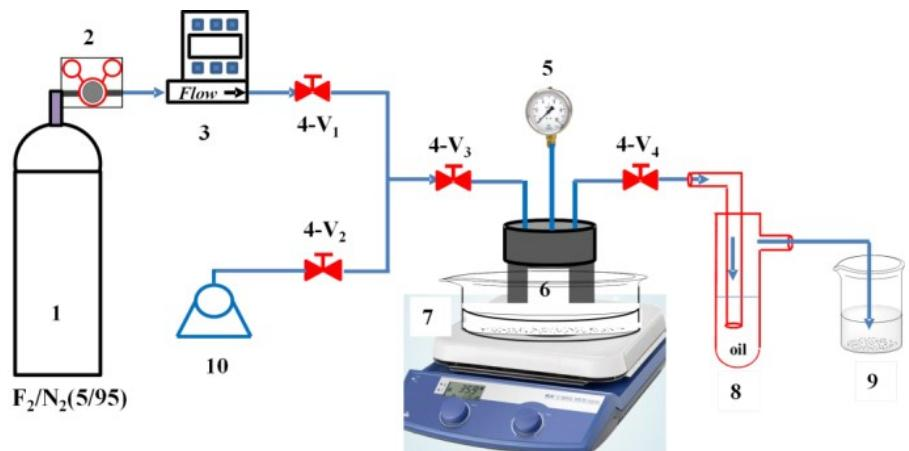
**Fig. S1.** Set-up for direct fluorination of PIM-1, 1:  $\text{F}_2/\text{N}_2$  (5/95) mixed-gas cylinder, 2: Regulator, 3: Mass flow meter, 4: (4-V<sub>1</sub> to V<sub>4</sub>), Ball valve, 5: Pressure gauge, 6: Autoclave for sample holder, 7: Water bath, 8: Vent gas with oil seal, 9: Sodium carbonate solution (aq), 10: Vacuum pump.
