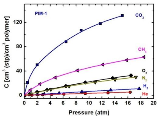
**Fig. S13.** Barometric gas sorption of PIM-1 at 35 °C from pressure ranging from 0 to ~ 18 bar.
