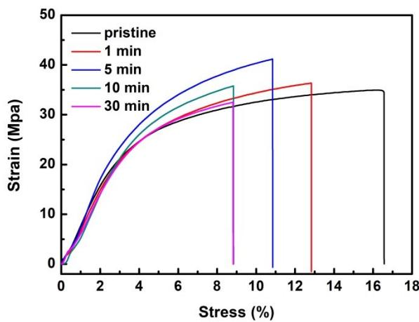
**Fig. S9.** Stress-strain curves of PIM-1 and FPIM membranes at different fluorination times.
