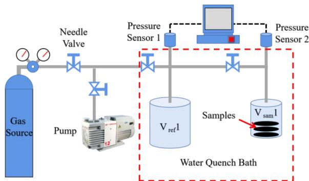
**Fig. S5.** Set up for barometric sorption testing instrument.
