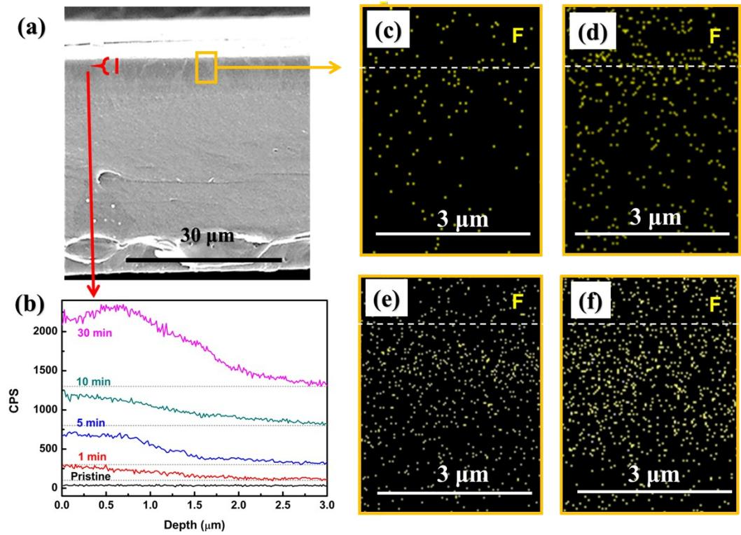
**Fig. S10.** (a) Cross-sectional image of PIM-1. (b) The depth of fluorine signals in cross-sectional EDS mapping of the FPIMs. (c), (d), (e), (f) EDS mapping of the fluorine signals during different fluorination time, (c) 1 min, (d) 5 min, (e) 10 min, (f) 30 min.
