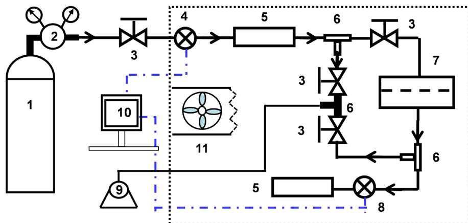
**Fig. S3.** Schematic set-up of pure-gas permeability measurement apparatus; 1: Cylinder, 2: Regulator, 3: Bellows sealed valve, 4: Upstream transducer, 5: Gas cylinder, 6: Welded T-pipe, 7: Membrane cell, 8: Downstream transducer, 9: Pump, 10: Computer, 11: Temperature control.
