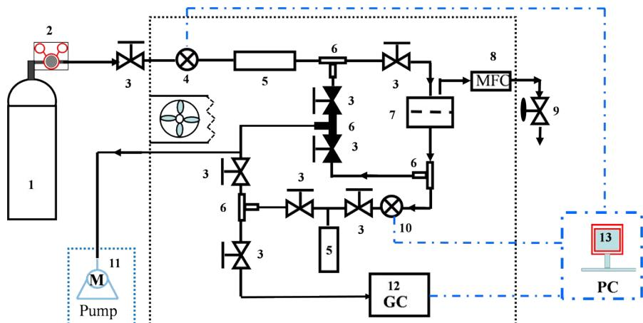
**Fig. S4.** Schematic set-up of mixed-gas properties testing system, 1: Mixed-gas cylinder, 2: Regulator, 3: Bellows sealed valve, 4: Upstream transducer, 5: Gas storage tank, 6: Tee pipeline with welding, 7: Membrane cell, 8: Mass flow meter, 9: Needle valve, 10: Downstream transducer, 11: Vacuum pump, 12: Gas chromatograph, 13: Computer.
