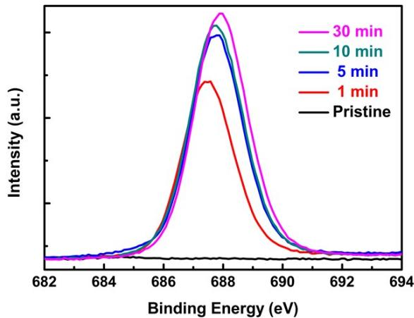
**Fig. S7.**  $\text{F}_{1\text{s}}$  XPS spectra of PIM-1 and FPIMs membranes at different fluorination times.
