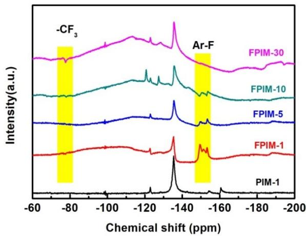
**Fig. S6.** Solid-state  $^{19}\text{F}$ -NMR spectra of the polymer membranes.
