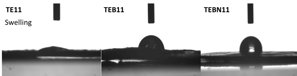
Figure S65: Contact angle images against water of TE11, TEB11 and TEBN11. For swelling polymer TE11, the image is taken several seconds after the drop is deposited onto the polymer surface.
