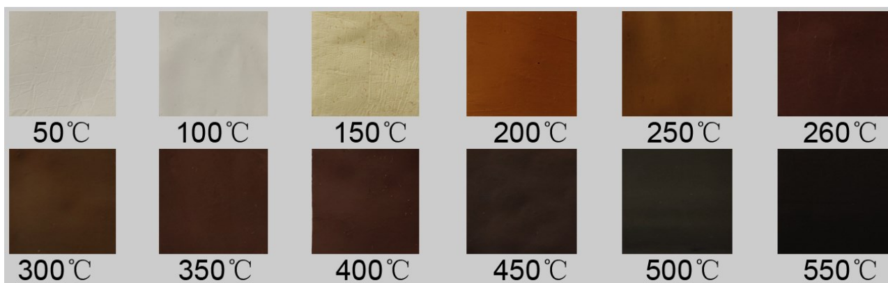
Fig. S3 Digital photos to show the appearance of the fibrous membrane after different treatment steps.
