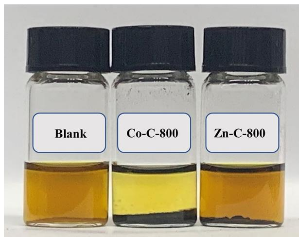
**Fig. S14** Optical image of blank  $\text{Li}_2\text{S}_6$  solution and after adsorbing with Co-C-800 and Zn-C-800, respectively.
