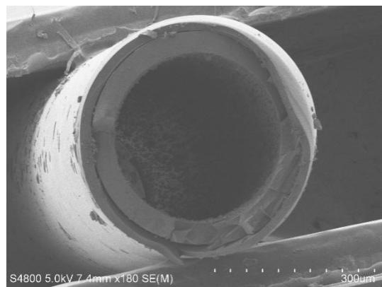
**Fig. S27** The SEM image of the inner wall of (R)-CTzDva coated capillary column.
