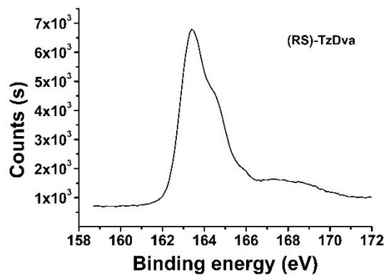
**Fig. S35** S 2p XPS spectra of (RS)-TzDva.
