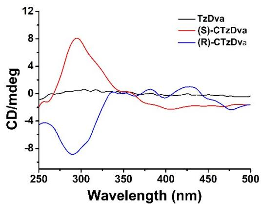
**Fig. S19** Circular dichroism spectra of TzDva and CTzDva.
