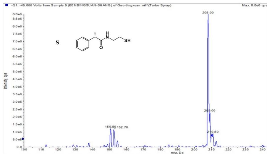
**Fig. S3** Mass spectrum of (S)-*N*-(2-mercaptoproethyl)-2-phenylpropanamide.
