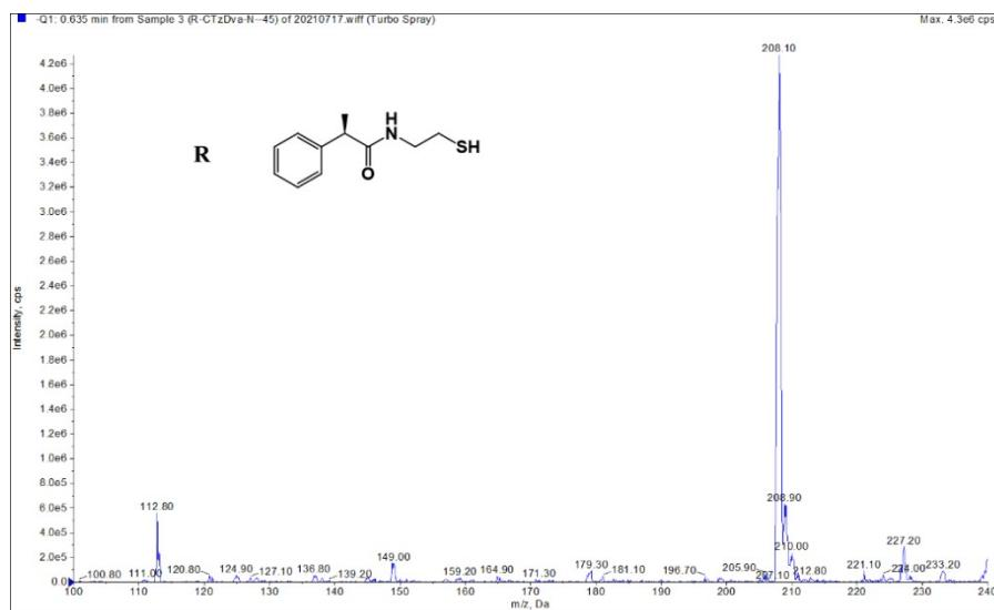
**Fig. S6** Mass spectrum of (R)-N-(2-mercaptoproethyl)-2-phenylpropanamide.
