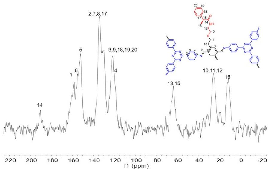
**Fig. S18** Solid  $^{13}\text{C}$  NMR spectrum and peak contribution for CTzDva
