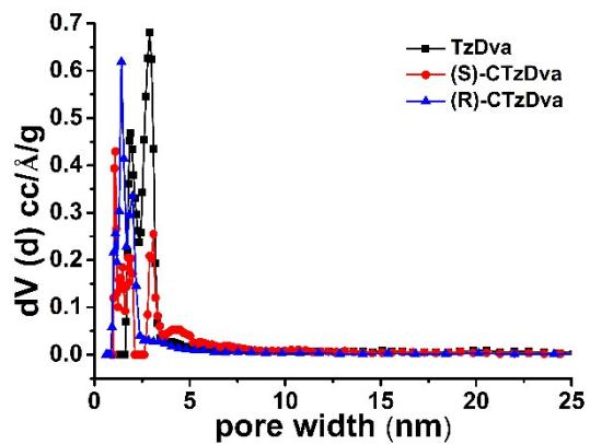
**Fig. S21** Pore size distribution of the as-prepared TzDva and CTzDva.
