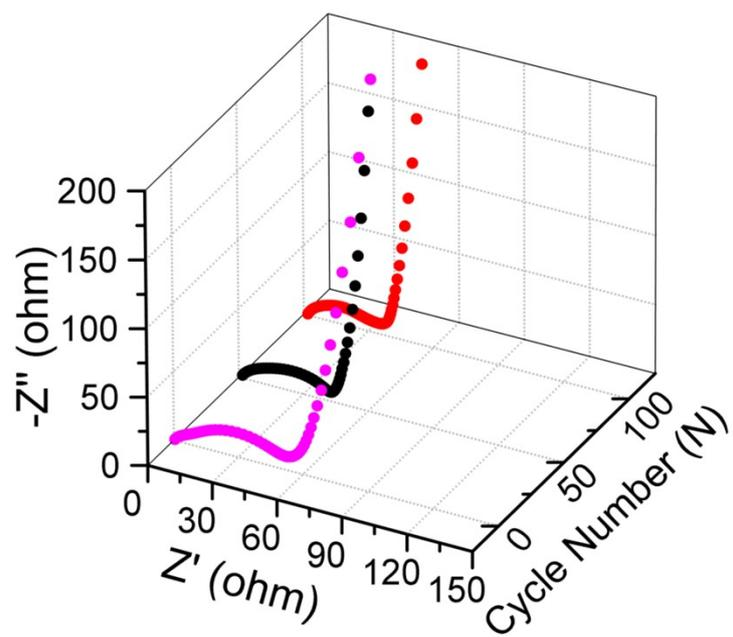
**Fig. S10** Nyquist plots of the impedance spectra of Zn-NC-CNT-Cu symmetric cell before cycling, after 50 cycles and after 100 cycles.
