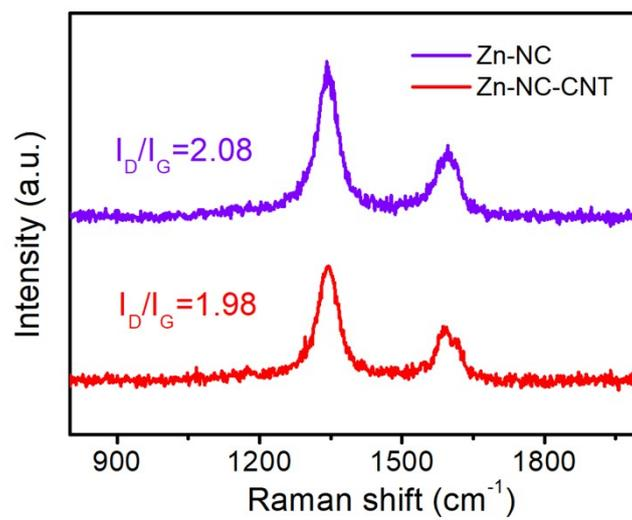
**Fig. S7** Raman spectra of the Zn-NC-CNT and Zn-NC composites.
