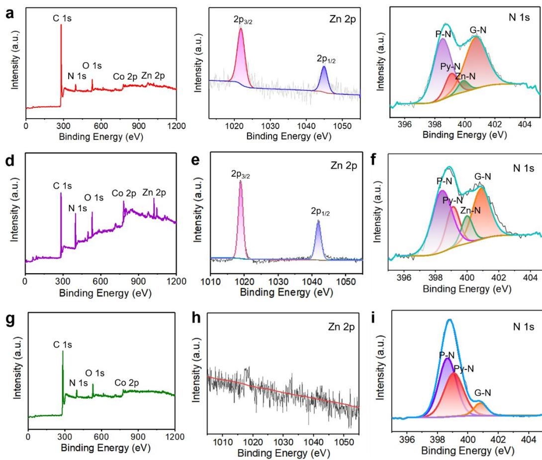
**Fig. S6** (a,b,c) XPS spectra of the Zn-NC-CNT composite. (d,e,f) XPS spectra of the Zn-NC composite. (h,i,j) XPS spectra of the NC-CNT composite. P-N, Py-N, and G-N denote pyridinic N, pyrrolic N, and graphitic N, respectively.
