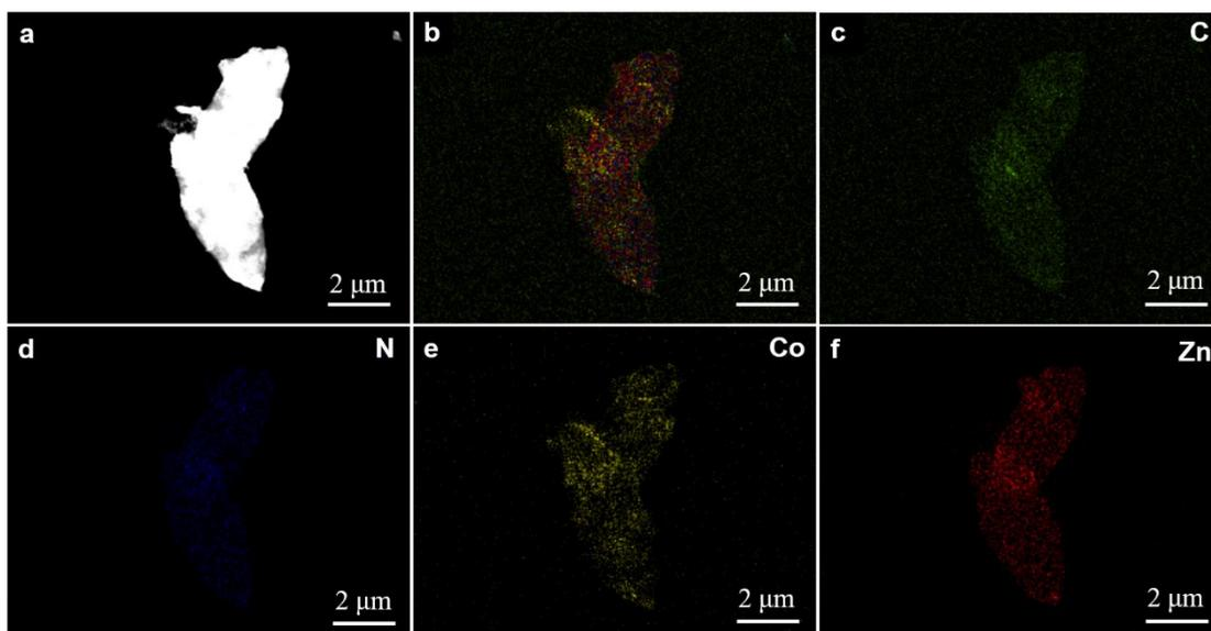
**Fig. S2** SEM image and corresponding EDS elemental maps for the ZIF-L(Zn)@ZIF-L(Co) precursor.
