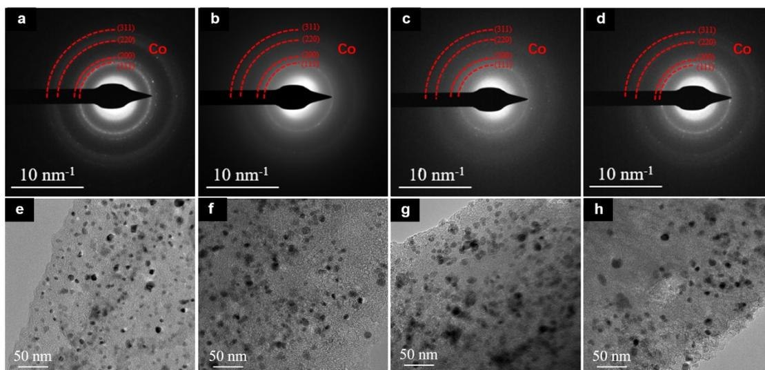
**Fig. S11** (a) SAED and (e) HRTEM images of the Zn-NC-CNT-Cu electrode before cycle. (b) SAED and (f) HRTEM images of the Zn-NC-CNT-Cu electrode after discharge to 0 V. (c) SAED and (g) HRTEM images of the Zn-NC-CNT-Cu electrode after the lithium plating process. (d) SAED and (h) HRTEM images of the Zn-NC-CNT-Cu electrode after the lithium stripping process.
