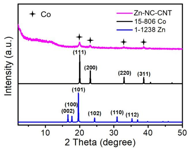
**Fig. S4** XRD pattern of the Zn-NC-CNT composite.
