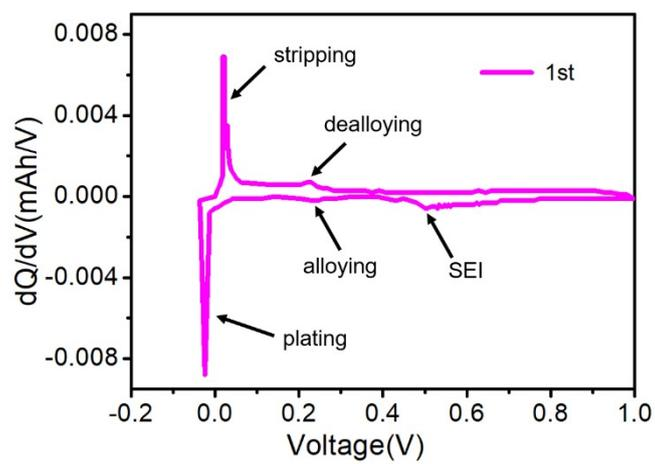
**Fig. S8** The differential capacitance curve of the Zn-NC-CNT-Cu half cell for the first cycle.
