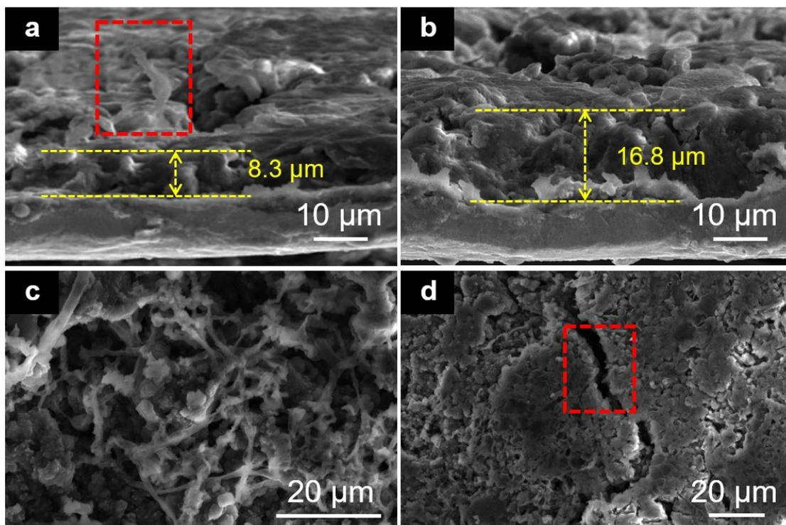
**Fig. S12** (a) Cross section view and (c) top view SEM images of the NC-CNT-Cu electrode after 300 cycles of Li plating/stripping process with a  $1 \text{ mA h cm}^{-2}$  capacity limit. (b) Cross section view and (d) top view SEM images of the Zn-NC-Cu electrode after 300 cycles of Li plating/stripping process with  $1 \text{ mA h cm}^{-2}$  capacity.
