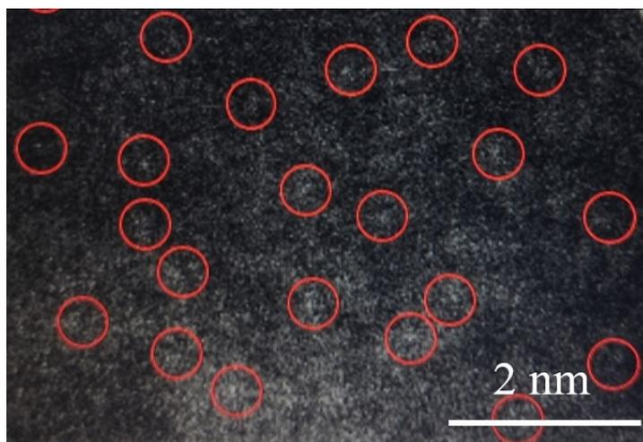
**Fig. S13** Zoom-in HAADF-STEM image of the Zn-NC-CNT-Cu electrode after 300 cycles of Li plating/stripping process, in which the Zn species were highlighted with the red circles.
