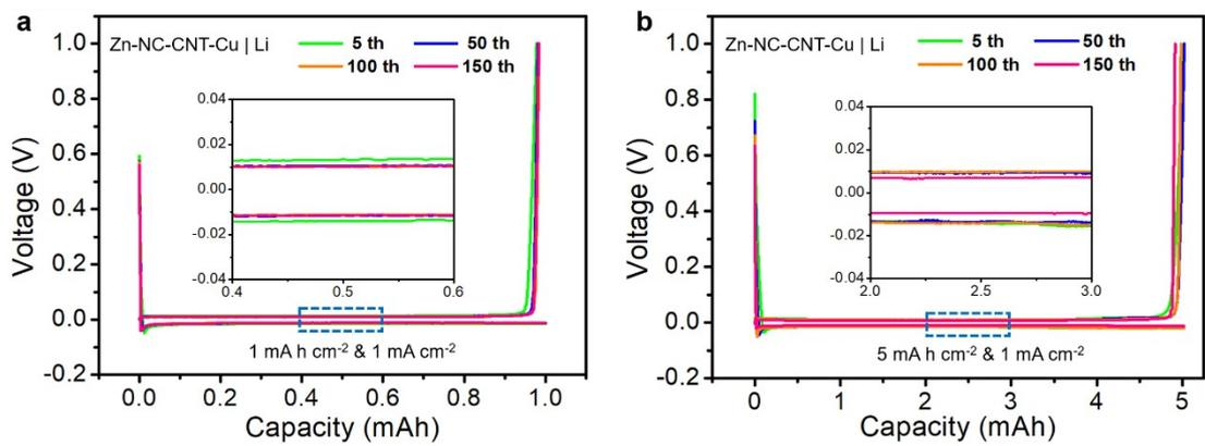
**Fig. S9** Voltage profiles of the different cycles of Zn-NC-CNT-Cu electrode with (a) 1 mA h  $\text{cm}^{-2}$  capacity and (b) 5 mA h  $\text{cm}^{-2}$  capacity.
