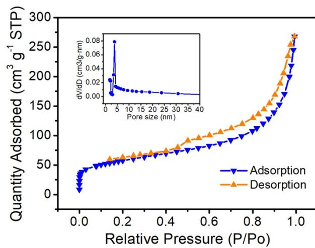
**Fig. S5** Nitrogen adsorption-desorption isotherm and BJH pore size distribution (inset) of the Zn-NC-CNT composite.
