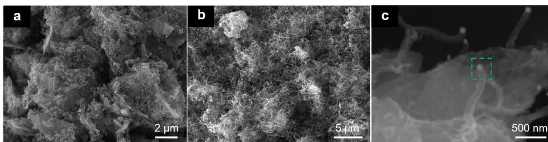
**Fig. S3** SEM images of the Zn-NC-CNT composite at different magnifications. Co was represented in the dotted line in Figure S3c.
