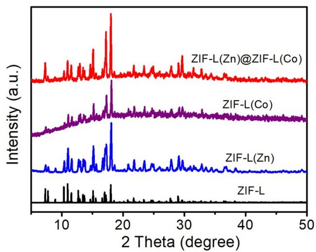
**Fig. S1** XRD pattern of the ZIF-L(Zn)@ZIF-L(Co) precursor.
