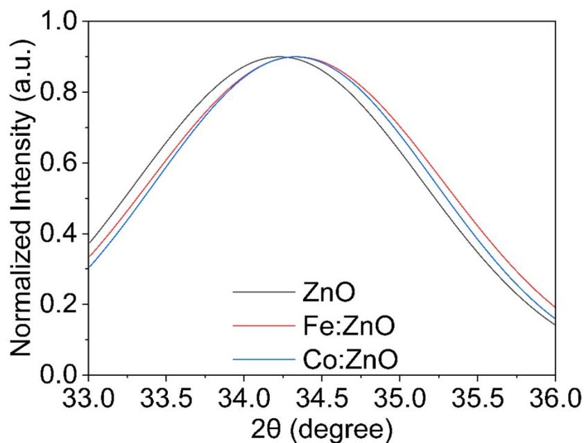
Figure S1. X-ray diffraction of TM:ZnO (TM: Fe, Co) NRs coated by silver NPs in the (002)-indexed plane (corresponding to JCPDS No.36-1451).
