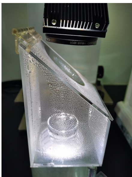
Figure S14. Digital photograph of the simulated seawater desalination device.
