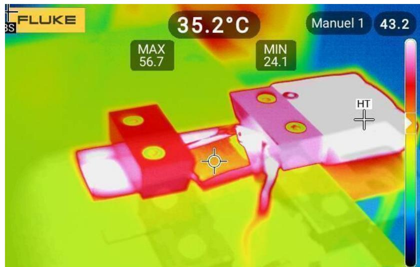
Figure S10. Photograph taken with a thermal camera to measure the surface temperature of the studied film under simulated sunlight (1 sun 1.5AM, Xenon lamp). The central peephole indicates the surface temperature of the perovskite film.
