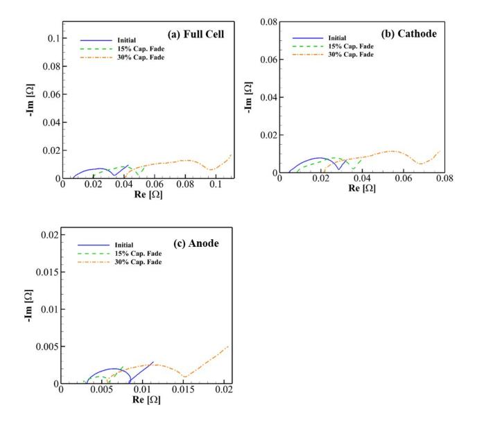
**S2.** EIS spectra of the baseline cell at 0%, 15%, and 30% capacity fade increments for the (a) full cell, (b) cathode, and (c) anode. The cathode semicircle width slightly increases after 30% capacity fade, but the largest increase is apparent in the anode impedance. Lithium plating and passivation layer formation cause the increase of anode impedance.
