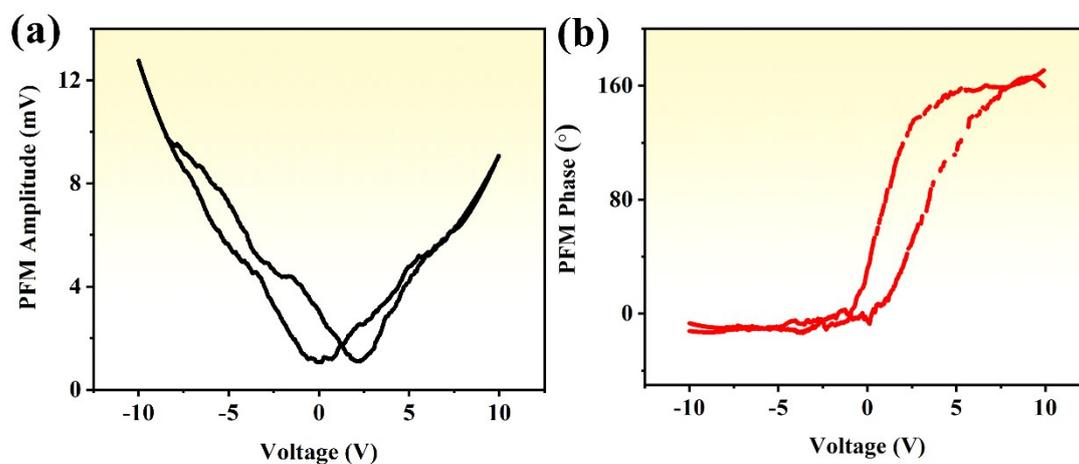
Fig. S1 The piezoresponse force microscopy (PFM) of BNT nanosphere, (a) Amplitude-voltage butterfly loops; (b) phase hysteresis loops.
