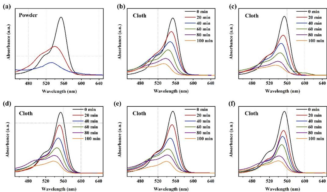
Fig. S7. (a), (b) 0.023 g BNT@3%BVO powder catalyst and cloth-3 were applied to degrade the 50 mL 10 mg/L RhB for comparison; (c)-(f) the same with (b) for the cycle test.
