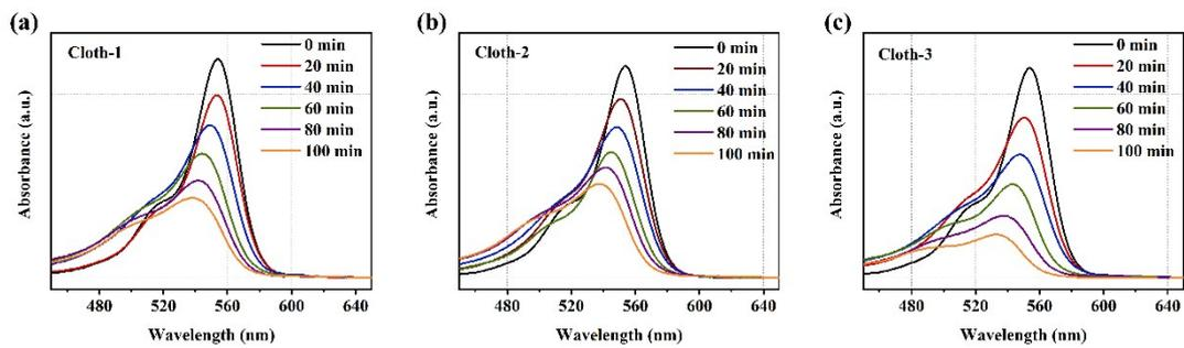
Fig. S6. The degradation of 10 mg/L RhB with (a) cloth-1; (b) cloth-2; (c) cloth-3.
