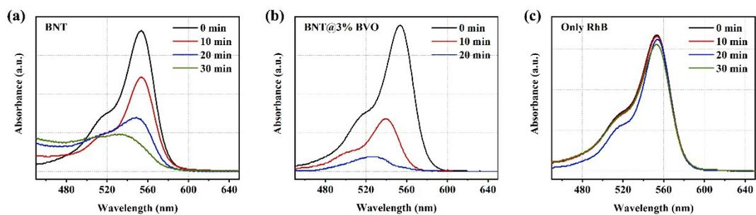
Fig. S3. The Piezo-photocatalytic degradation efficiencies of RhB with concentration of 5 mg/L for (a) pure BNT, (b) BNT@3%BVO and (c) without any calalytics respectively under the simulated sun irradiation together with ultrasonication.
