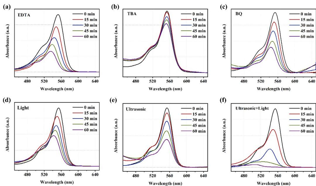
Fig. S8. Time-resolved UV-vis absorption spectra of the RhB solutions ( $C_0 = 10$  mg/L) with (a) EDTA, (b) TBA, (c) BQ as holes ( $h^+$ ),  $\bullet O_2^-$ , and  $\bullet OH$  radicals scavengers, respectively; with (d) light irradiation, (e) ultrasonic vibration, (f) light irradiation and ultrasonic vibration coefficient in the presence of BNT@3%BVO nanospheres.
