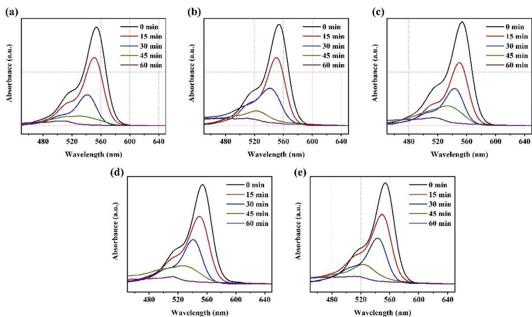
Fig. S5. The five cycle tests of the BNT@3%BVO sample for the piezo-photocatalytic degradation of 10 mg/L RhB.
