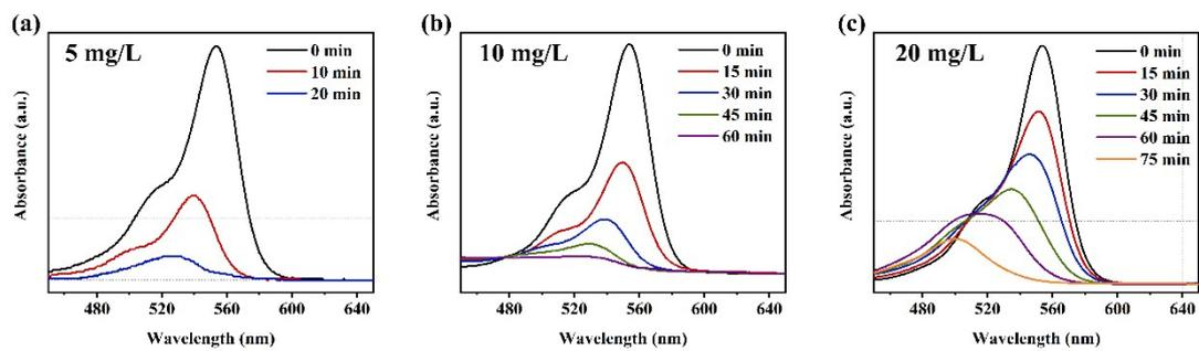
Fig. S4. The degradation efficiencies of RhB with different concentration as (a) 5 mg/L, (b) 10 mg/L and (c) 20 mg/L by using BNT@3%BVO.
