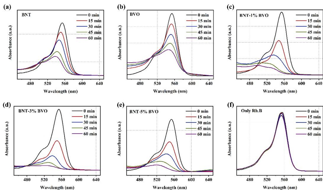
Fig. S2. The Piezo-photocatalytic degradation efficiencies of RhB with concentration of 10 mg/L for (a) pure BNT, (b) BVO, (c) BNT@1%BVO, (d) BNT@3%BVO, (e) BNT@5%BVO and (f) without any calalytics respectively under the simulated sun irradiation together with ultrasonication.
